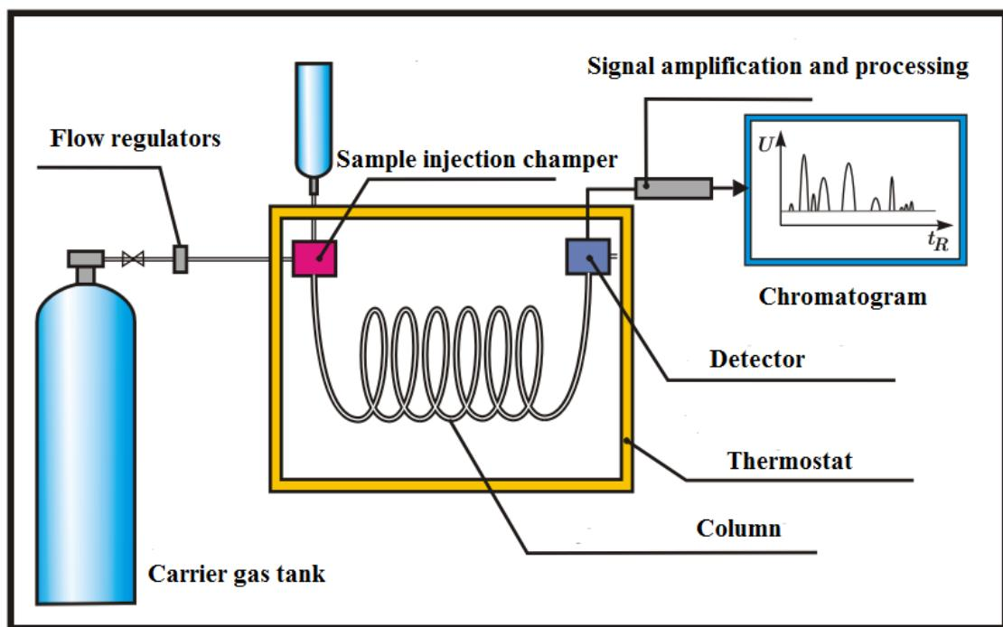
Figure 2.1. Block diagram of a typical gas chromatography[177]
