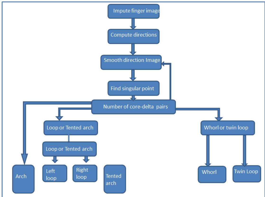
**Figure 2.4. Block diagram of the fingerprint classification algorithm[193]**
