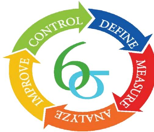
**Figure 4.3:** Six Sigma DMAIC Cycle
