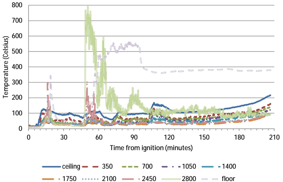
Figure 149 – Temperature data at thermocouple tree B during Reconstruction 1
