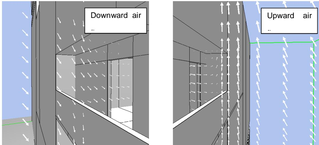
**Figure 107 – JASMINE predictions of flow into flat due to wind<sup>140</sup>**
