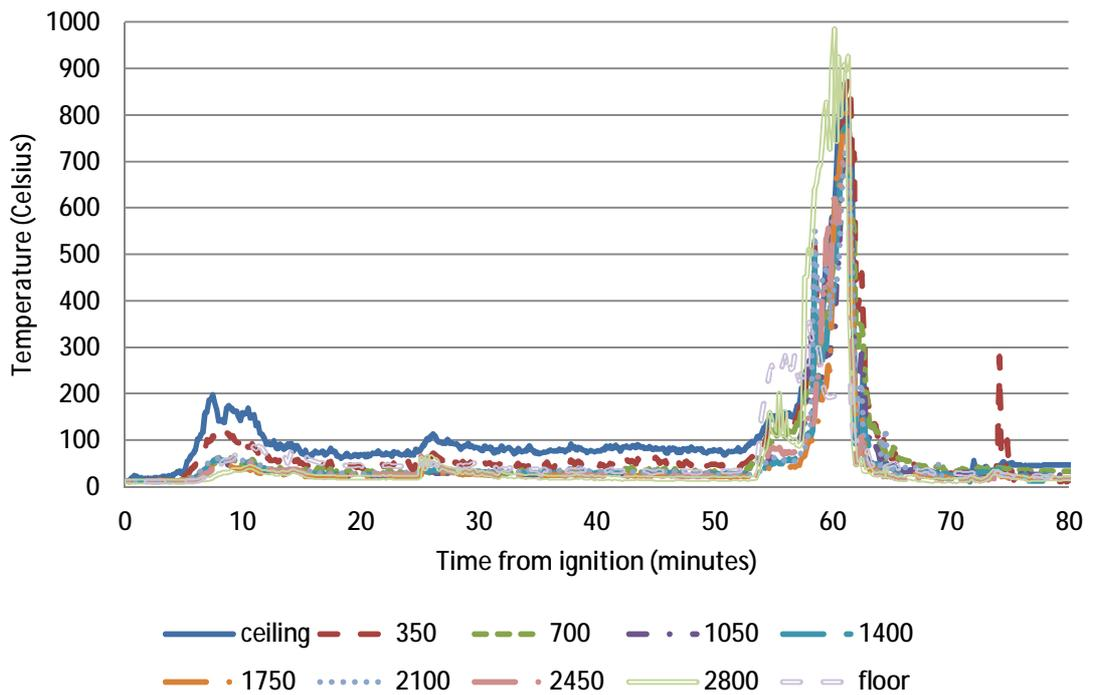
**Figure 157 – Temperature data at thermocouple tree B during Reconstruction 2**
