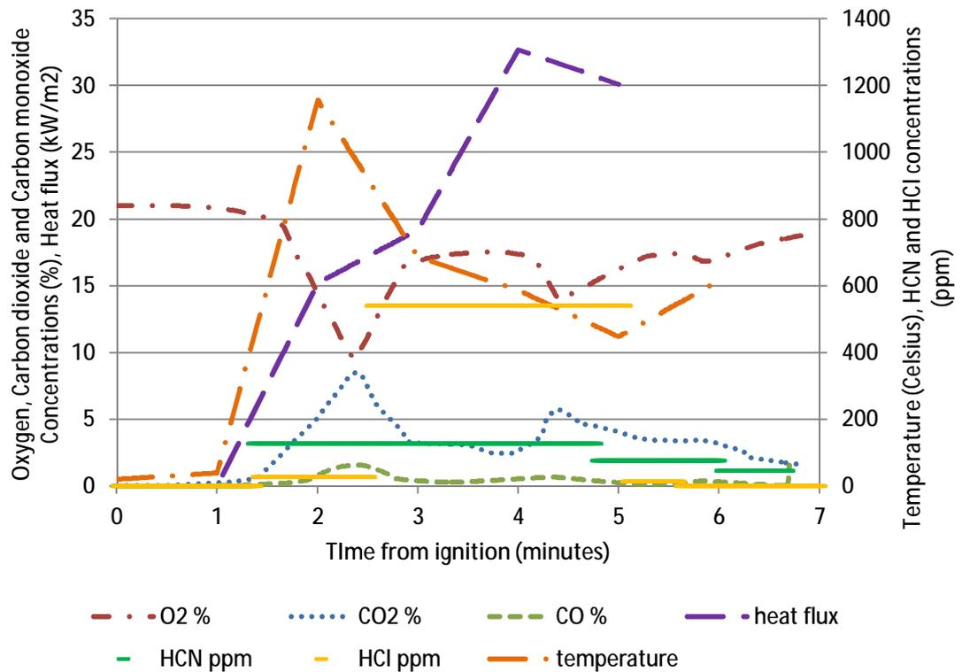
**Figure 15 – Data used from Stardust reconstruction vent point measurements for FED calculations (N.B. HCN and HCl were collected as discrete samples to provide average concentration over set periods, so data is presented as discrete periods)**
