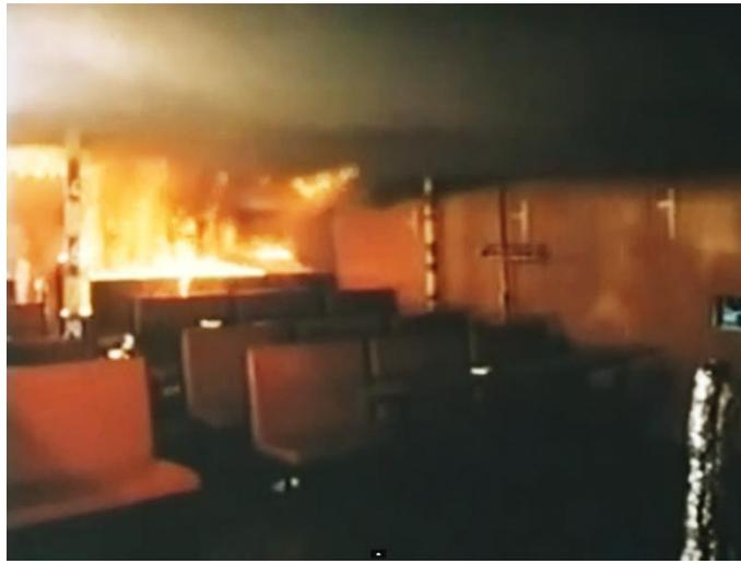
**Figure 8 – Still from BRE/FRS video of Stardust reconstruction (see Appendix A), fire initially developed on seating and involving nearby carpet tiles lining walls**
