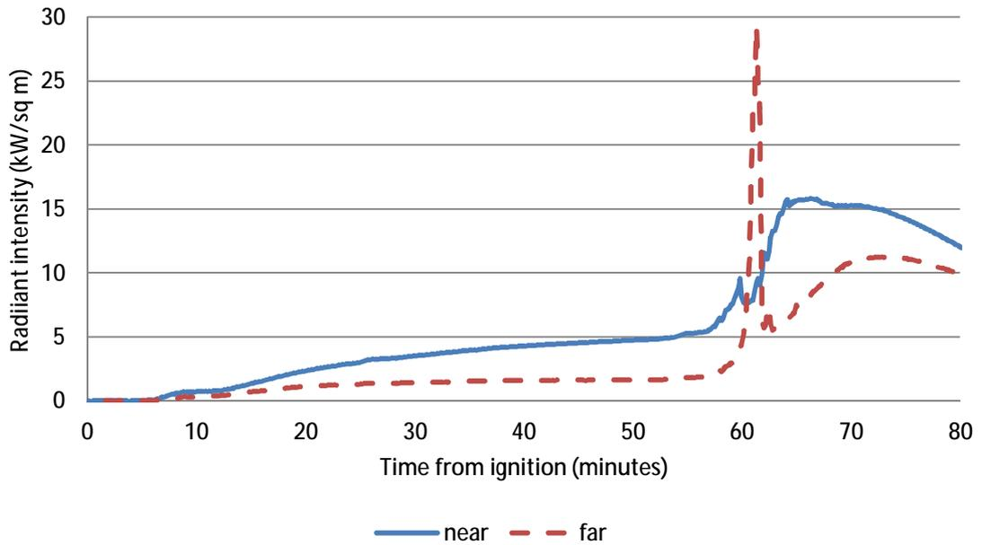
**Figure 162 – Radiant heat fluxes measured at floor level inside the corridor 2m (near) and 4m (far) away from the front edge of the room during Reconstruction 2**
