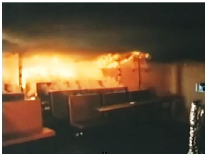
**Figure 9 – Still from BRE/FRS video of Stardust reconstruction (see Appendix A), downward radiation causing pyrolysis of seat covering**
