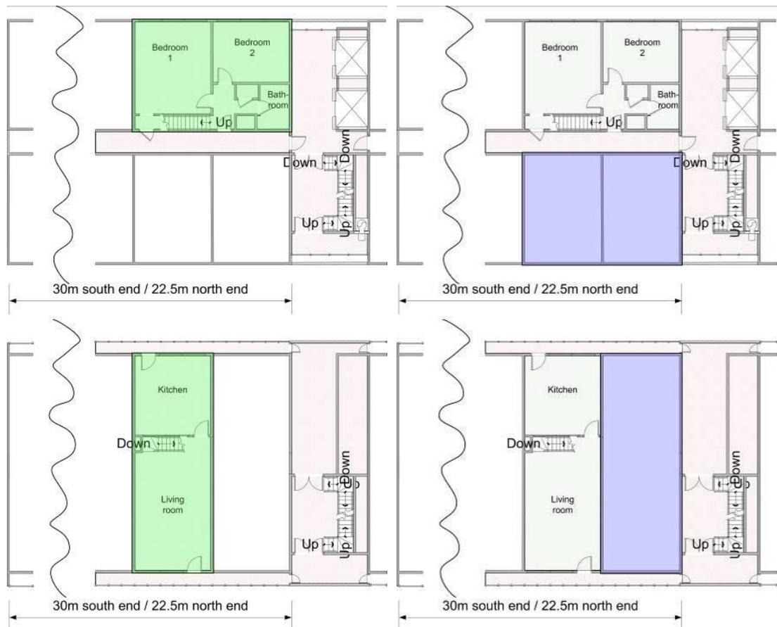
Figure 49 – Plan view diagram showing interlocking of flats and corridor<sup>140</sup>
