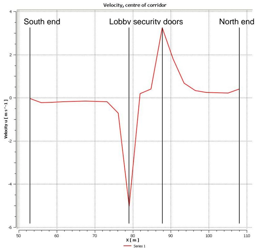
**Figure 106 – Predictions of airflow along the 11<sup>th</sup> floor corridor produced by CFX software<sup>140</sup>**
