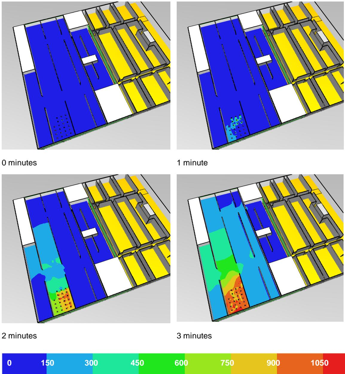
**Figure 172 – Contours of temperature predictions for Scenario 4; horizontal section at head height in Section B and lift lobby**
