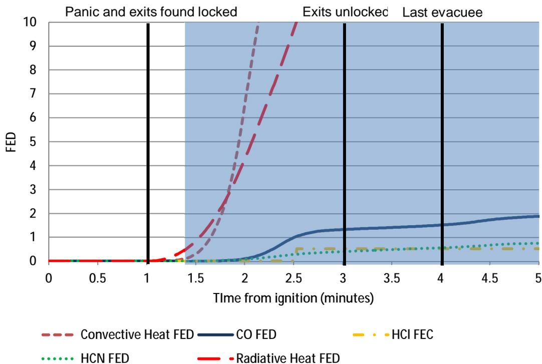
**Figure 181 – FED values based upon Stardust reconstruction vent point measurements. Markers have been added to show relevant events. The shaded area indicates where under-ventilated conditions are predicted by CO:CO<sub>2</sub> ratio exceeding 0.1 on Figure 180**
