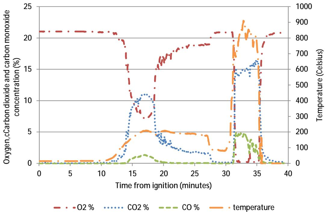
**Figure 47 – Data used from Harrow Court reconstruction data lying down measurements for FED calculations**
