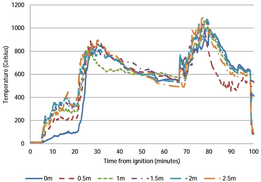
Figure 78 – Temperature data at thermocouple tree D<sup>140</sup>
