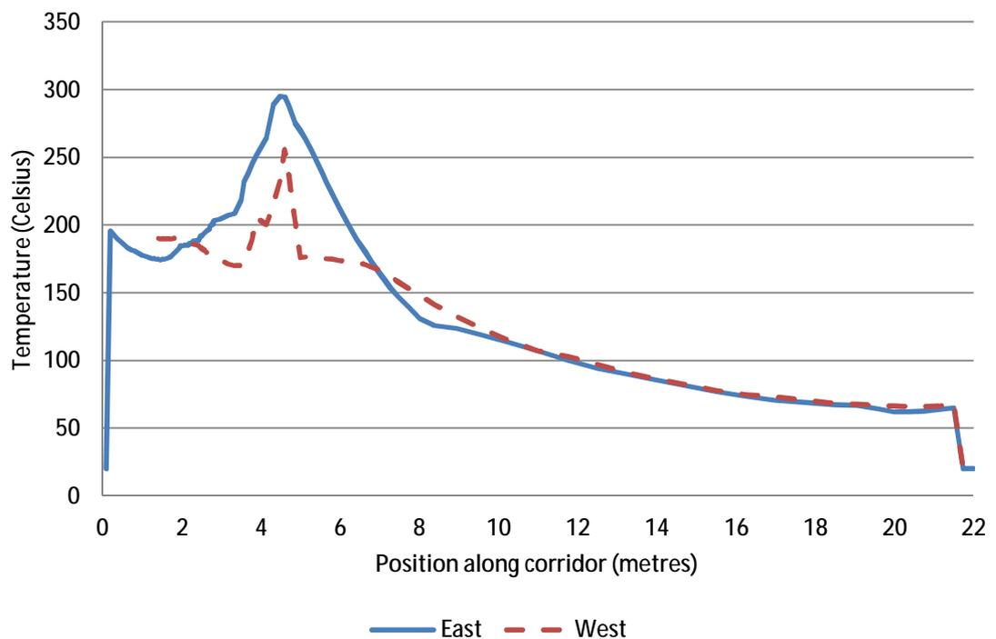
**Figure 128 – Temperature above the false ceiling<sup>140</sup>**
