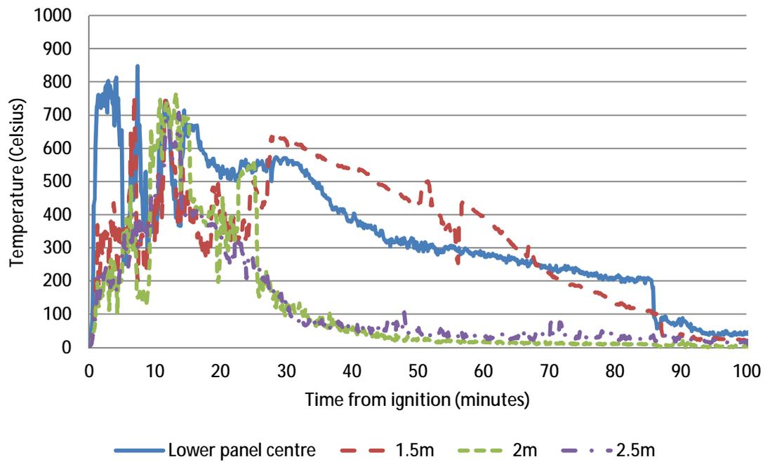
Figure 85 – Temperature data at thermocouple positions on window B<sup>140</sup>
