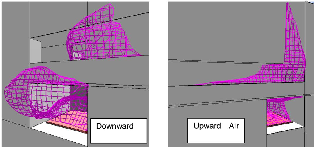
**Figure 108 – JASMINE predictions of flow into flat due to wind and a 6MW fire in bedroom 1<sup>140</sup>**
