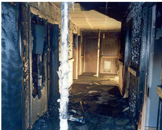
**Figure 30 – View of corridor in Rosepark reconstruction rig corresponding with Figure 29, but after the fire**
