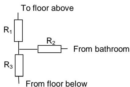
**Figure 133 – Duct damper network<sup>140</sup>**
