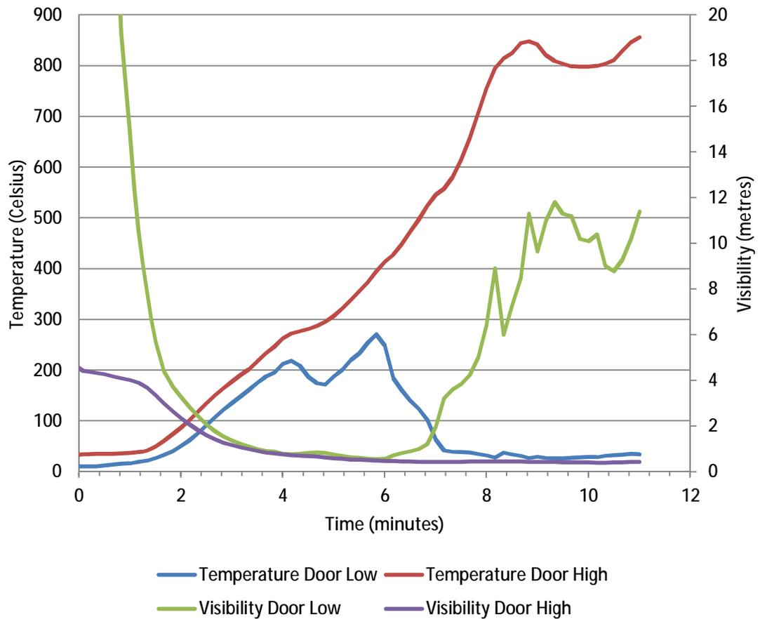
**Figure 177 – Temperature and visibility at opening in four hour wall for Scenario 4**
