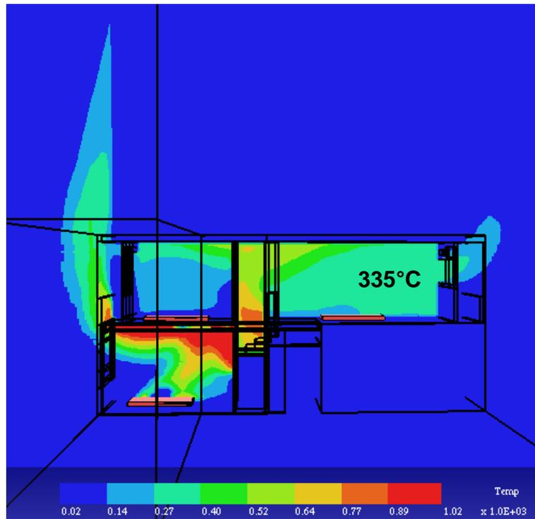
Figure 115 – Flat 65 JASMINE simulation 640 seconds<sup>140</sup>
