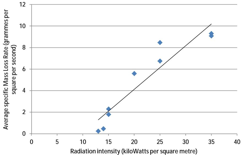
**Figure 165 – Average mass loss rate plot from cone calorimeter tests on particle board flooring**
