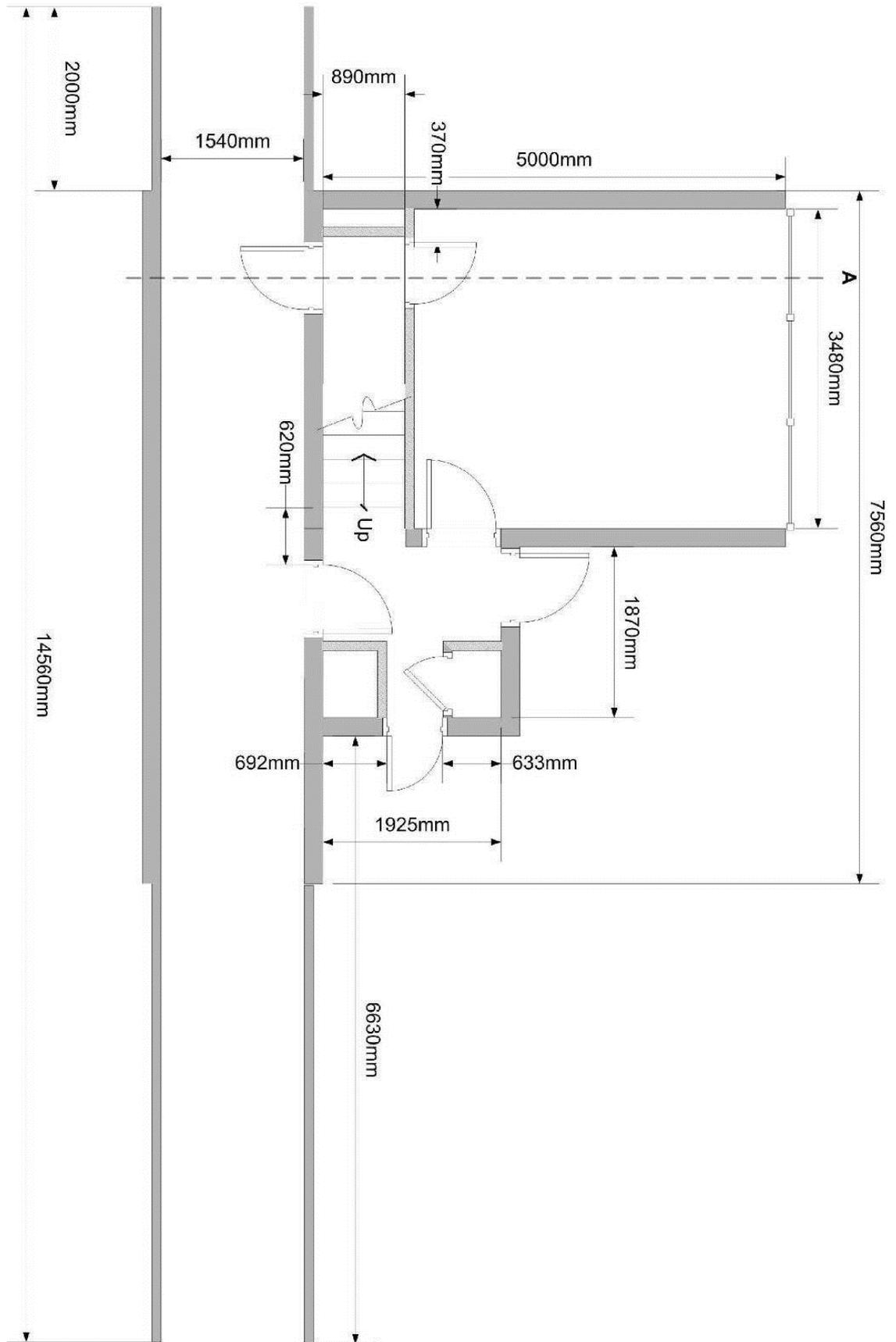
Figure 61 – Ground floor plan of the reconstruction rig<sup>140</sup>
