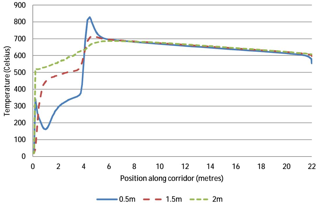
Figure 123 – JASMINE simulation of corridor and ceiling void<sup>140</sup>
