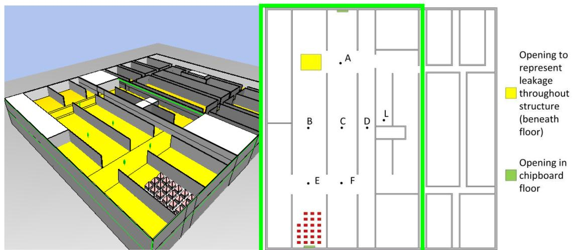
**Figure 168 – Geometric model of first floor storage area. The green box indicates the extent of the calculation domain**
