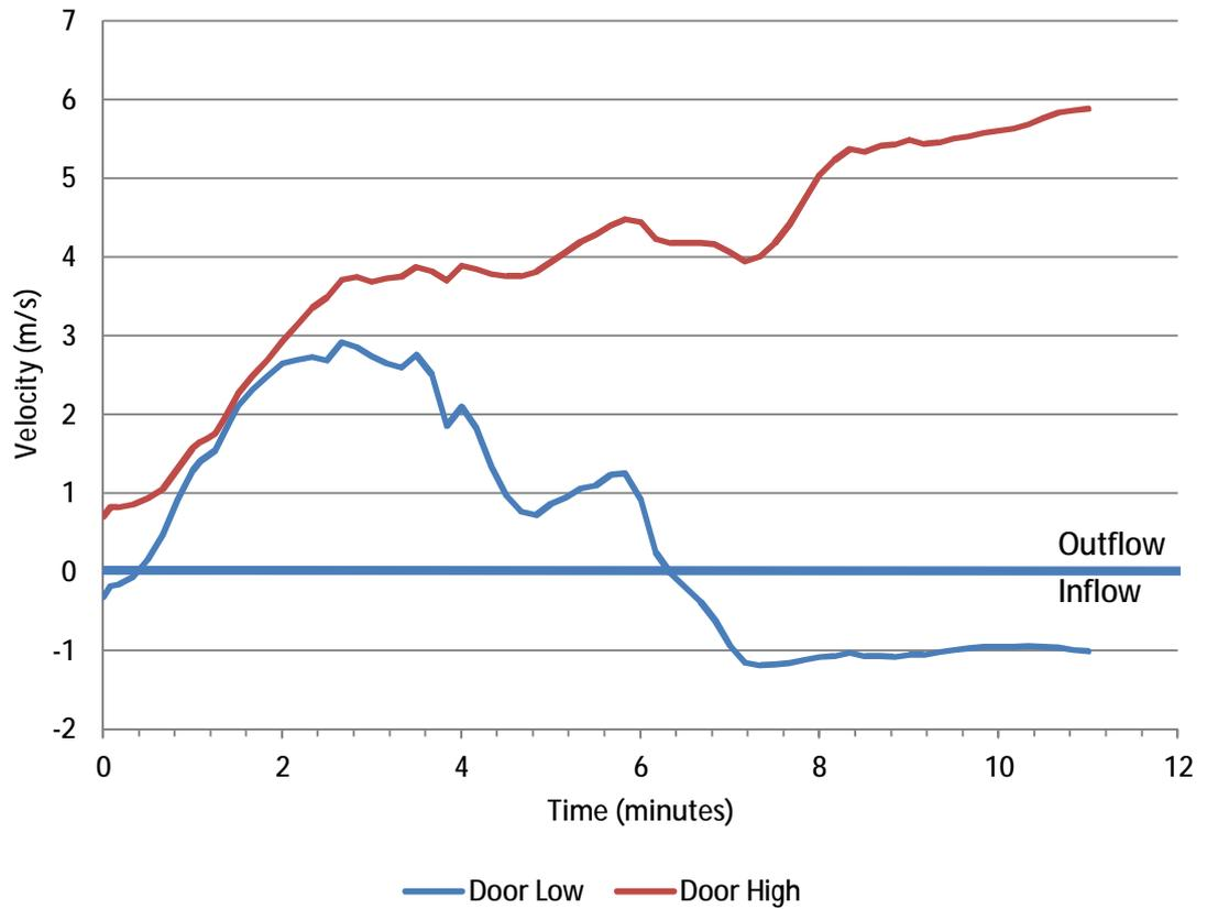
**Figure 175 – Velocity at first floor storage area door for Scenario 4**
