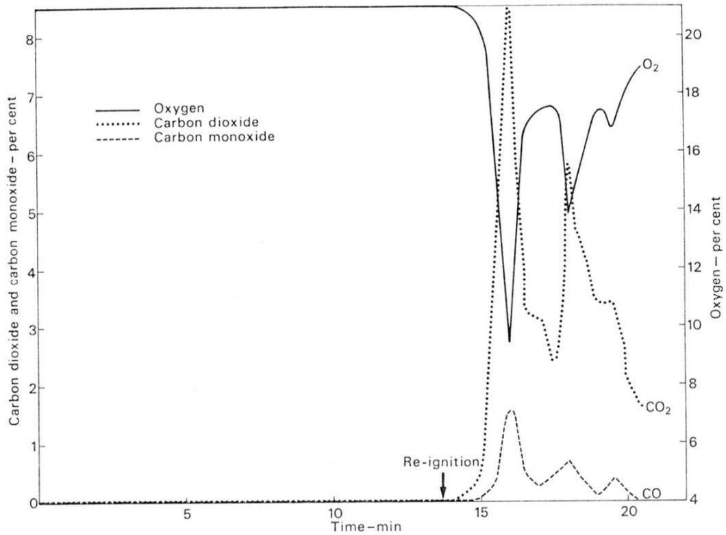
Figure K9 Permanent gas analysis (vent point)
