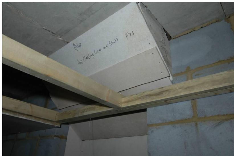
Figure 68 – Mineral fibre box assembly beneath the stairs in the reconstruction rig<sup>140</sup>
