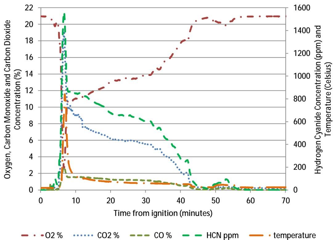
Figure 32 – Gas concentrations measured in Rosepark corridor 4B (fire corridor)
