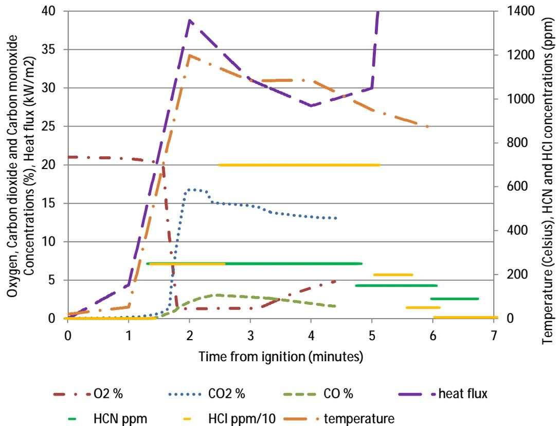
**Figure 14 – Data used from Stardust reconstruction annex point measurements for FED calculations (N.B. HCN and HCl were collected as discrete samples to provide average concentration over set periods, so data is presented as discrete periods)**
