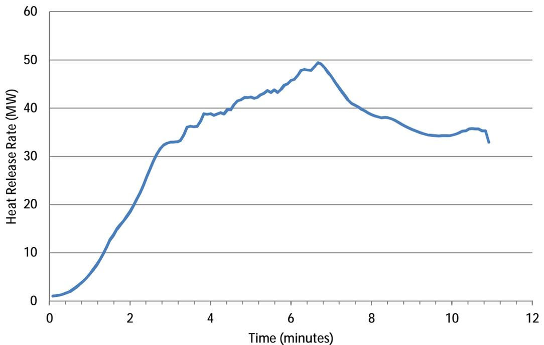
**Figure 174 – Total heat release rate for Scenario 4**
