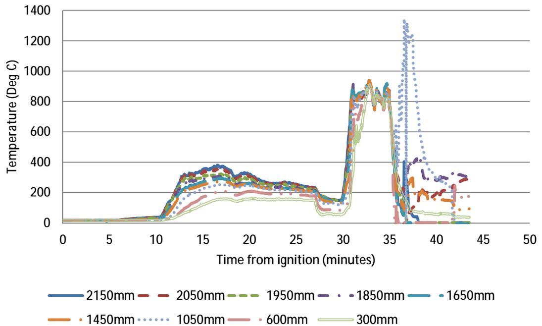
**Figure 43 – Temperatures measured in reconstruction fire in Harrow Court bedroom at heights from floor. N.B. The erratic peaks after 35 minutes are due to fire fighting activity<sup>138</sup>**
