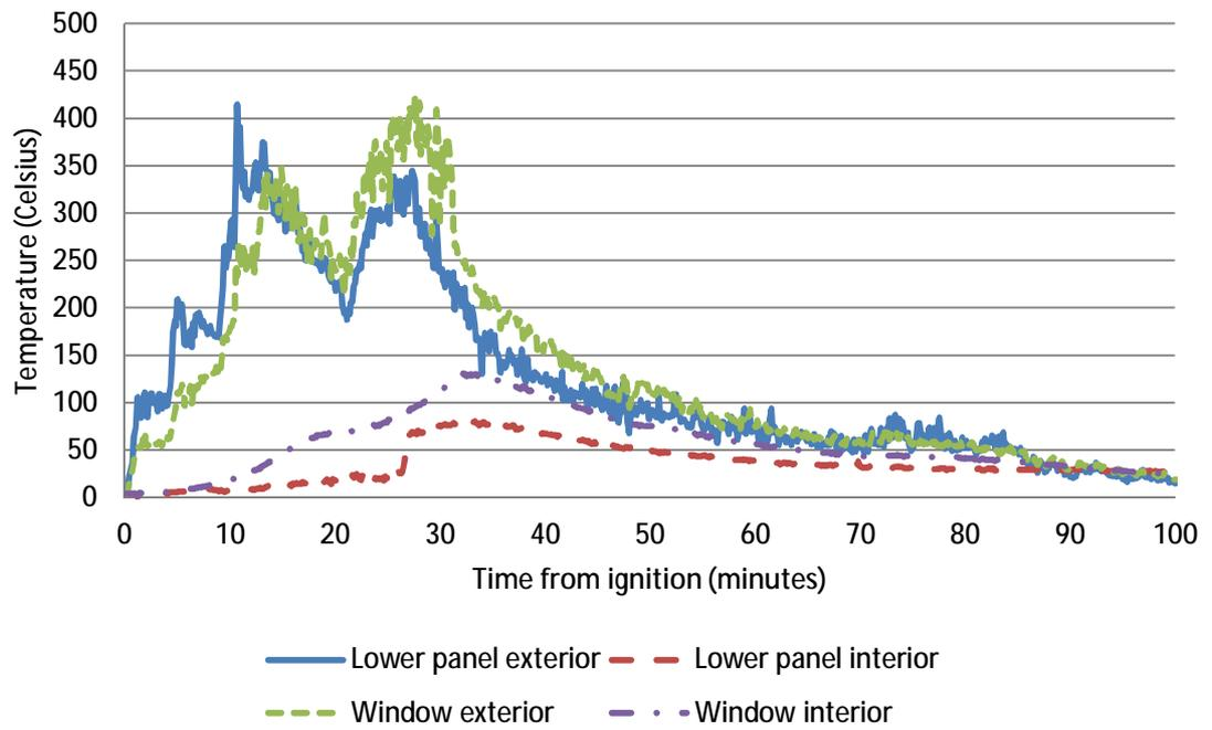
Figure 88 – Temperature data at thermocouple positions on window D <sup>140</sup>
