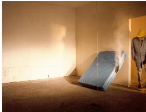
**Figure 21 – Plate number 1 from the FRS report into the Maysfield fire<sup>131</sup> (see Appendix A) showing the smouldering test on the crash mat 20 minutes after ignition**
