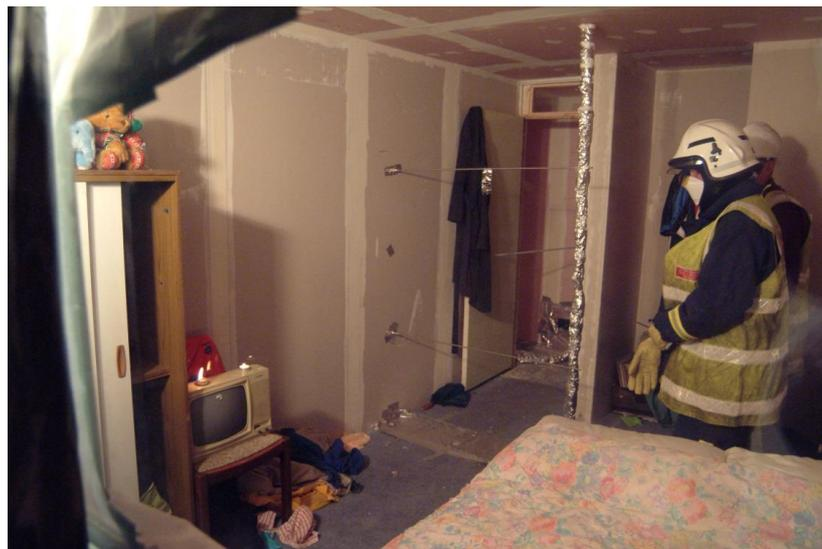
**Figure 40 – View of start of reconstruction fire (ignition recreates candle “tea-lights” left on top of television set by occupants). Thermocouple column and gas sampling lines can**
