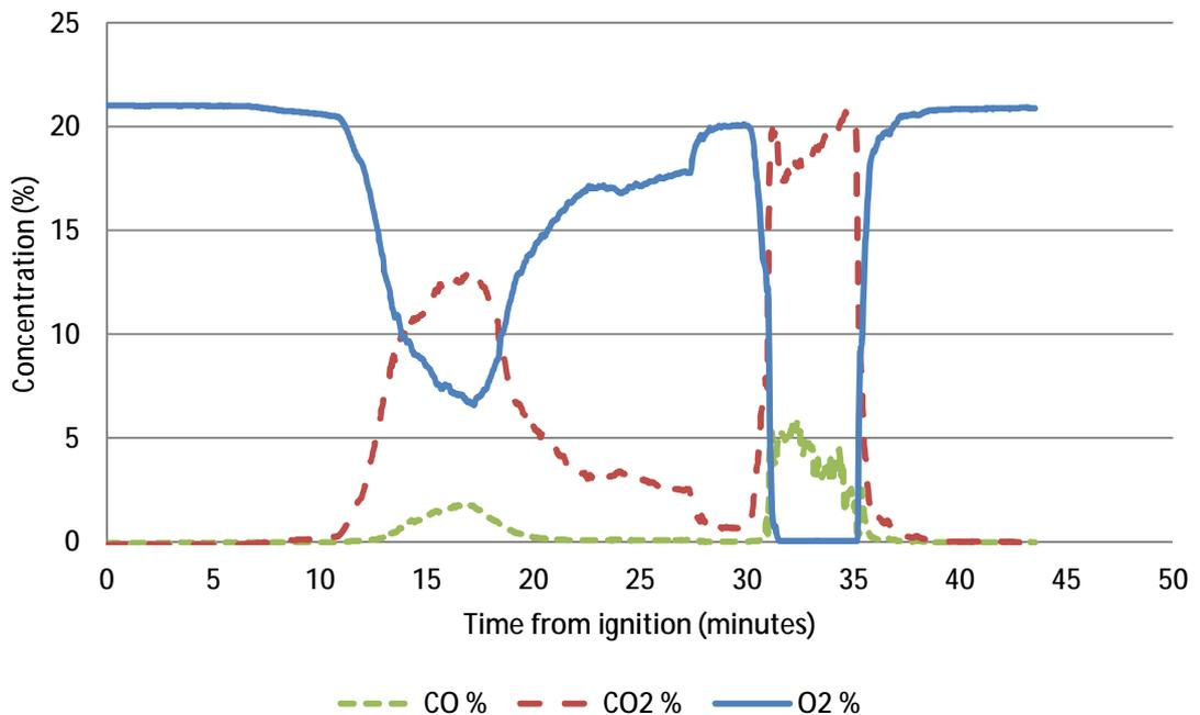
**Figure 42 – Gas concentrations measured in reconstruction fire in Harrow Court bedroom, nose height of standing person<sup>138</sup>**
