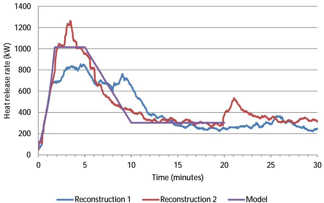
**Figure 167 – Comparison of the heat release rates with aligned ignition times for the reconstruction fires and the “model”**
