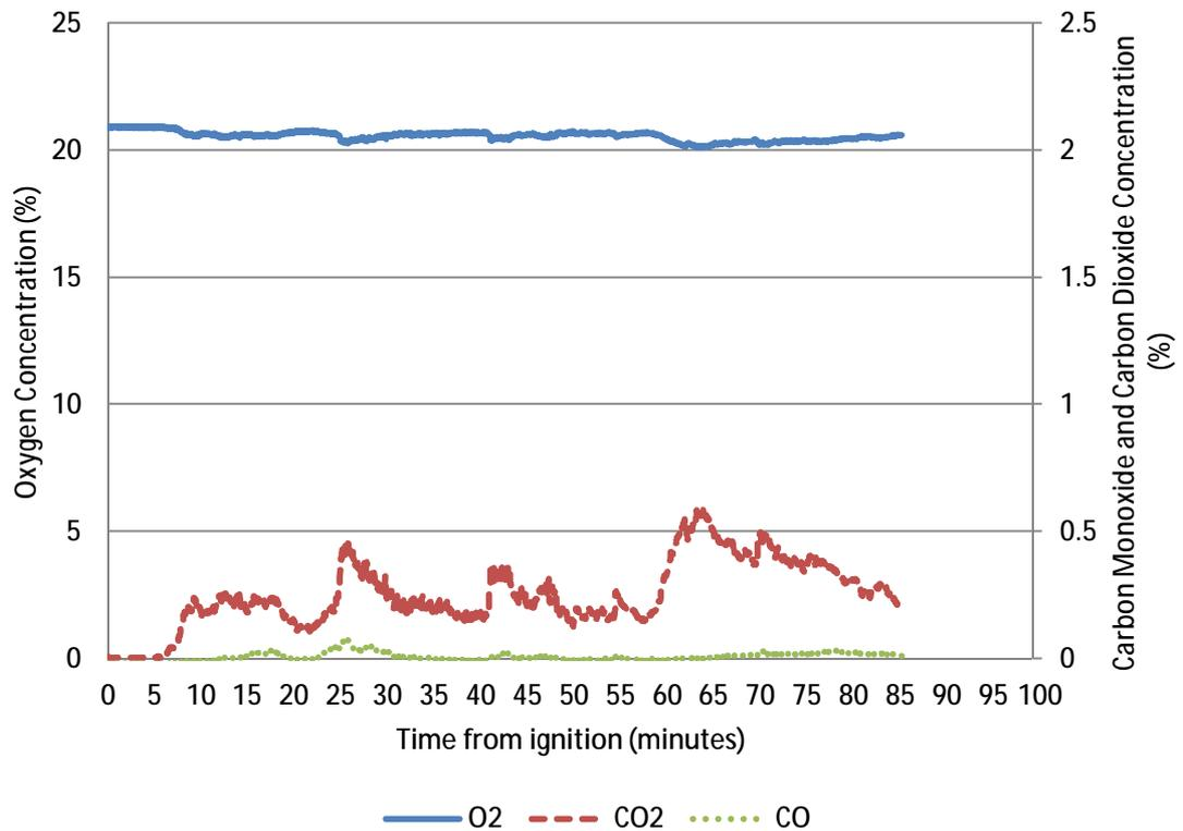
**Figure 102 – Gas concentrations measured by corridor calorimeter (collecting gases from end of corridor)<sup>143</sup>**
