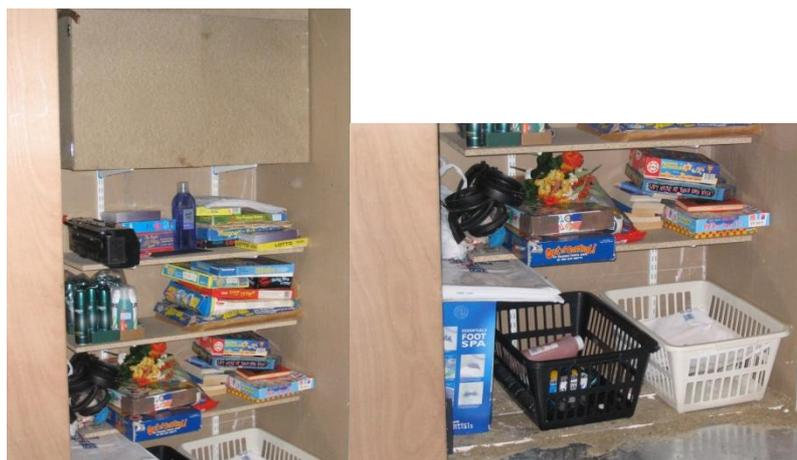
**Figure 27 – Contents of cupboard used for Rosepark reconstruction fires, understood to represent actual contents of cupboard at time of fire. The distribution board (ignition source for the fire) is located in the brown box in the top of the left hand image**
