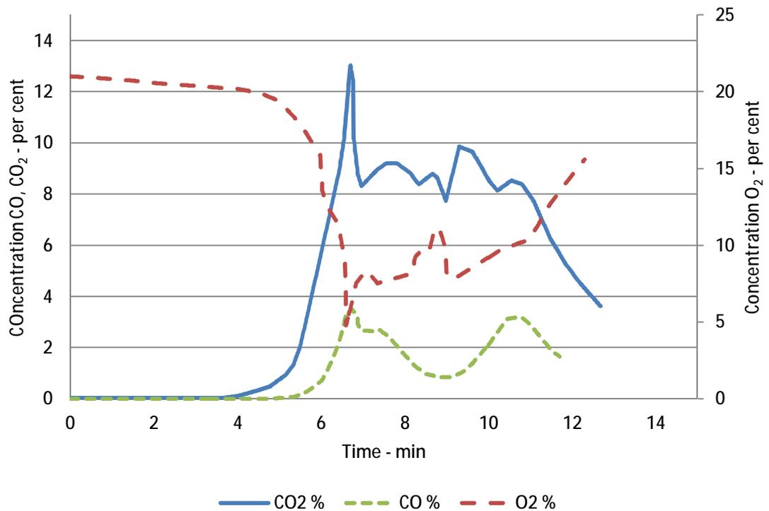
**Figure 25 – Excel plot of data manually “recovered” from Figure 24 (N.B. Only data for 300mm below the ceiling has been used)**
