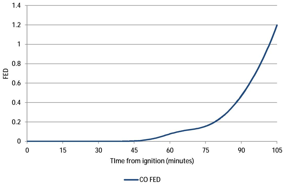
**Figure 139 – FED values calculated using ISO 13571 method based upon reconstruction, modelling data and engineering calculations for the bathroom of Flat 81**
