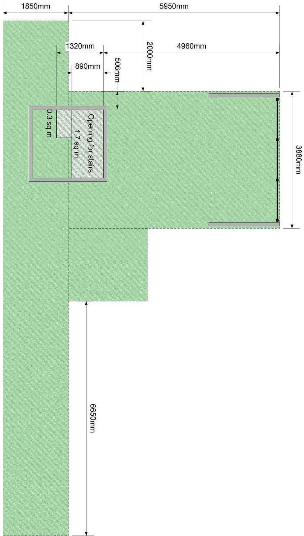
Figure 62 – Upper floor plan of the reconstruction rig<sup>140</sup>
