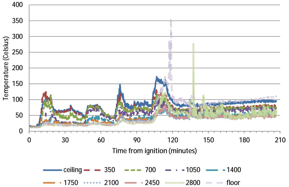
Figure 148 – Temperature data at thermocouple tree A during Reconstruction 1
