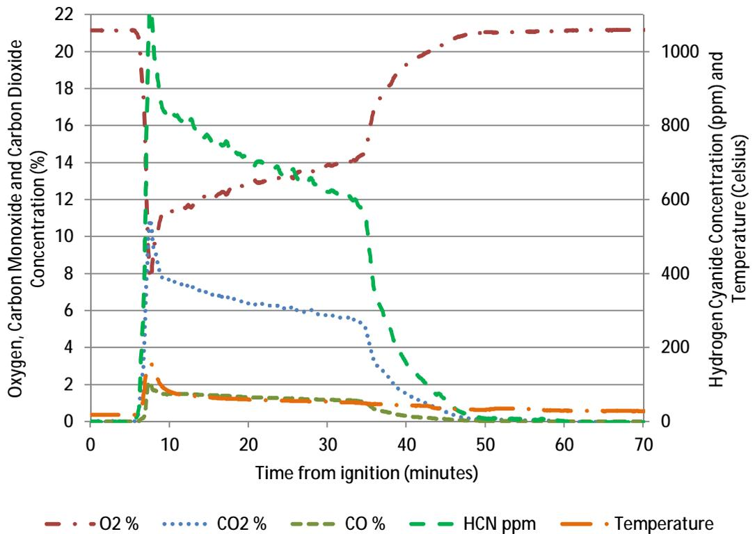
**Figure 34 – Gas concentrations measured in Rosepark open room condition**
