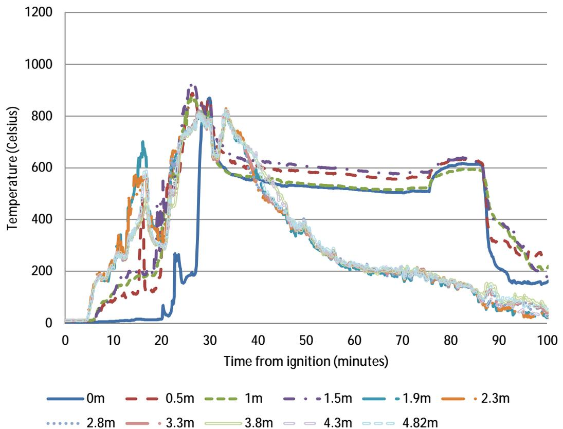
**Figure 77 – Temperature data at thermocouple tree C<sup>140</sup>**
