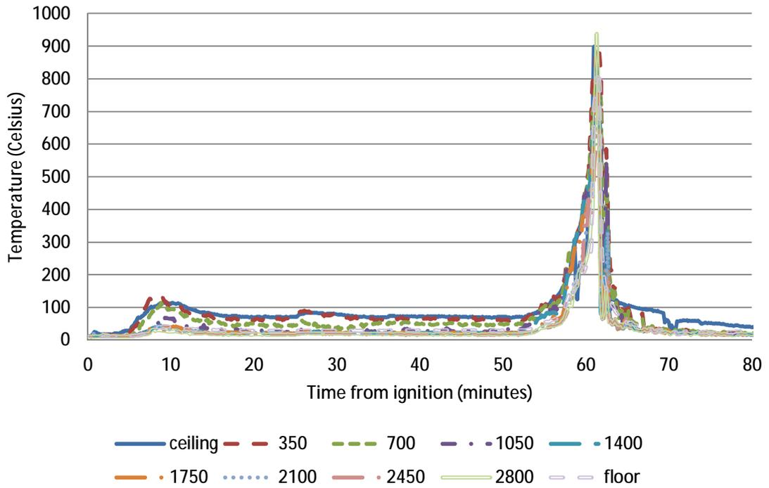
**Figure 156 – Temperature data at thermocouple tree A during Reconstruction 2**
