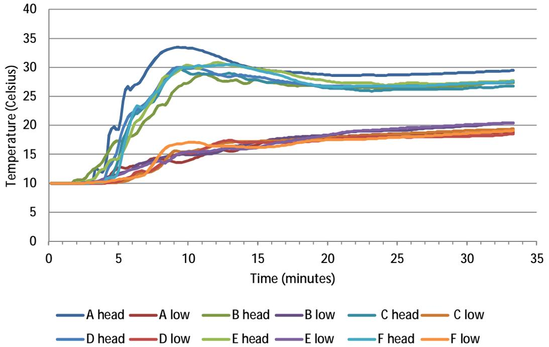
**Figure 169 – Predictions of temperature in first floor storage area at the locations shown on Figure 168**
