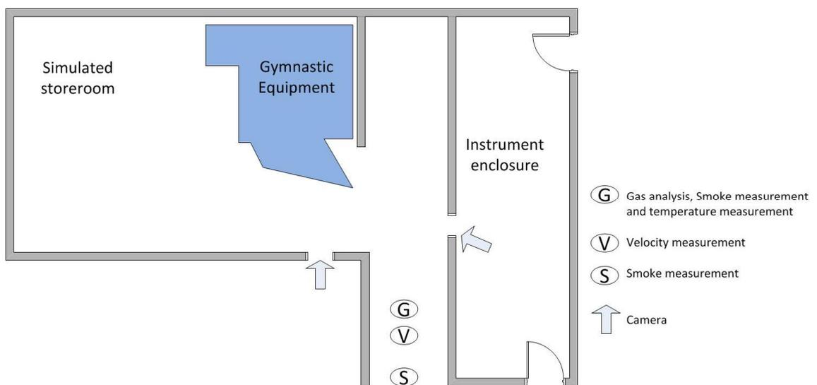
**Figure 20 – Figure 2 from the FRS report into the Maysfield fire<sup>131</sup>, showing the layout of the reconstruction rig used to simulate the fire. Note that the rig was designed to be mirror image of the actual layout in the incident**
