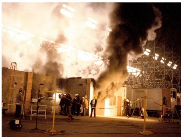
**Figure 23 – Plate number 12 from the FRS report into the Maysfield fire<sup>131</sup> (see Appendix A) showing the amount of smoke issuing from the full-scale flaming test 7 minutes after ignition**
