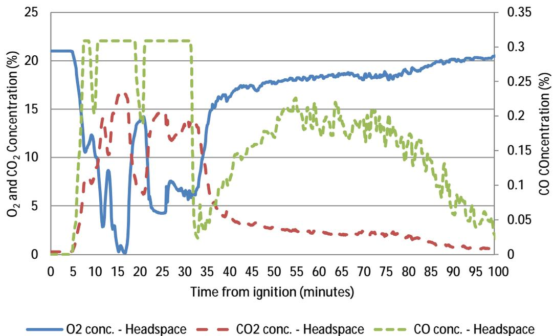
**Figure 103 –Gas concentration data for gases sampled at low level in the 1<sup>st</sup> floor headspace above the stairs<sup>140</sup>**
