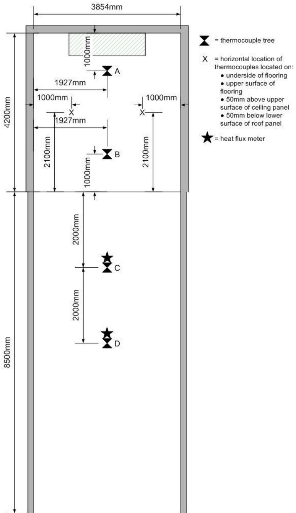
Figure 147 – Plan view of reconstruction rig showing the instrumentation locations
