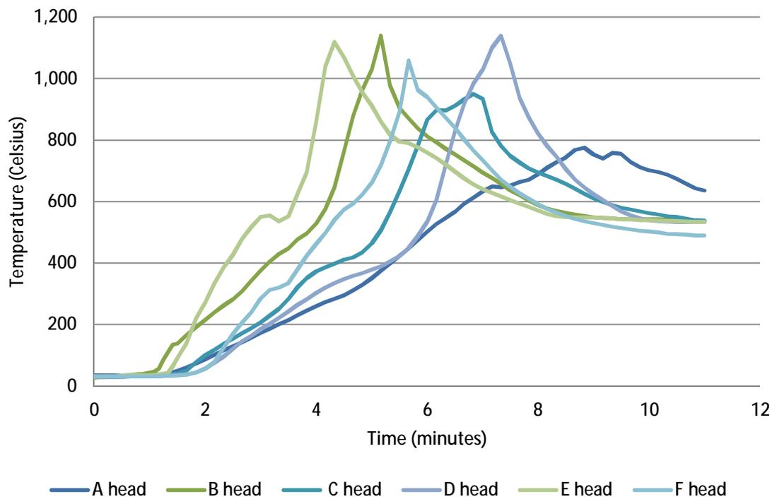
**Figure 171 – Temperature predictions for Scenario 4 at head height at the locations shown on Figure 168. Note that time zero does not relate to the first ignition during the incident, but to the ignition of the secondary pallets**
