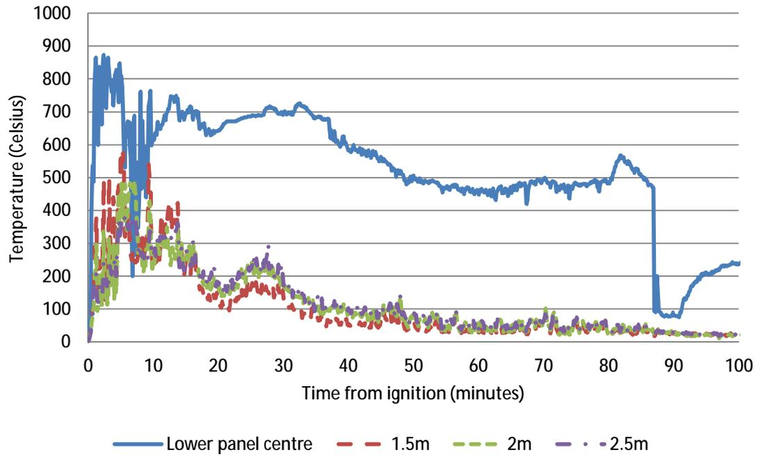
Figure 84 – Temperature data at thermocouple positions on window A<sup>140</sup>
