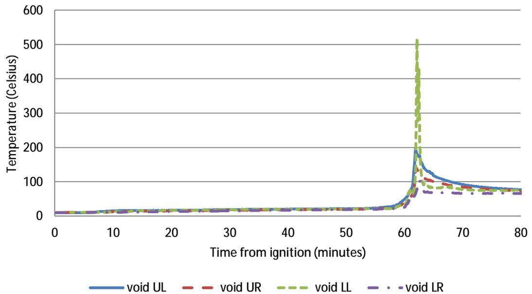
**Figure 160 – Temperature data at thermocouples located in ceiling void during Reconstruction 2**
