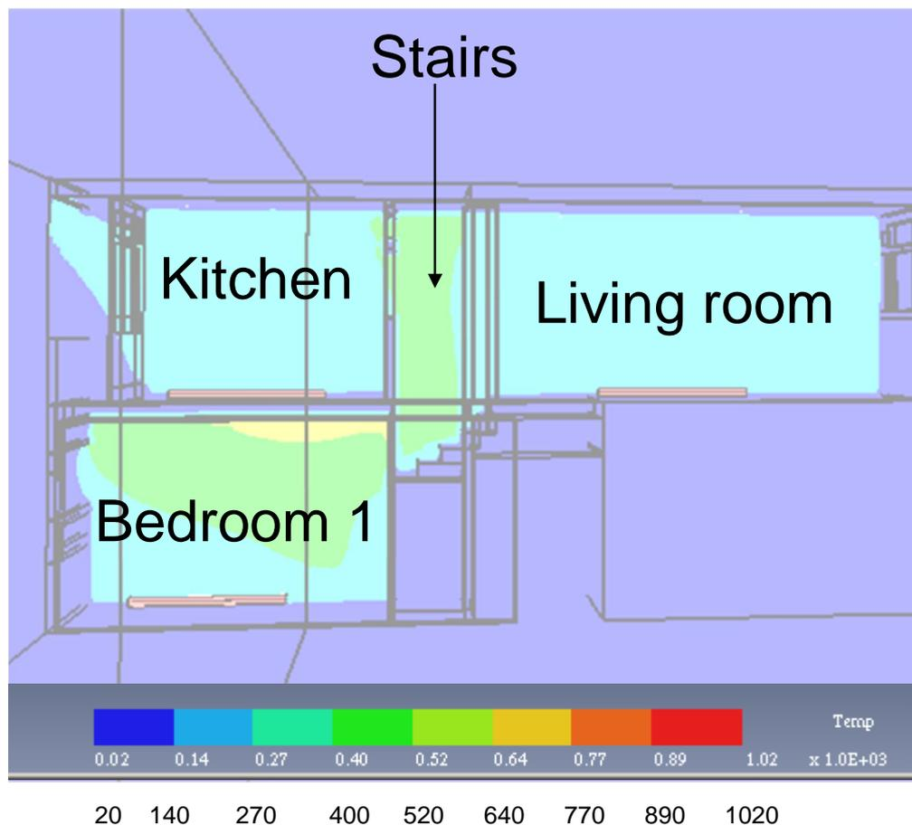
**Figure 112 – Wire frame image (i.e. wall and object outlines only) of Flat 65 used to display JASMINE simulation results<sup>140</sup>**
