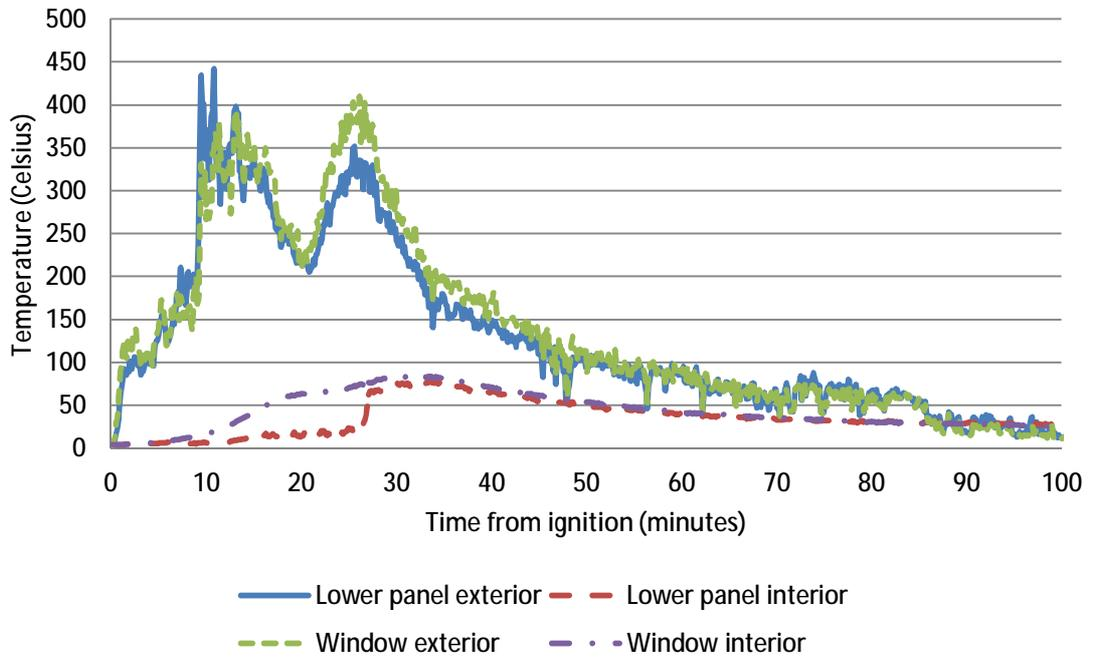
**Figure 89 – Temperature data at thermocouple positions on window E<sup>140</sup>**
