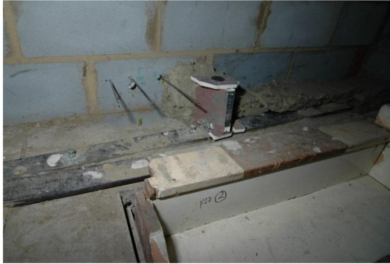
**Figure 70 – Gas sampling points at top of staircase in headspace of reconstruction rig<sup>142</sup>**
