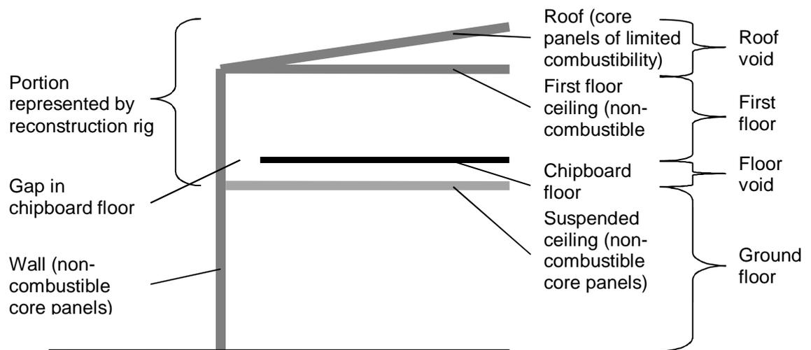
**Figure 141 – Portion of Wealmoor Atherstone elevation Section B that it represented by reconstruction rig**
