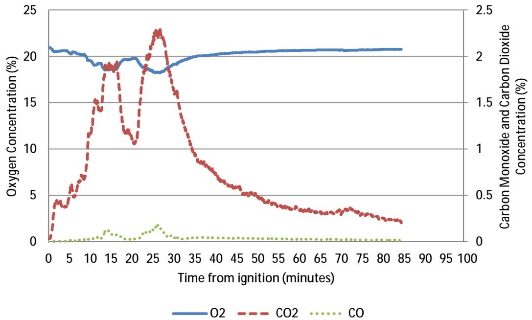
Figure 101 – Gas concentrations measured by 9m calorimeter (collecting gases from above bedroom façade)<sup>143</sup>
