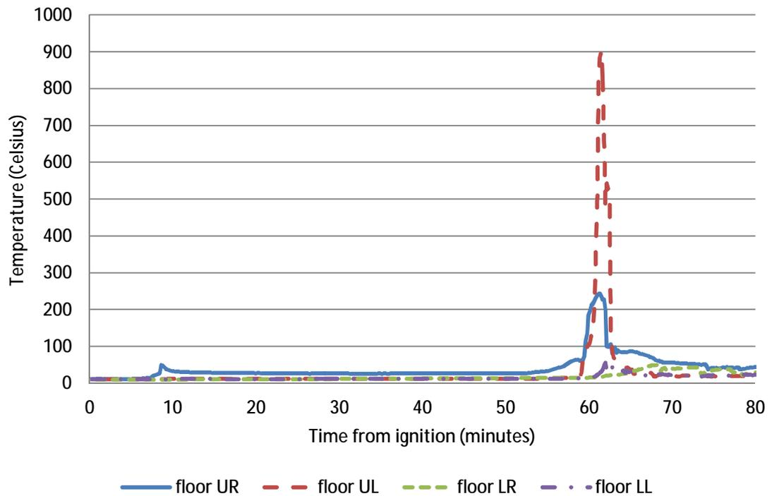
**Figure 161 – Temperature data at thermocouples located on upper and lower surfaces of suspended floor during Reconstruction 2**
