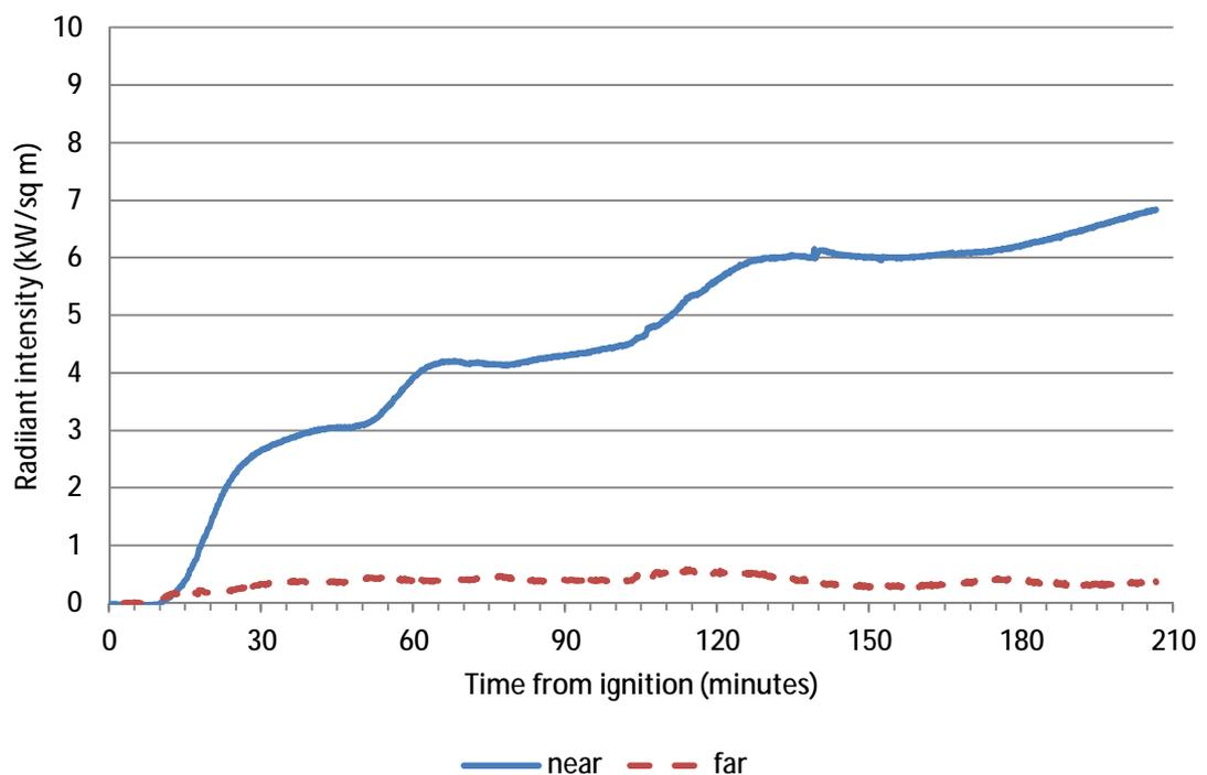
**Figure 154 – Radiant heat fluxes measured at floor level inside the corridor 2m (near) and 4m (far) away from the front edge of the room during Reconstruction 1**
