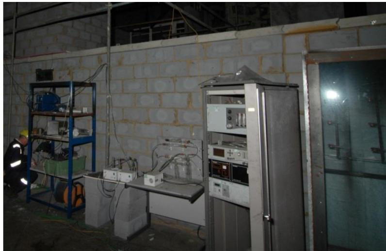
**Figure 71 – Gas analysers for continuous gas analysis and bubblers for discrete samples<sup>142</sup>**
