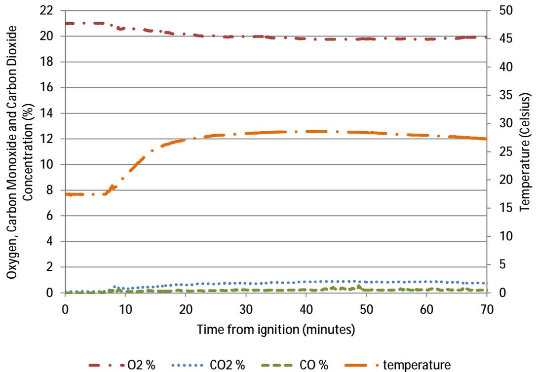
**Figure 35 – Gas concentrations measured in Rosepark closed room condition**
