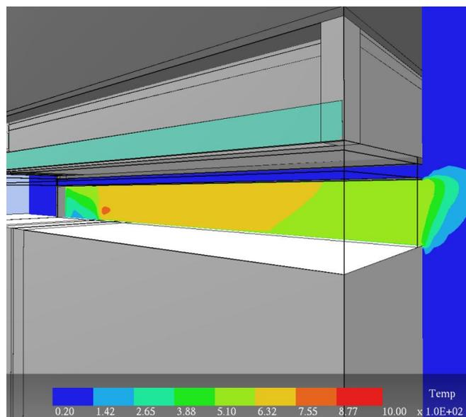
Figure 124 – JASMINE predicted temperature contours in the corridor<sup>140</sup>
