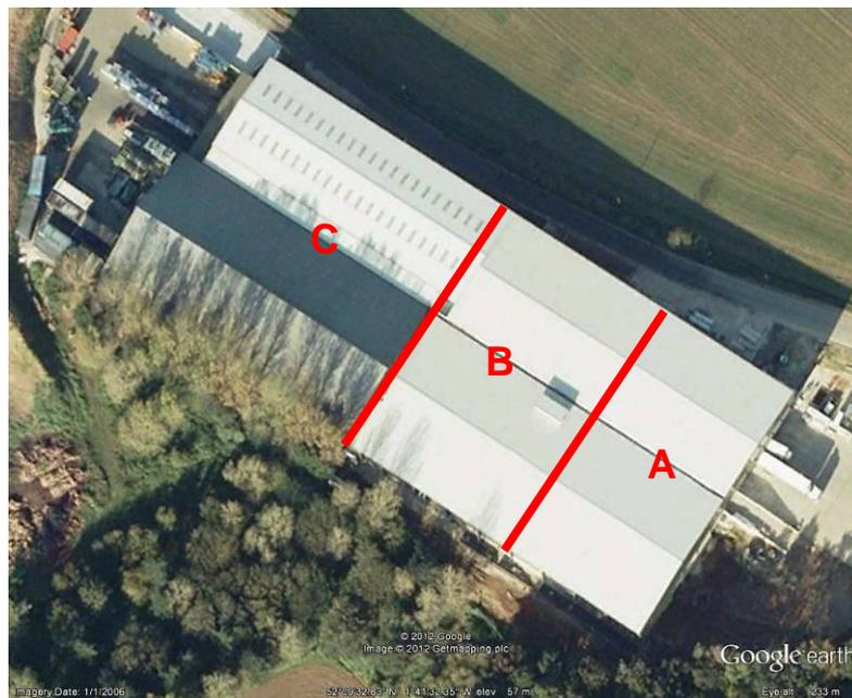
**Figure 140 – Aerial view of Wealmoor Atherstone prior to fire showing three sections identified by Hereford and Worcester Fire and Rescue Service fire investigation. The fire started in the first floor of Section B. Image from Google Earth, dated December 2006 (© 2012 Getmapping Plc, © 2012 Google)**
