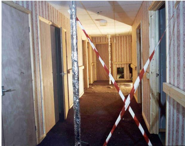
**Figure 29 – View of corridor in Rosepark reconstruction rig. The door to the cupboard where the fire started is slightly ajar on the left hand side. One of the thermocouple columns can be seen in the foreground**
