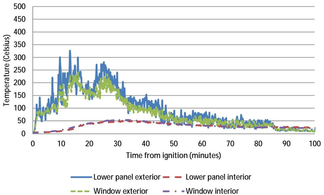
**Figure 90 – Temperature data at thermocouple positions on window F<sup>140</sup>**
