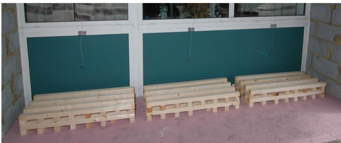
**Figure 74 – Wood cribs in place in front of windows of reconstruction rig<sup>140</sup>**
