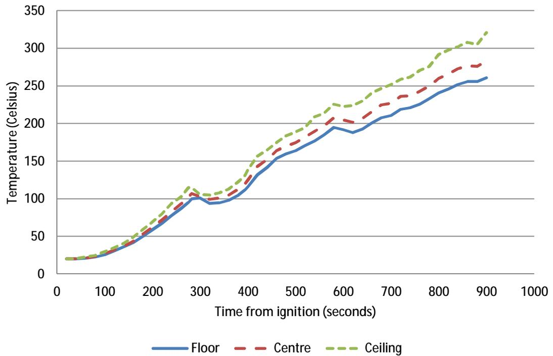
**Figure 119 – Flat 79 JASMINE simulation temperatures<sup>140</sup>**
