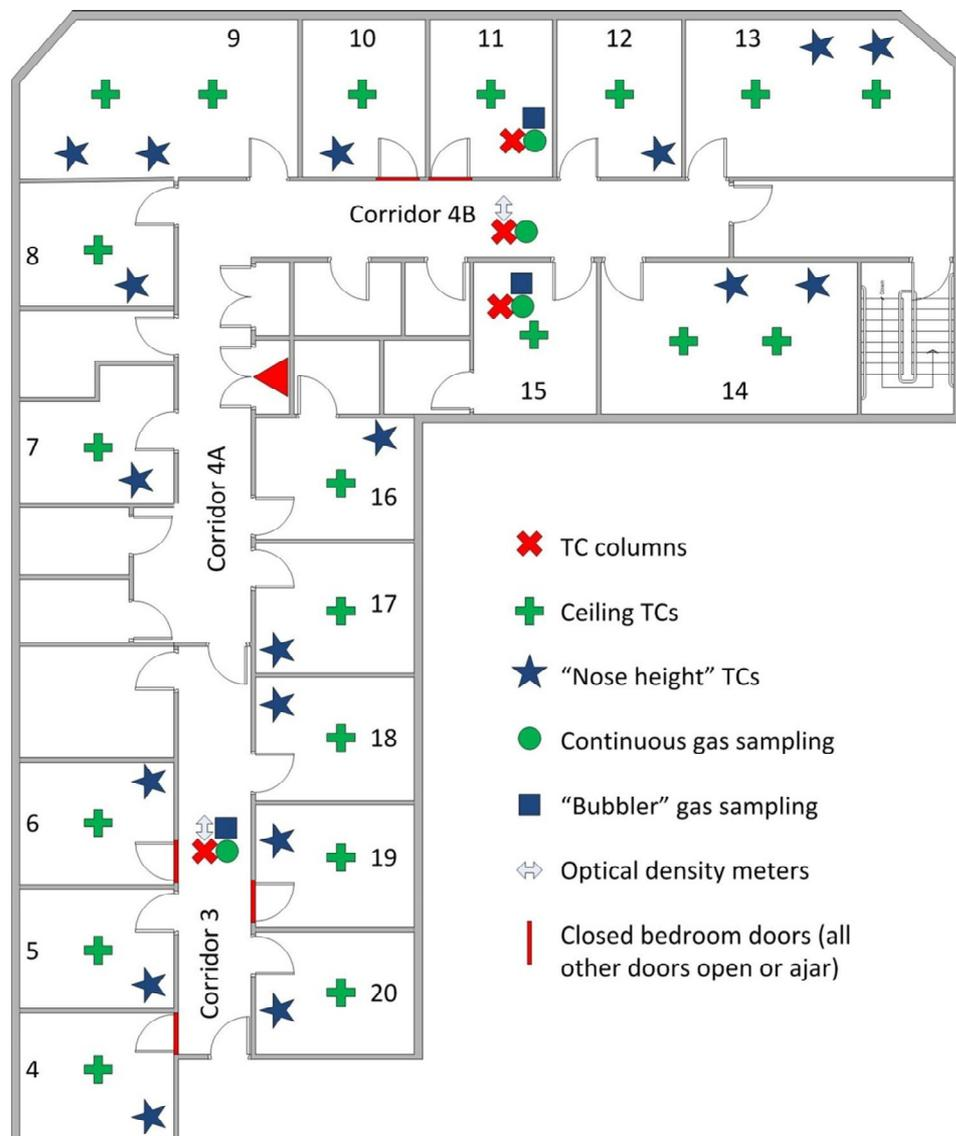
Figure 31 – Plan of instrumentation installed into Rosepark reconstruction rig
