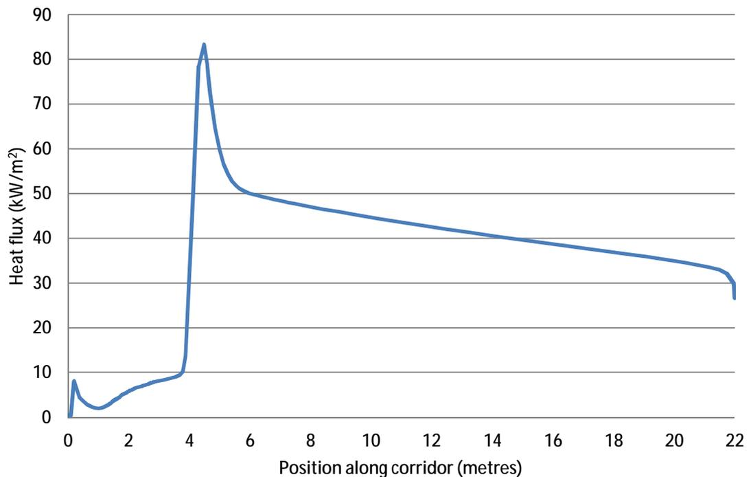
**Figure 125 – Heat flux to surfaces in 11<sup>th</sup> floor corridor<sup>140</sup>**
