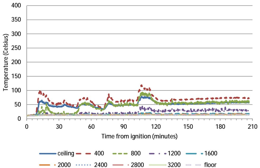
**Figure 151 – Temperature data at thermocouple tree D during Reconstruction 1**
