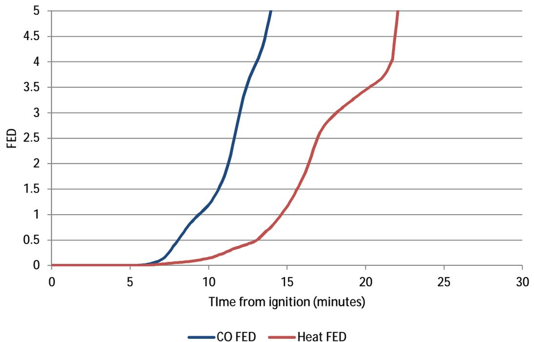
**Figure 138 – FED values calculated using ISO 13571 method based upon Lakanal reconstruction data relevant to the fatality in Flat 79**
