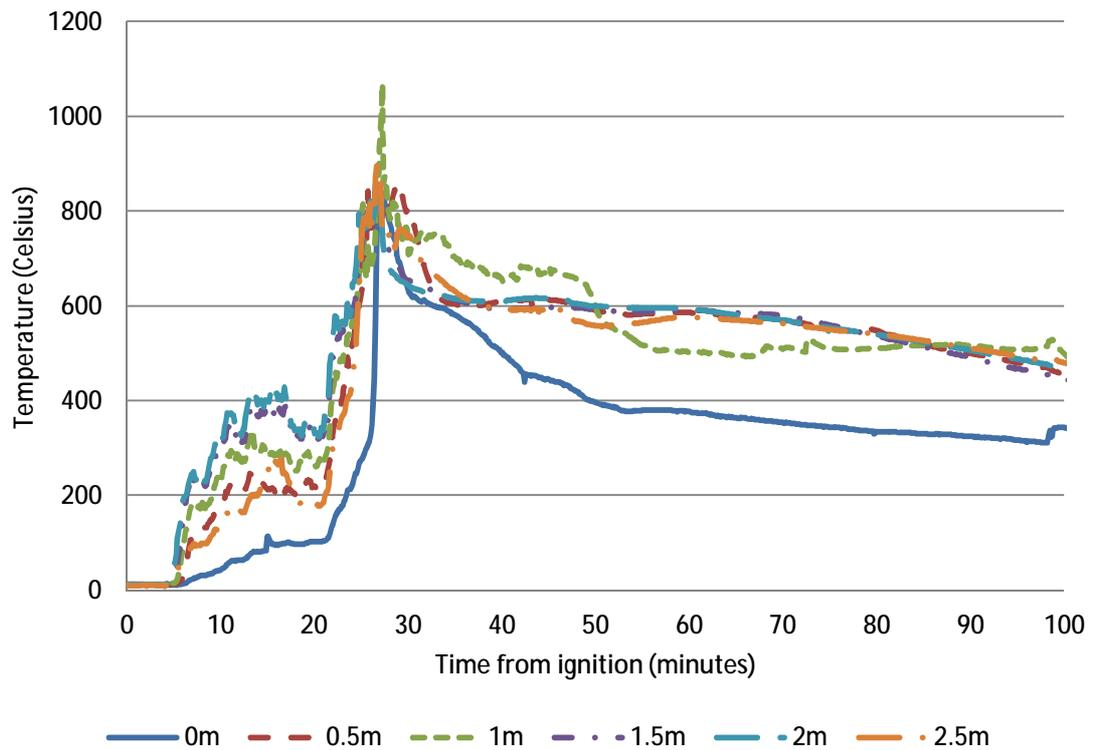
Figure 79 – Temperature data at thermocouple tree E<sup>140</sup>
