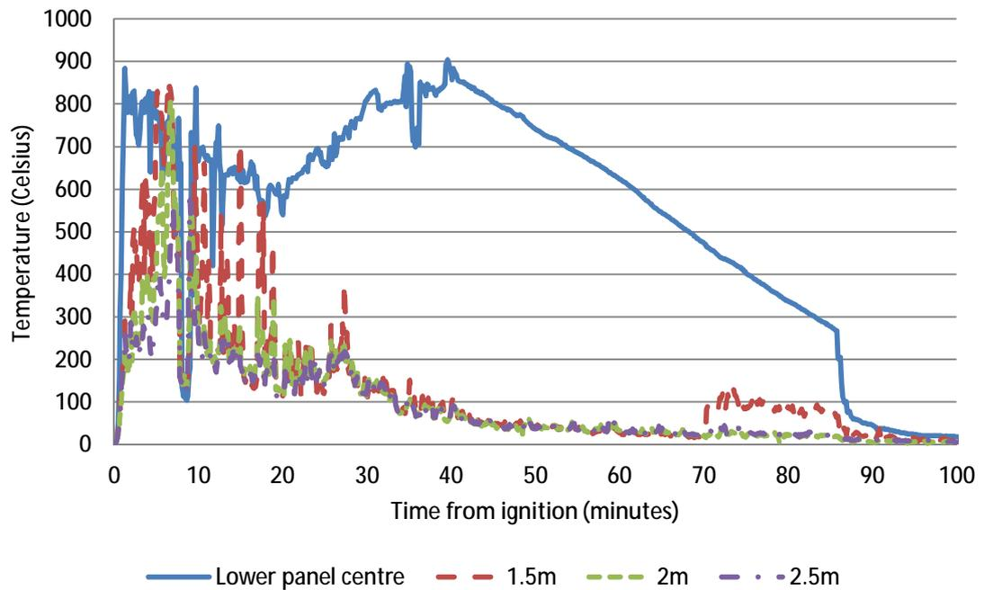
**Figure 86 – Temperature data at thermocouple positions on window C<sup>140</sup>**
