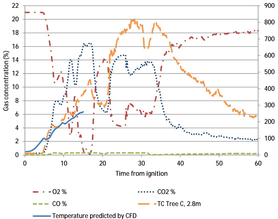
**Figure 136 – Data used from Lakanal reconstruction data headspace measurements for FED calculations**
