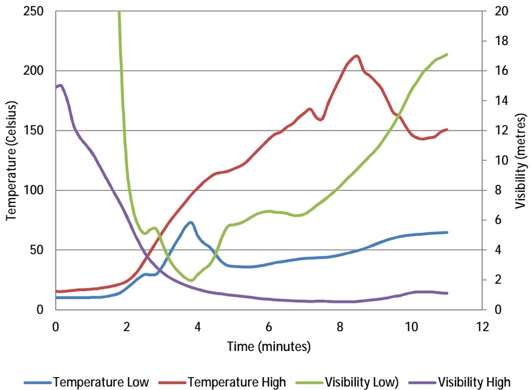
**Figure 176 – Temperature and visibility in the lift corridor at location L (shown on Figure 168) for Scenario 4**
