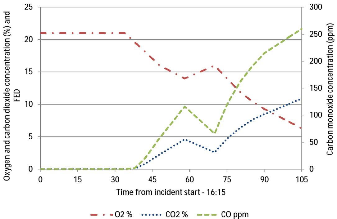
**Figure 137 – Data used from Lakanal Flat 81 gas concentration calculations for FED calculations**
