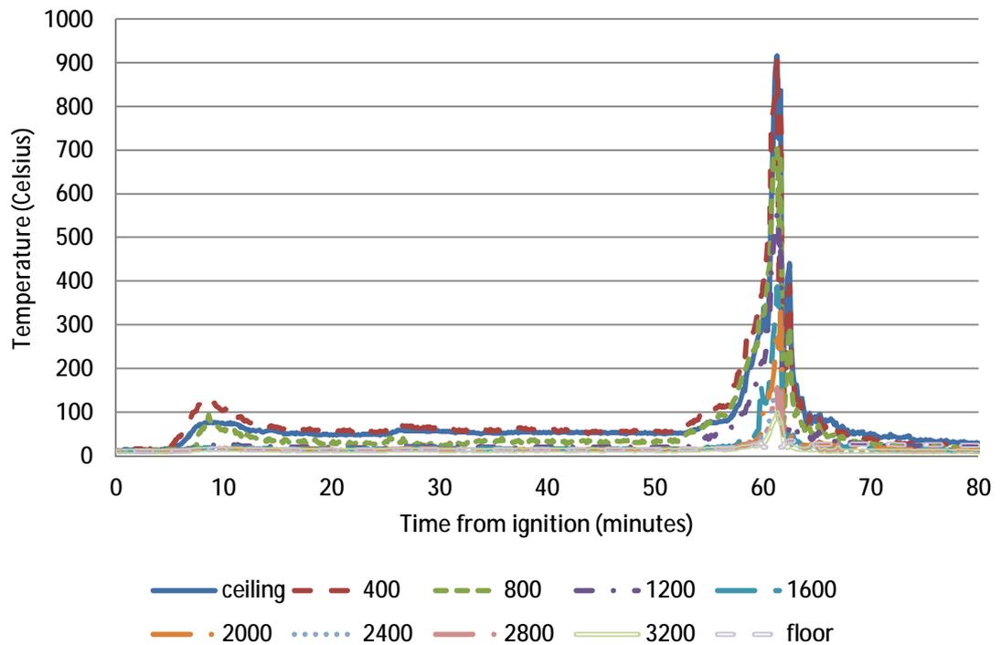
**Figure 158 – Temperature data at thermocouple tree C during Reconstruction 2**
