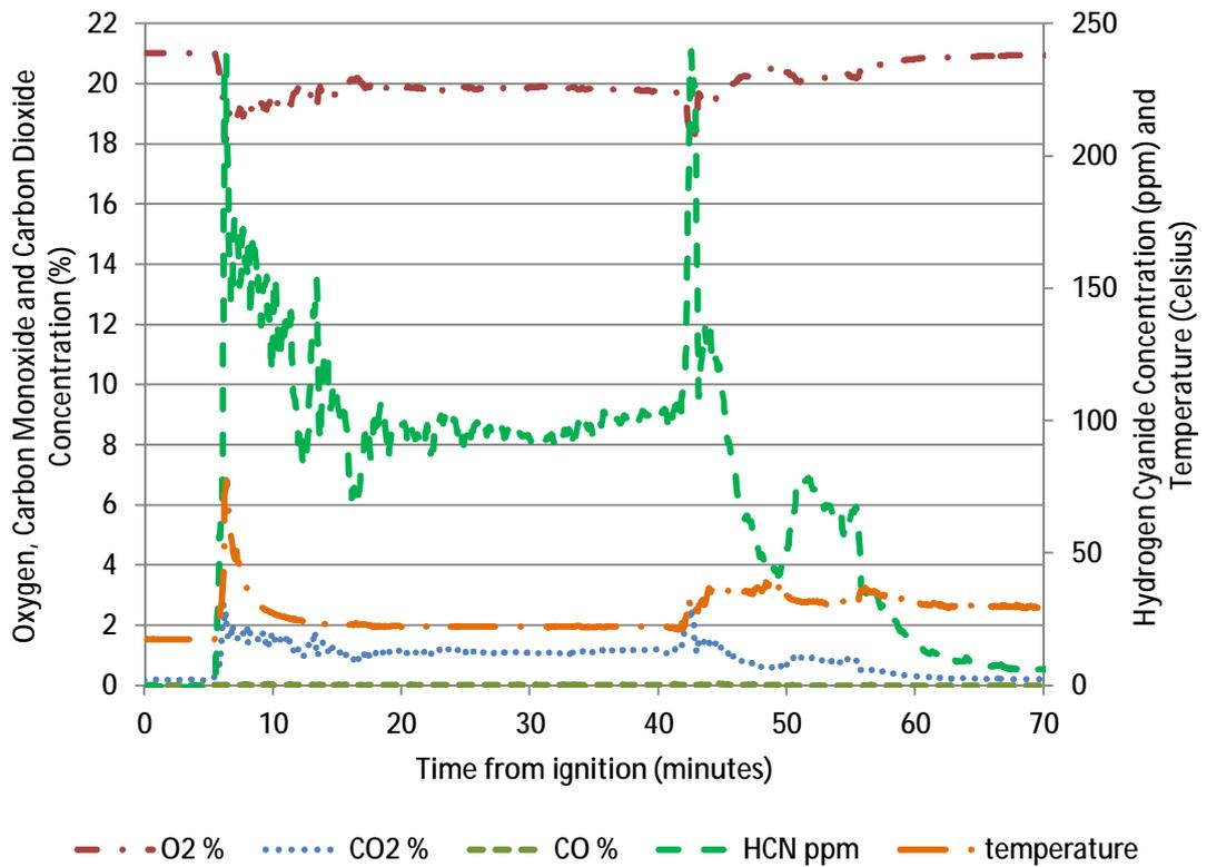
**Figure 33 – Gas concentrations measured in Rosepark corridor 3 (corridor off of fire corridor)**
