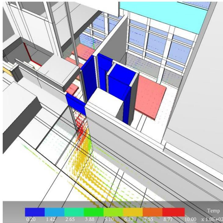
**Figure 127 – Flow of hot gases into the corridor<sup>140</sup>**
