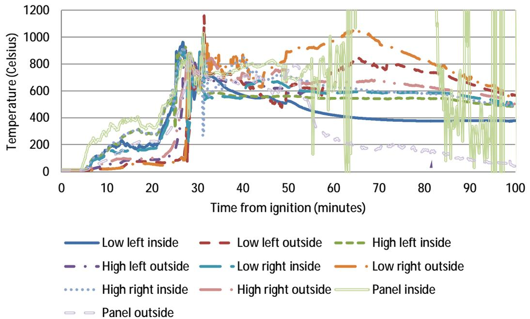
**Figure 94 – Temperature data at thermocouple positions on door C<sup>140</sup>**
