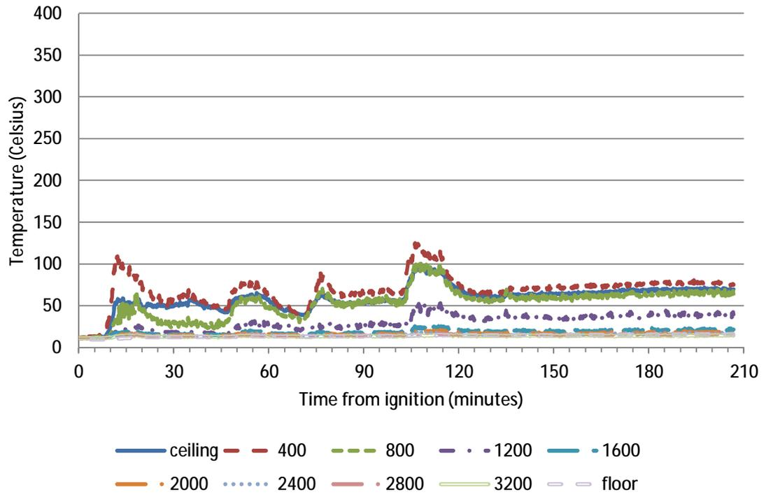
**Figure 150 – Temperature data at thermocouple tree C during Reconstruction 1**
