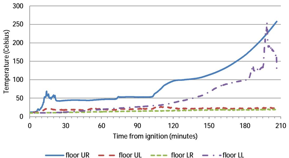
**Figure 153 – Temperature data at thermocouples located on upper and lower surfaces of suspended floor during Reconstruction 1**
