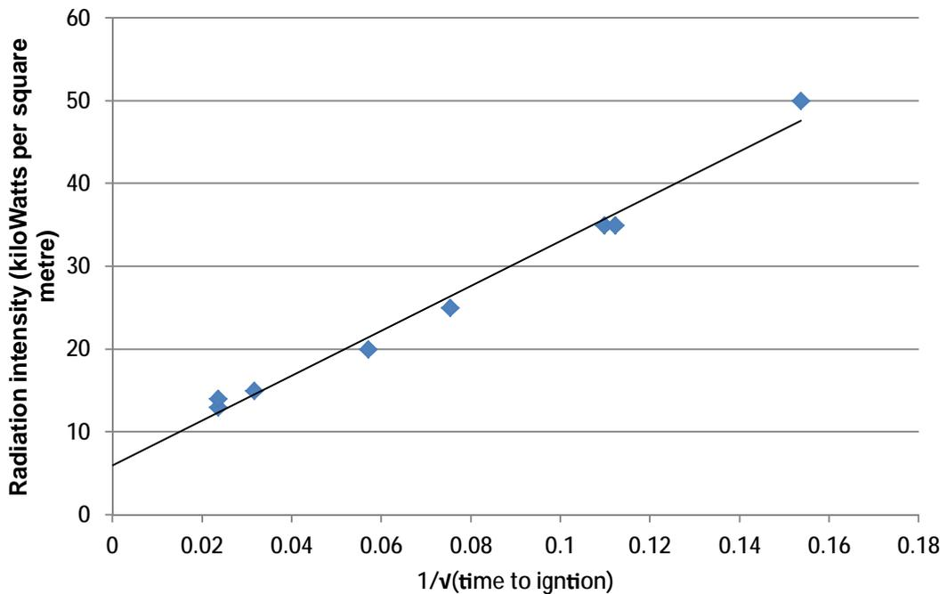
Figure 164 – Critical irradiance plot from cone calorimeter tests on particle board flooring
