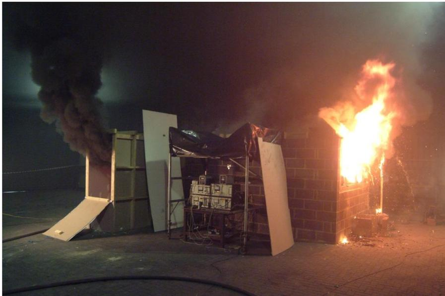
**Figure 41 – View of outside of reconstruction rig during fire, showing venting out of window and into corridor<sup>138</sup> (see Appendix A)**
