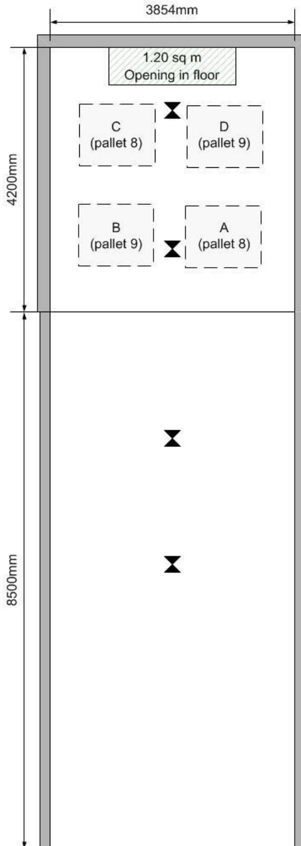
Figure 142 – Layout of Atherstone reconstruction rig, showing the positions of the four pallets in each reconstruction and the opening to the rear of the rig
