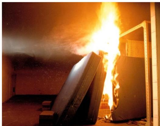
**Figure 22 – Plate number 7 from the FRS report into the Maysfield fire<sup>131</sup> (see Appendix A) showing the full-scale flaming test 4 minutes 30 seconds after ignition**
