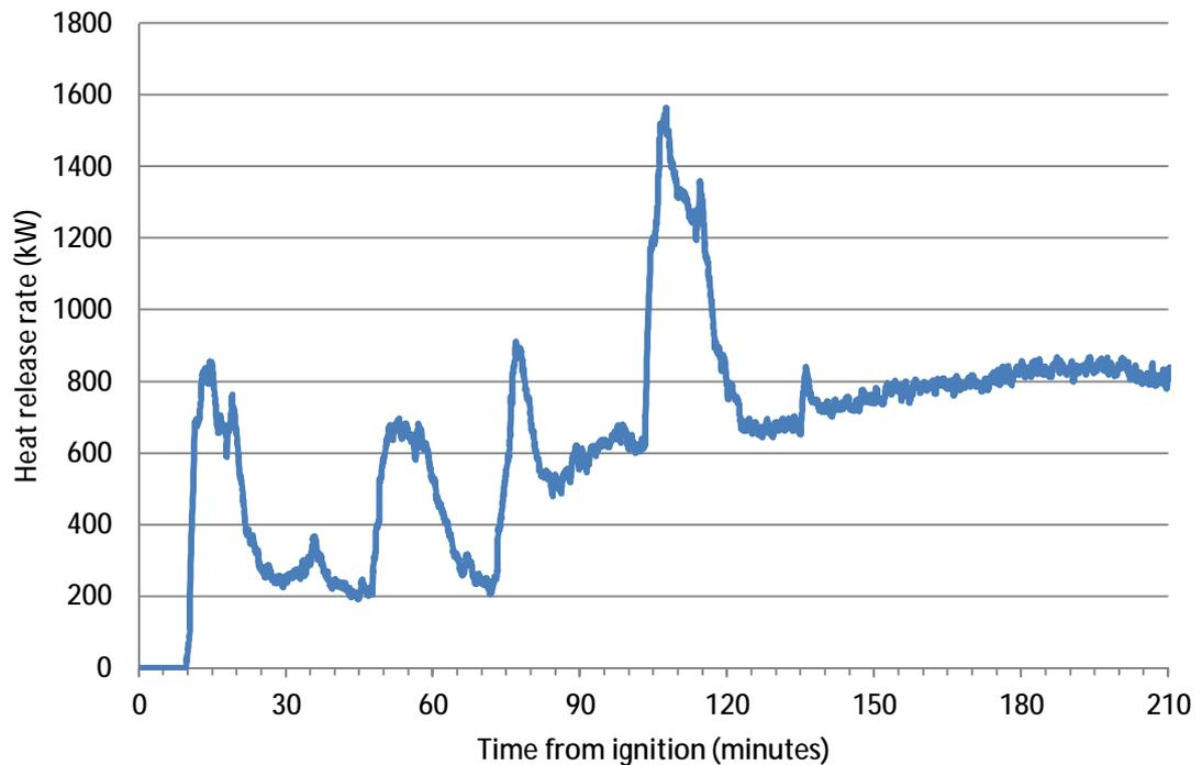
**Figure 155 – Heat release rate data during Reconstruction 1**
