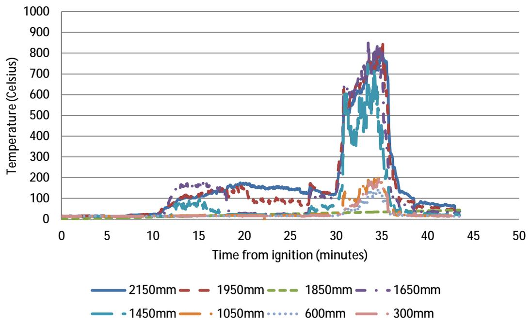
**Figure 44 – Temperatures measured in reconstruction fire in Harrow Court corridor at heights from floor<sup>138</sup>**
