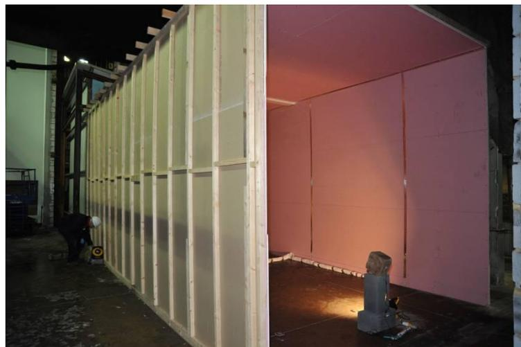
**Figure 144 – External view of timber frame and plasterboard corridor prior to reconstruction**
