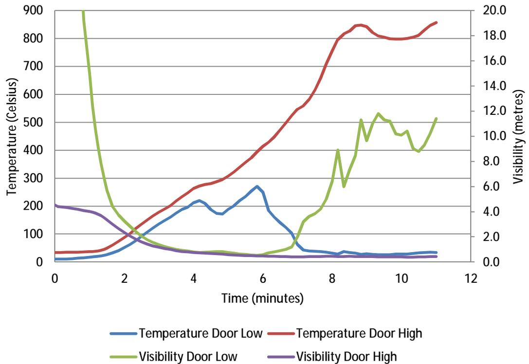
**Figure 178 – Data used from Atherstone modelling data for FED calculations. Time zero represents the time at which runaway fire spread started**
