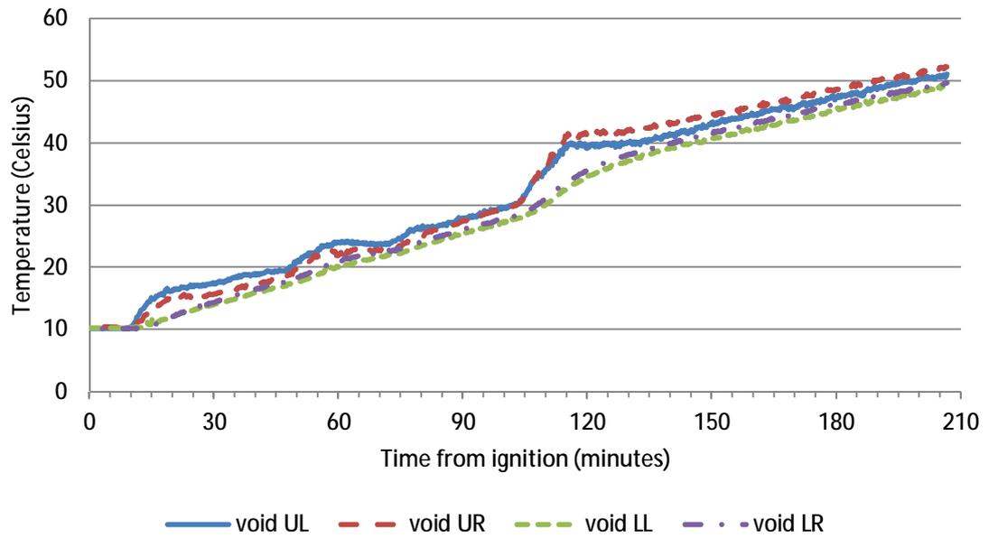
**Figure 152 – Temperature data at thermocouples located in ceiling void during Reconstruction 1**
