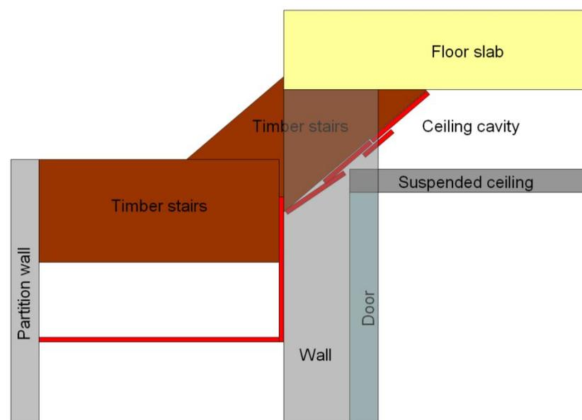
Figure 69 – Elevation section diagram of pieces of mineral fibreboard making up box beneath stairs. Wall position overlaid as transparent block<sup>140</sup>
