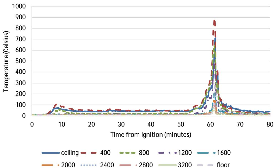
**Figure 159 – Temperature data at thermocouple tree D during Reconstruction 2**
