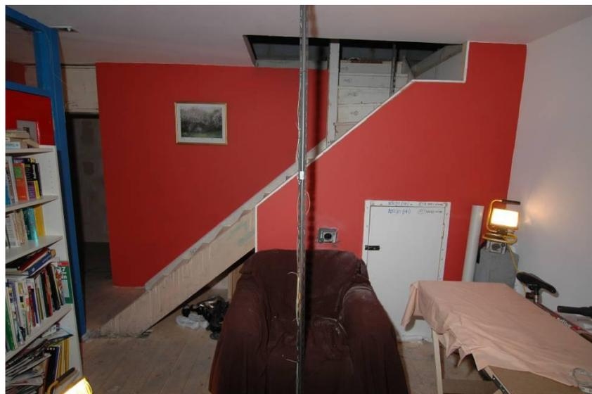
**Figure 67 – The staircase and modified partition wall fitted into the test rig<sup>140</sup>**
