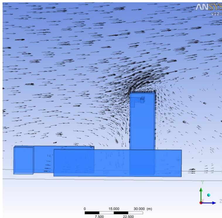
Figure 105 – Side view of vectors showing air flow around Lakanal House<sup>140</sup>
