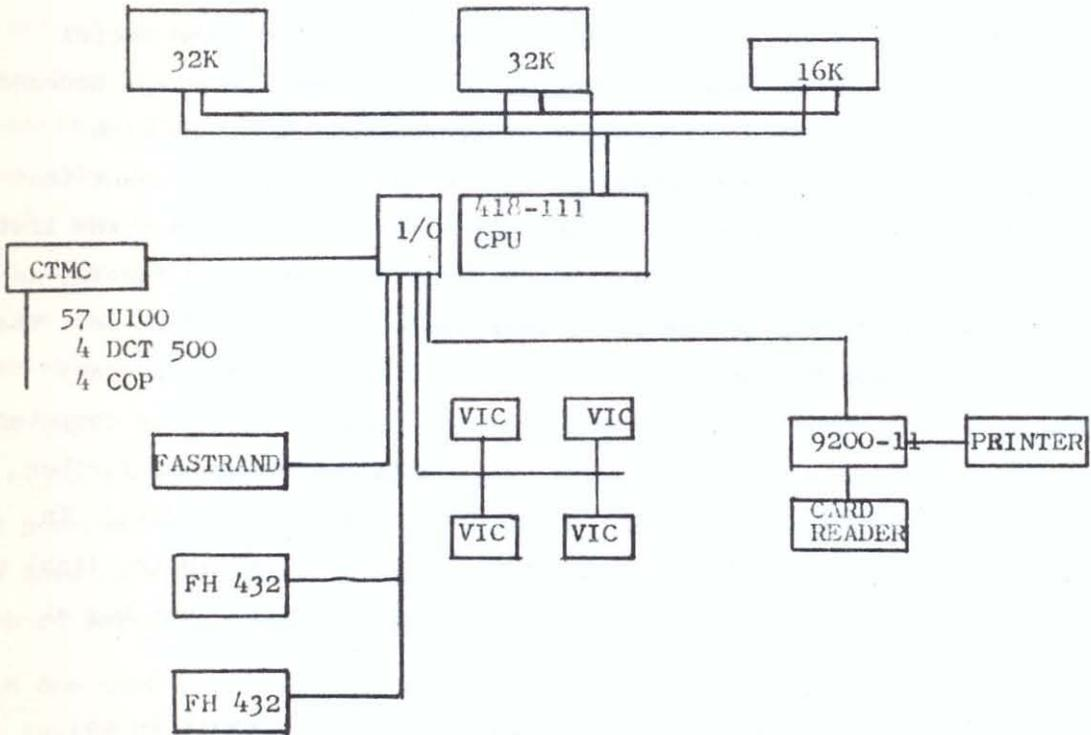
FIGURE 4 418-111 Batch Configuration
