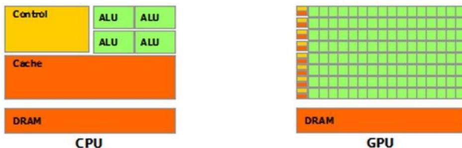
Figure 6.2: CPU and GPU architectures.
