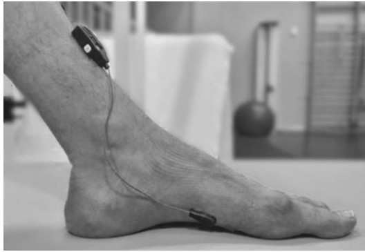
Figure 1. Trigno Mini wireless sensor placed on the foot for abductor hallucis muscle.
