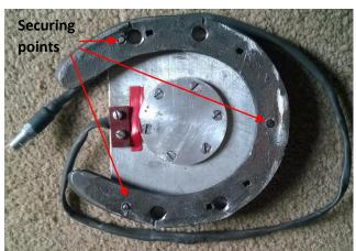
Plate 3: Dorsal view of the adapted aluminium housing secured to a used steel shoe in preparation for repeating the compression tests.
