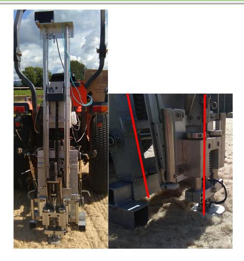
Plate 5.1.3: The OBST mounted onto a tractor
