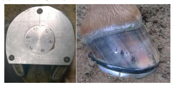
Plate 4a: Solar view of the prototype force shoe secured to the base of the right front shoe.
