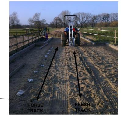
Plate 5.2.8: The OBST being used to test the 'horse track' and 'fresh track'. The small bags (n=10) contain the surface sample used to calculate moisture content.
