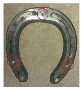
Plate 7.1.1: Modified steel shoe with three points of attachment prior to being fitted by the farrier
