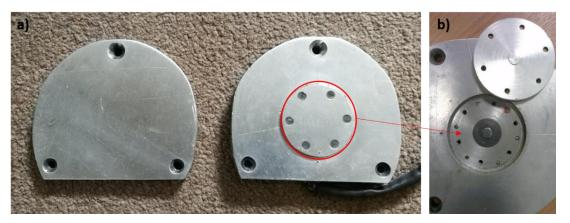
Plate 7.1.3 a: 'Dummy' force shoe (left) and prototype force shoe (right);b: The single axis button load cell (Interface LBS miniature compression load) secured beneath the plate.
