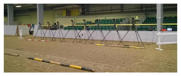
Plate 6: An 8 camera motion analysis system set up for an extended calibration
