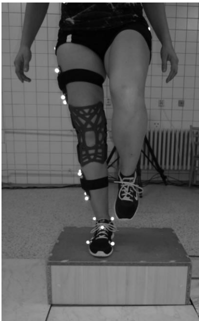
Fig. 1. Reaction Web Knee Brace and reflective markers placed on the foot, shank, and thigh using the Calibrated Anatomical System Technique.
