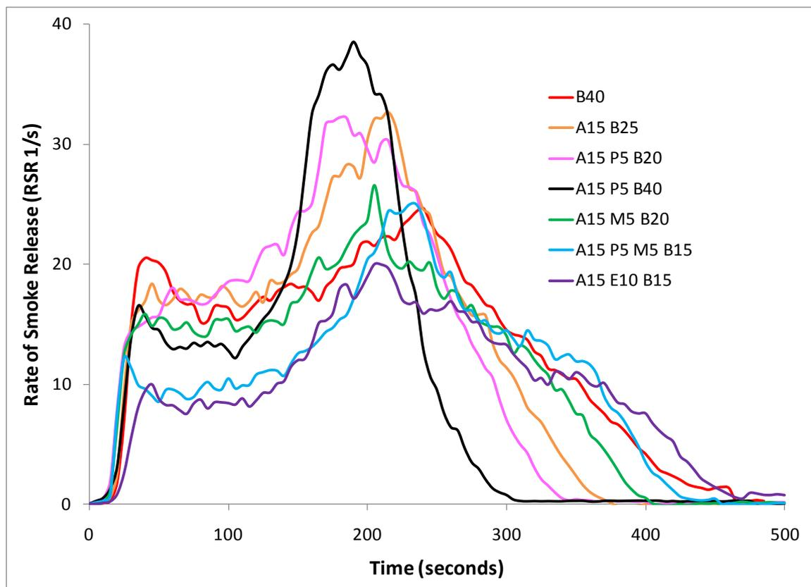
**Figure 57 Mean Rate of Smoke Release for APP formulations**
