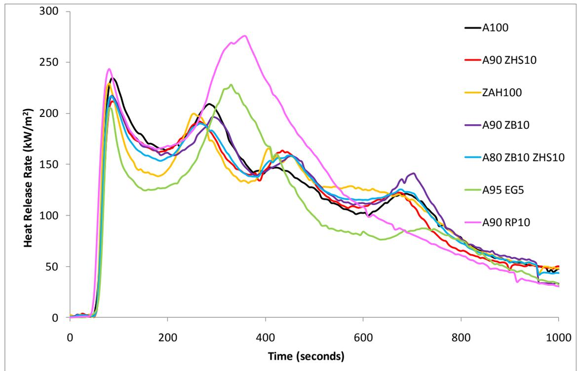
**Figure 86 Heat release rate from cone for ATH / synergist formulations**
