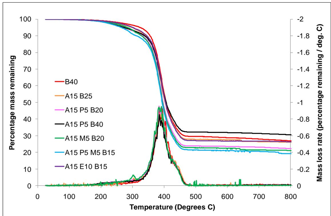
Figure 53 TGA and DTG curves for APP formulations in nitrogen
