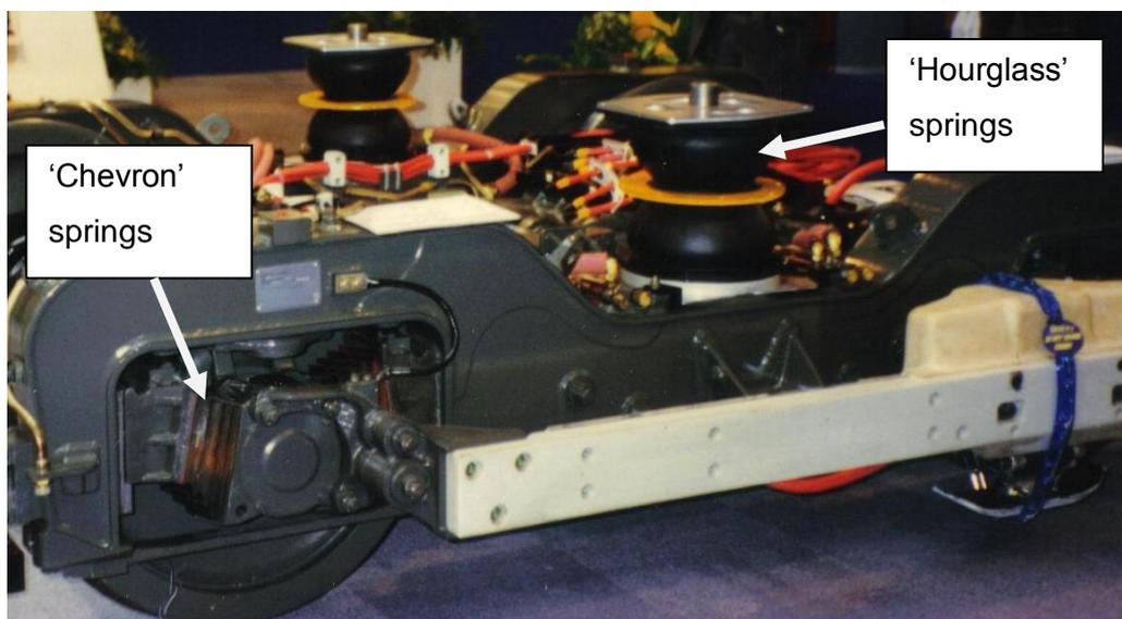
**Figure 2 Jubilee line bogie using TIAVS rubber suspension**
