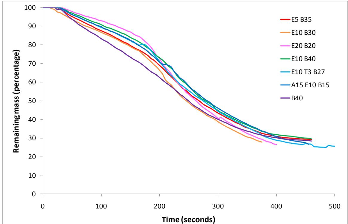
**Figure 61 Residual mass from cone calorimeter for expandable graphite formulations**
