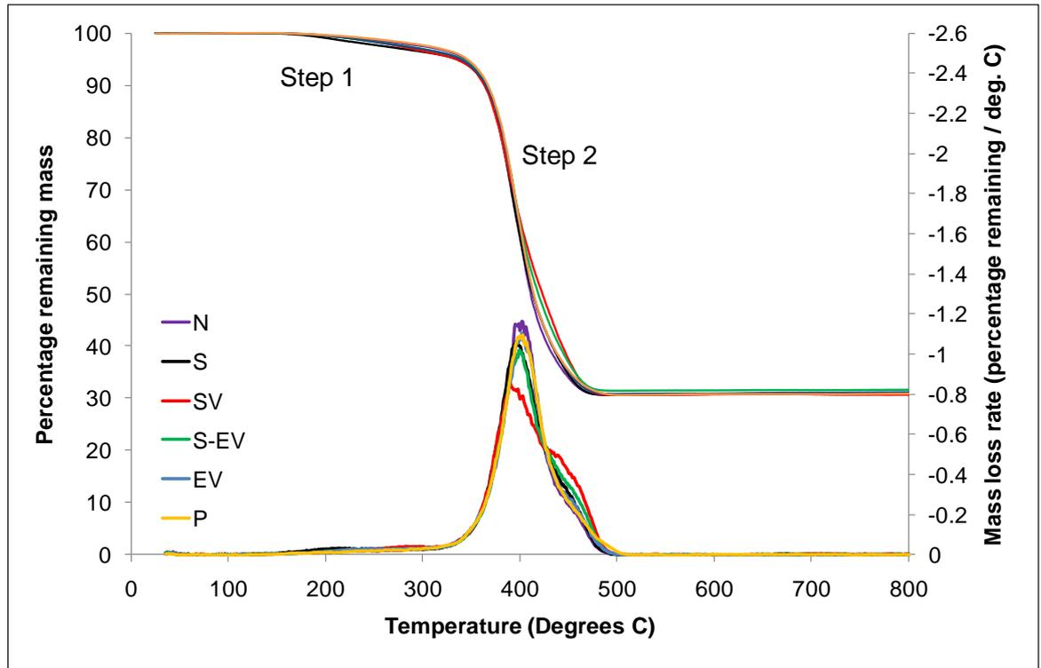
Figure 33 TGA and DTG curves for cross-linking formulations in nitrogen
