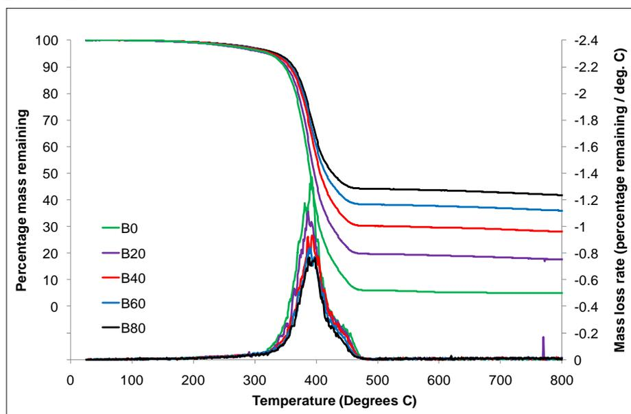
Figure 46 TGA and DTG curves for carbon black formulations in nitrogen
