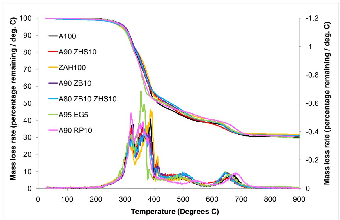
**Figure 83 TGA and DTG curves for ATH / synergist formulations in air**
