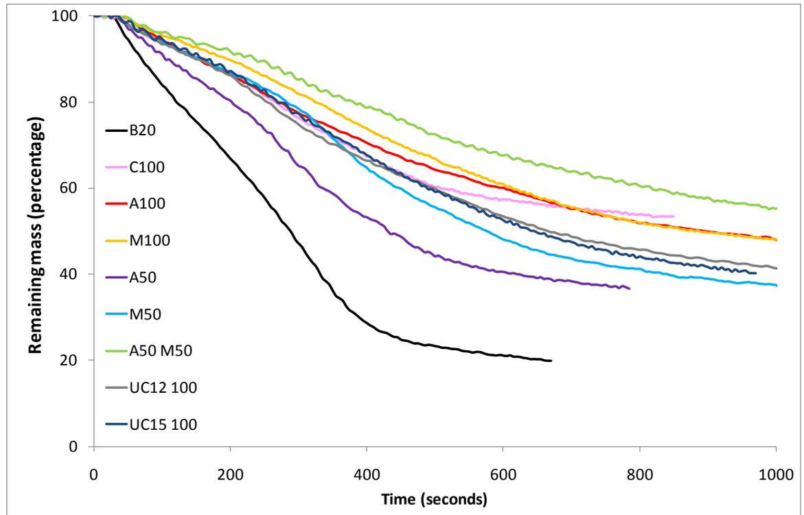
**Figure 72 Residual mass from cone calorimeter for hydrated filler formulations**
