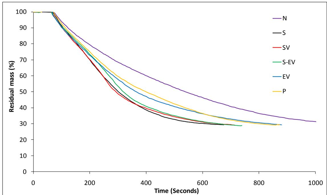
**Figure 38 Residual mass from cone calorimeter for cross-linking formulations**
