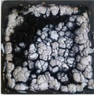
M100 has a noticeably stronger and complete residue, although still not continuous.
