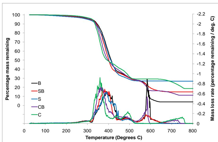
Figure 42 TGA and DTG curves for varied filler formulations in air
