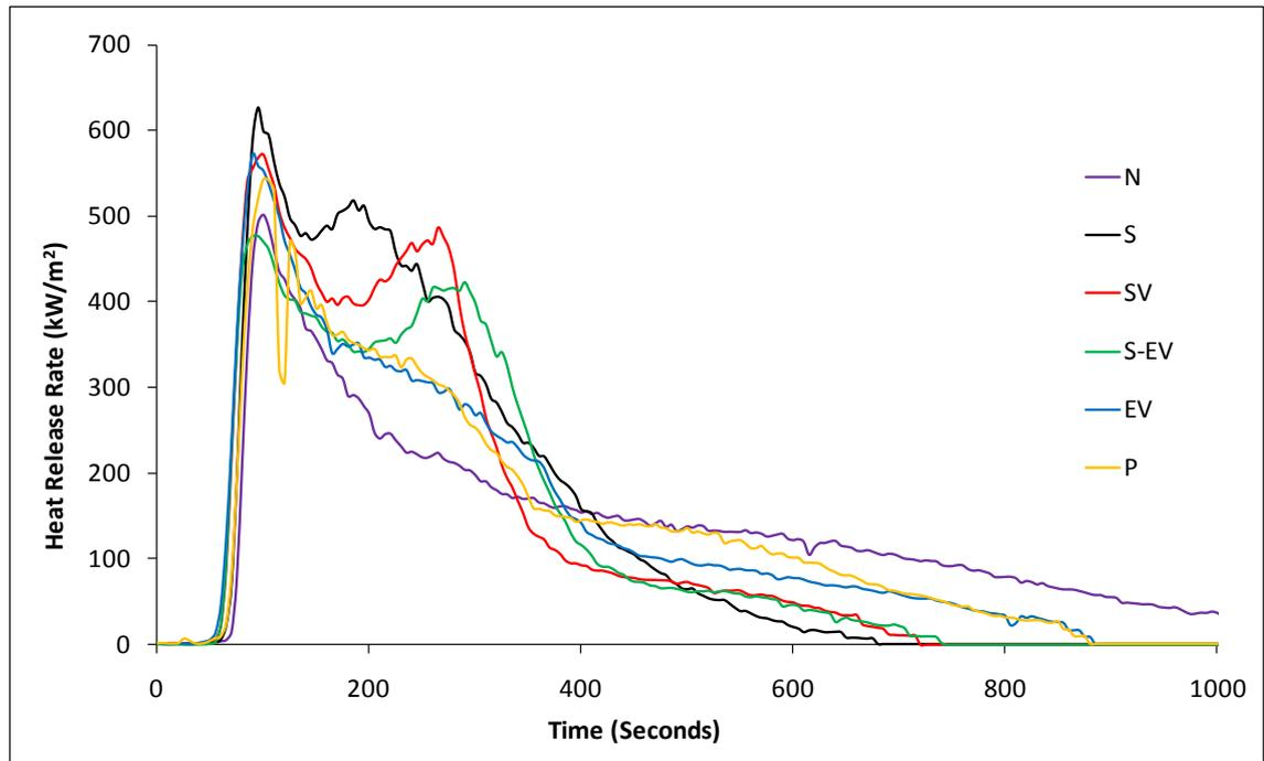
**Figure 37 Heat release rate from cone calorimeter for cross-linking formulations**
