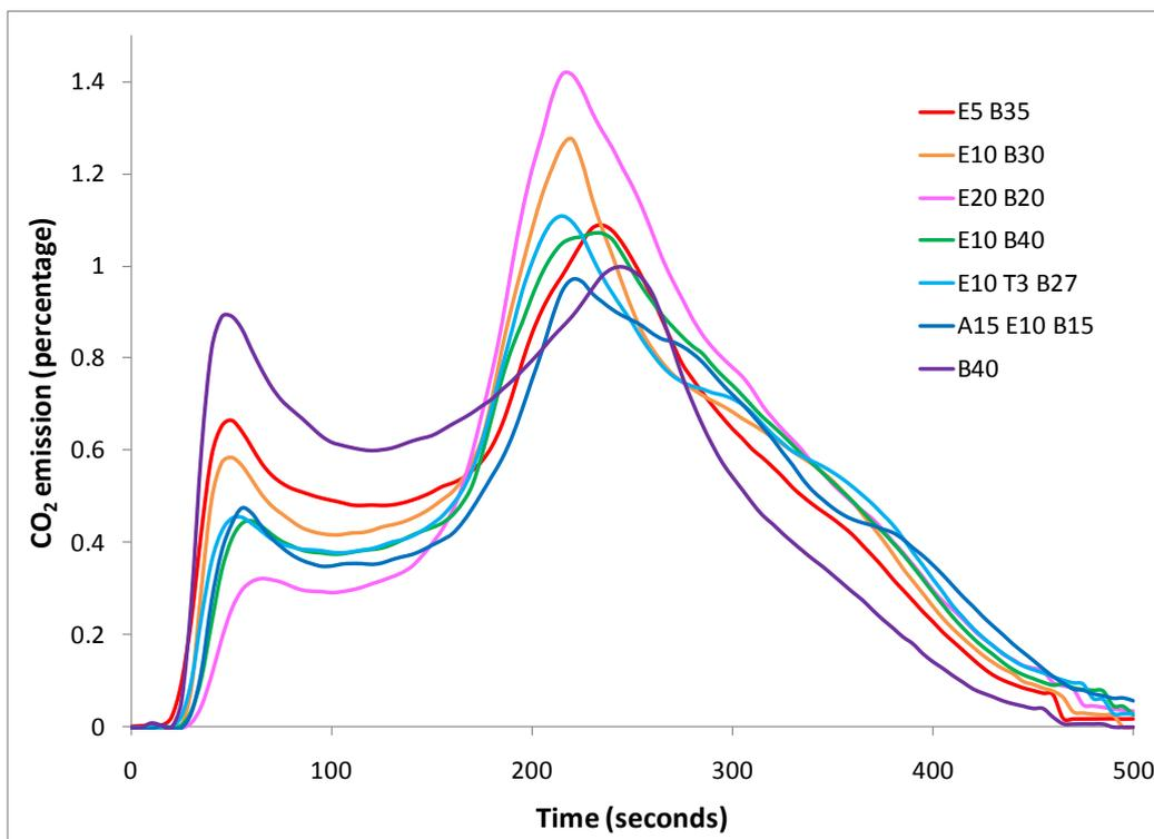
Figure 62 CO<sub>2</sub> emissions from cone for expandable graphite formulations
