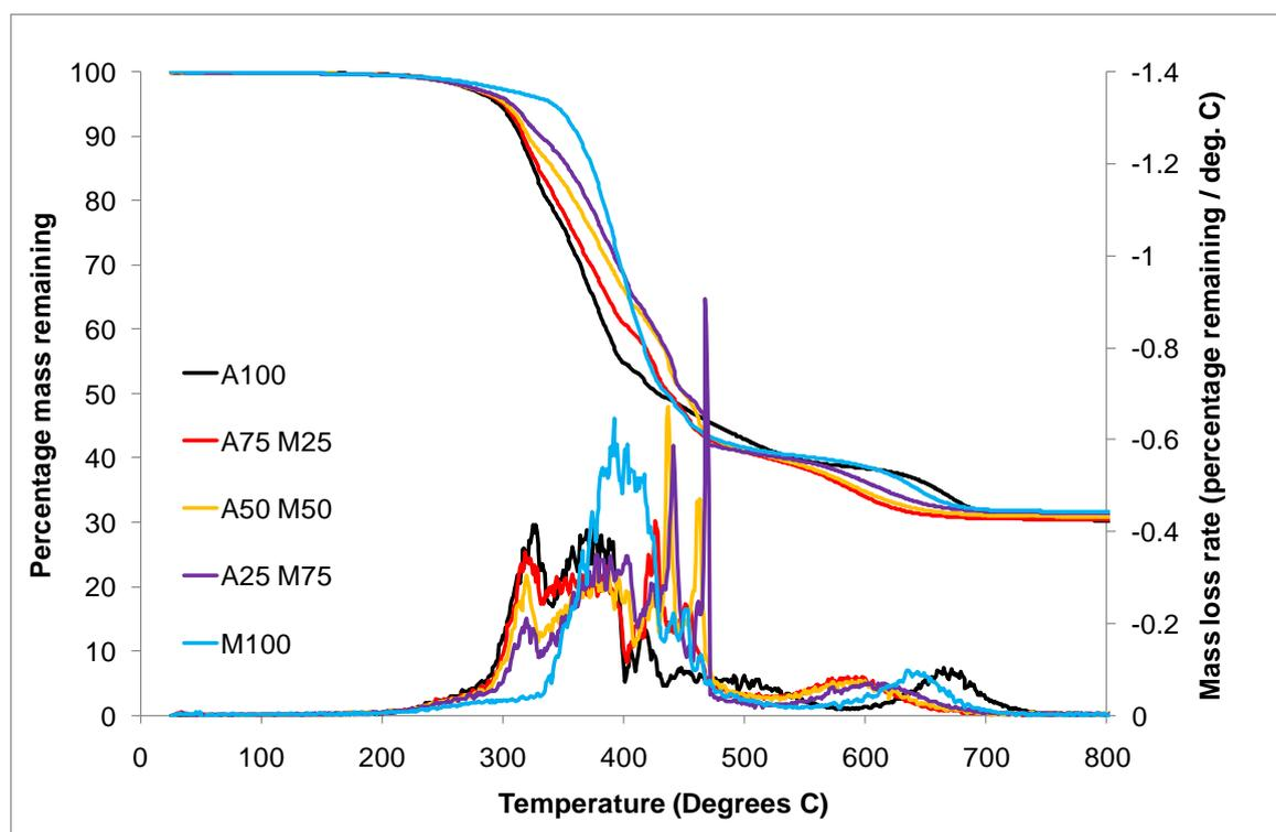
**Figure 104 TGA and DTG curves for ATH / MH blend formulations in air**
