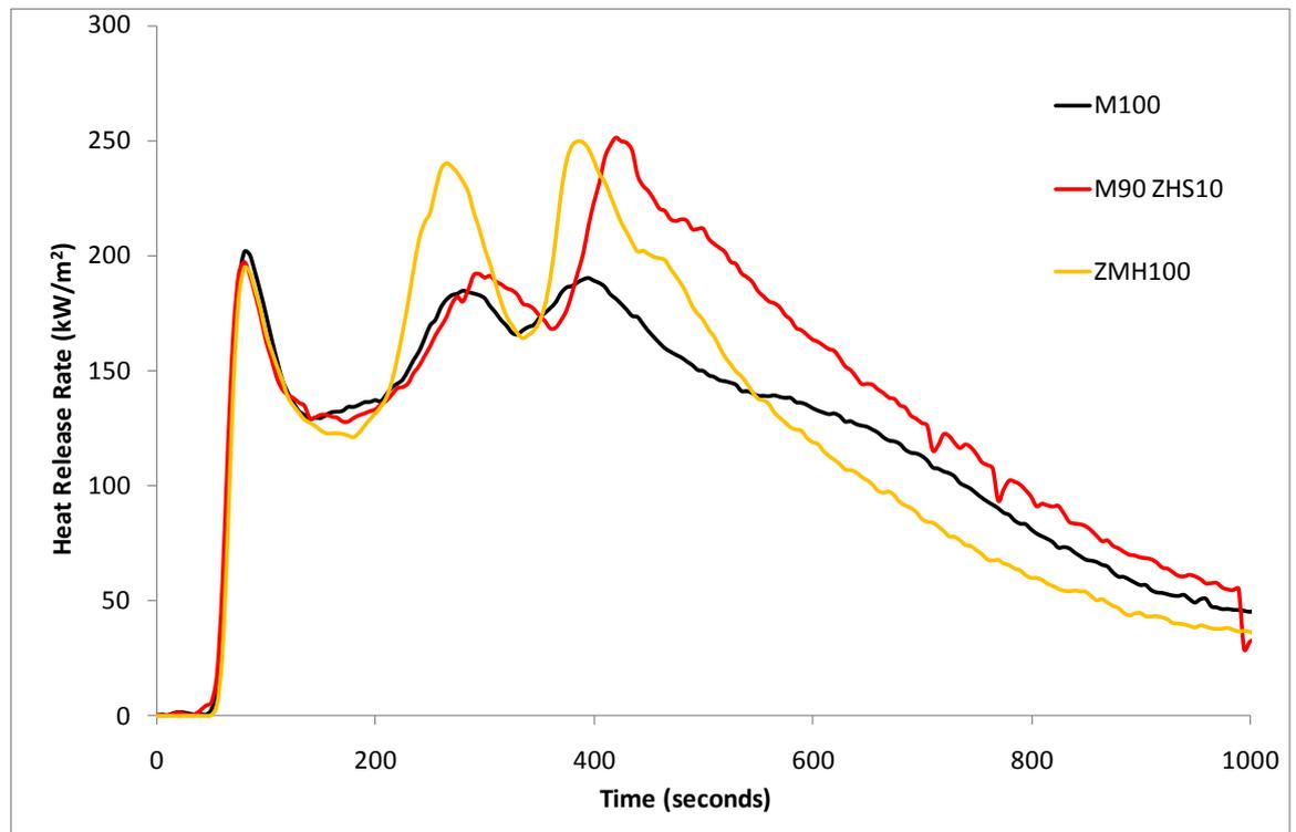
**Figure 87 Heat release rate from cone for MH / ZHS formulations**
