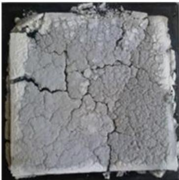
The use of calcium carbonate leads to an almost continuous and rigid residue structure, broken by long cracks along areas of weakness.
