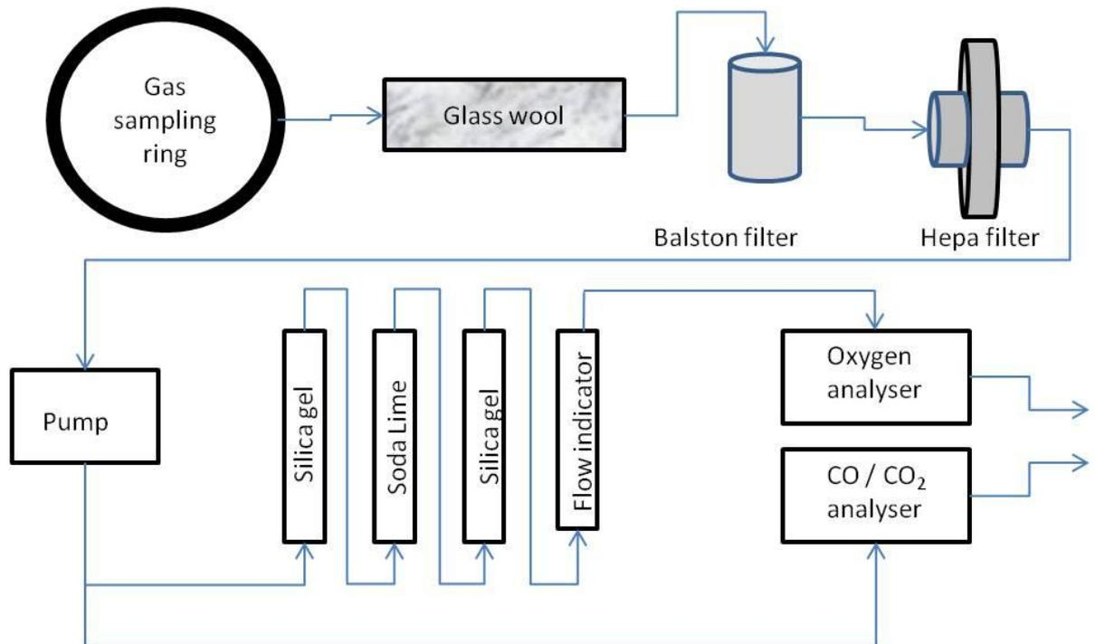
**Figure 22 Schematic view of sample gas flow in cone calorimeter**
