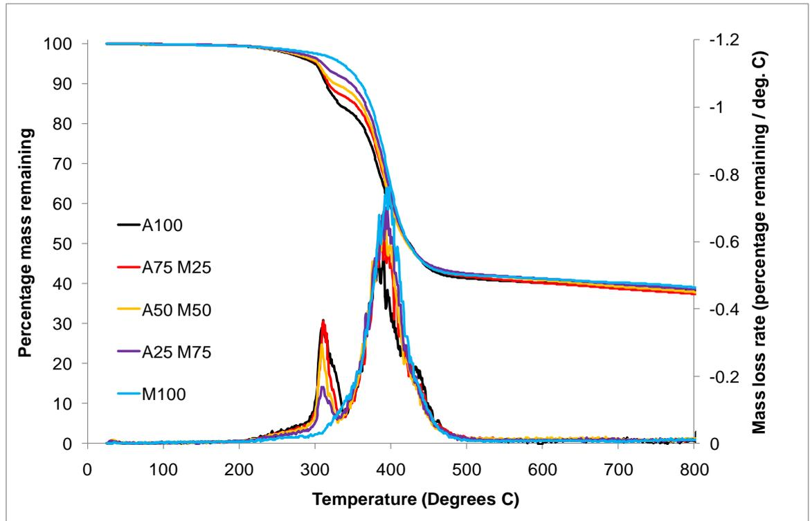
Figure 103 TGA and DTG curves for ATH / MH blend formulations in nitrogen
