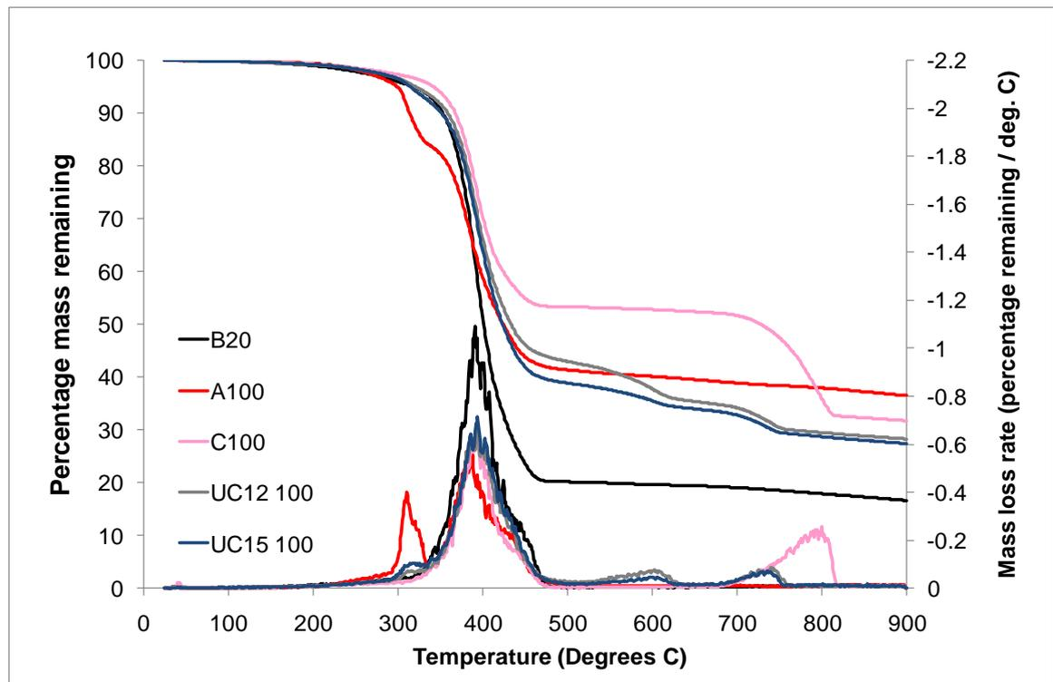
**Figure 67 TGA and DTG curves for selected hydrated filler formulations in nitrogen**
