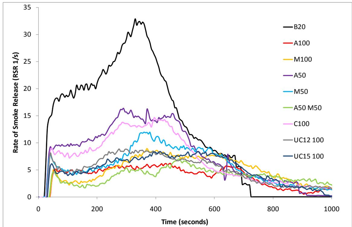
**Figure 73 Mean Rate of Smoke Release for hydrated filler formulations**
