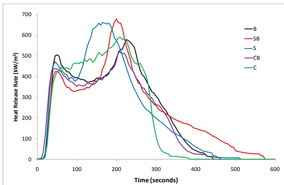
**Figure 43 Heat release rate from cone calorimeter for varied filler formulations**
