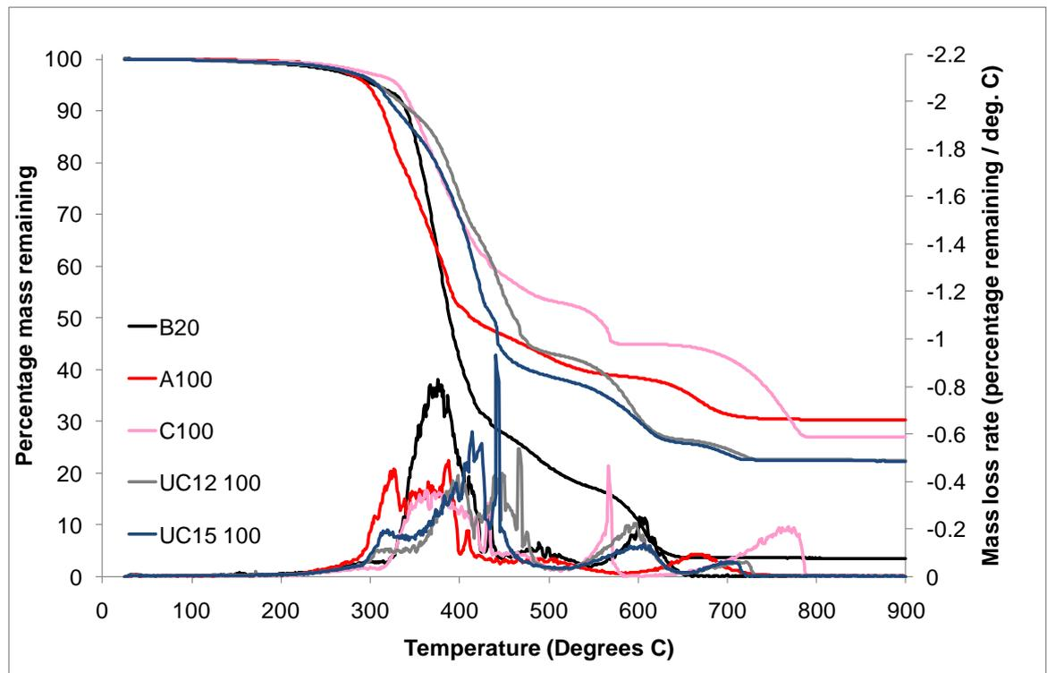
**Figure 68 TGA and DTG curves for selected hydrated filler formulations in air**
