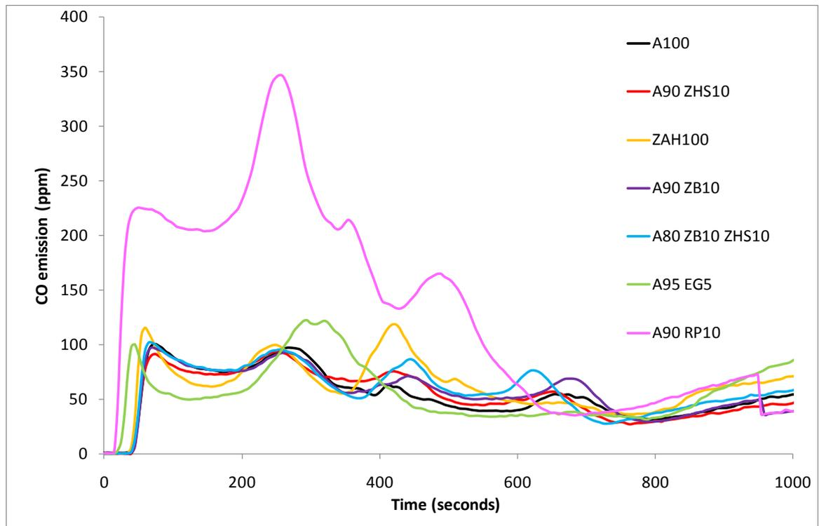
**Figure 89 mean CO ppm from cone for ATH / synergist formulations**
