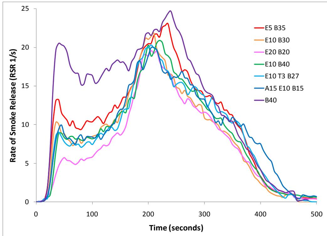
**Figure 64 Mean Rate of Smoke Release for expandable graphite formulations**
