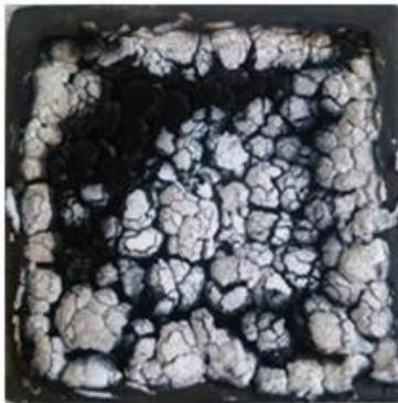
M100 has a noticeably stronger and complete residue than A100, although not continuous.
