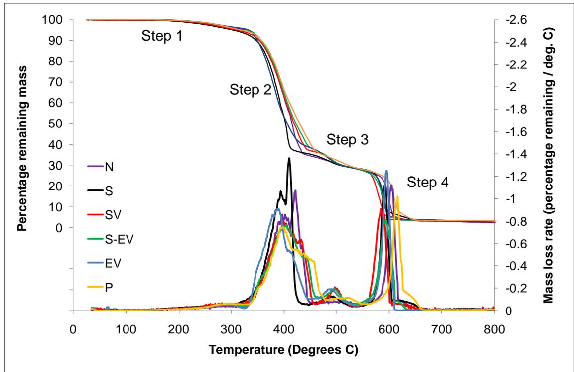
Figure 34 TGA and DTG curves for cross-linking formulations in air
