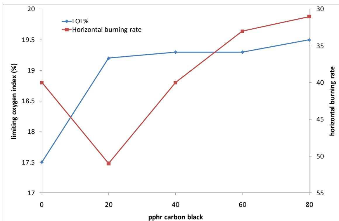
**Figure 48 LOI and horizontal burning values for carbon black formulations**
