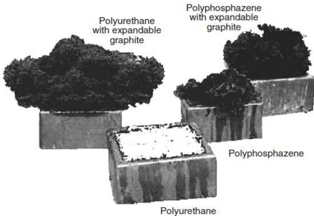
**Figure 13 Images of residue following cone calorimetry (Lyon)**
