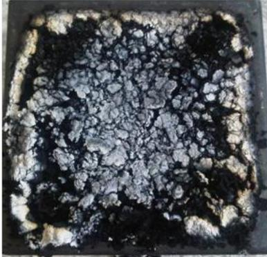
A100 shows evidence of a residue, but it is weak and friable
