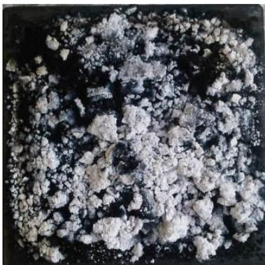
The use of ZHS coated onto MH in ZAH100 give a more powdery residue than M100
