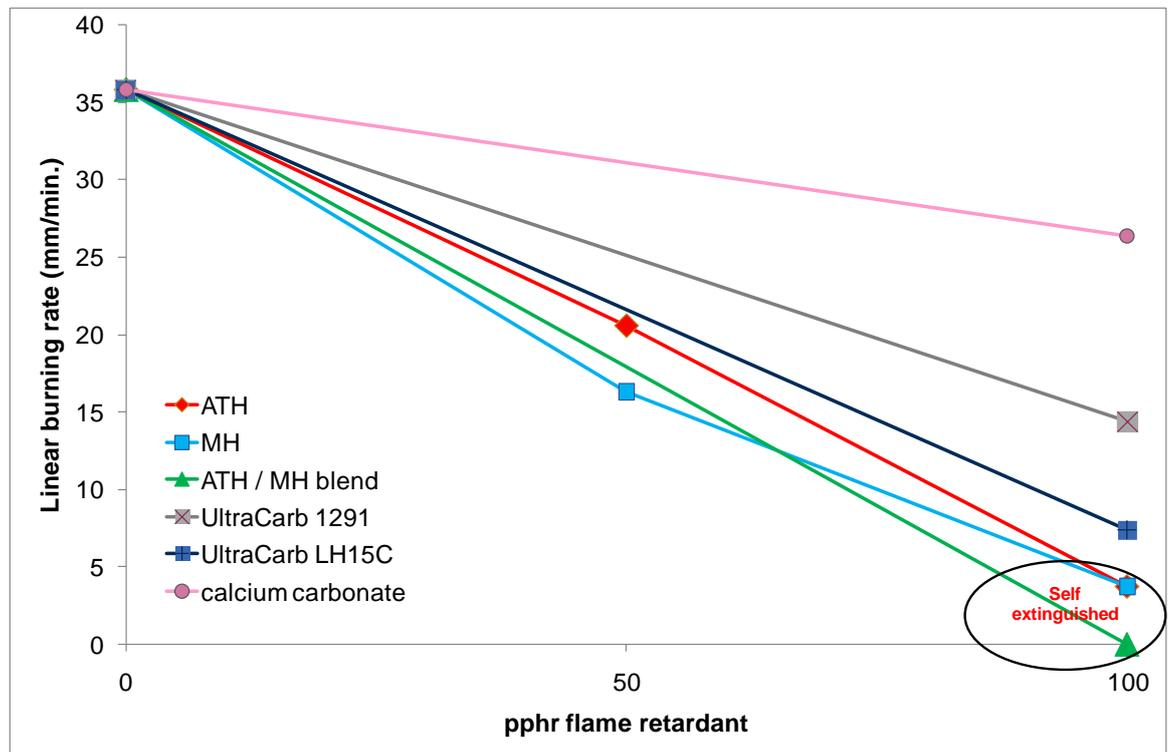
**Figure 70 Contribution to horizontal burning rate for hydrated filler formulations**
