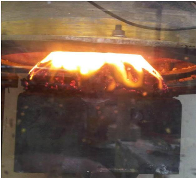
**Figure 102 Cone calorimeter sample showing the expansion of A95 EG5**
