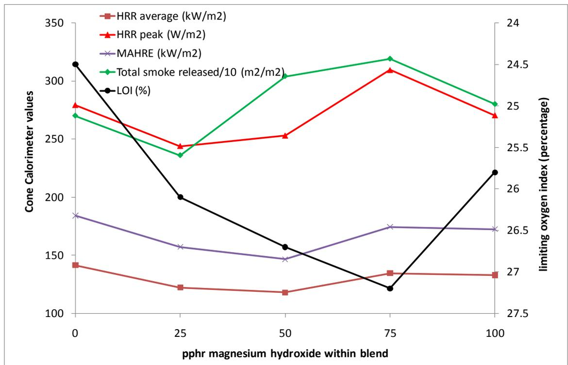
Figure 112 Comparison of burning values for ATH / MH blend formulations
