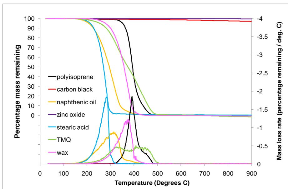
Figure 24 TGA and DTG curves for IR polymer and typical additives in nitrogen
