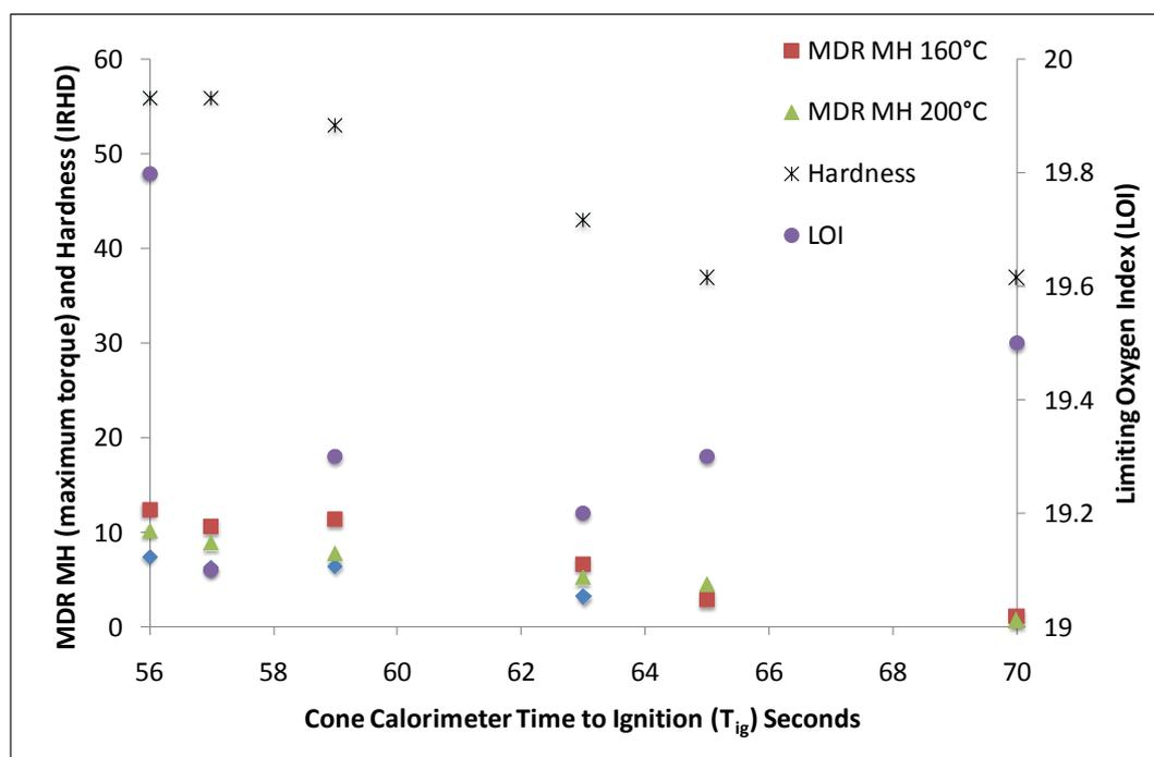
**Figure 39 Comparison of Time to Ignition to cross-linking data for cross-linking formulations**
