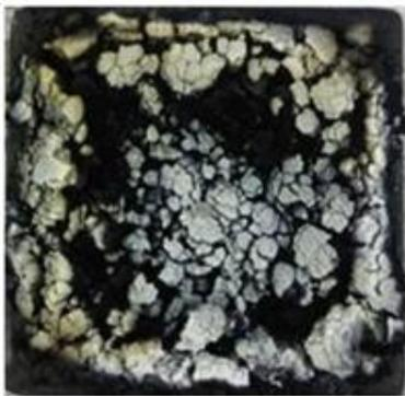
A50 M50 has a residue in appearance in-between A100 and M100, with some regions of well clumped residue, but patchy and inconsistent across the sample.
