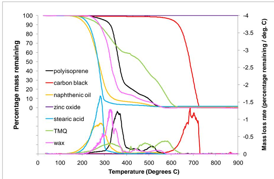
Figure 25 TGA and DTG curves for IR polymer and typical additives in air
