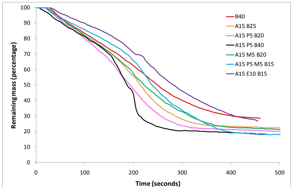
**Figure 56 Residual mass from cone calorimeter for APP formulations**
