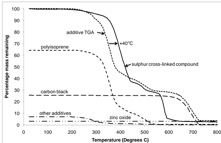
**Figure 36 TGA curves for compound SV - actual and additive in air**
