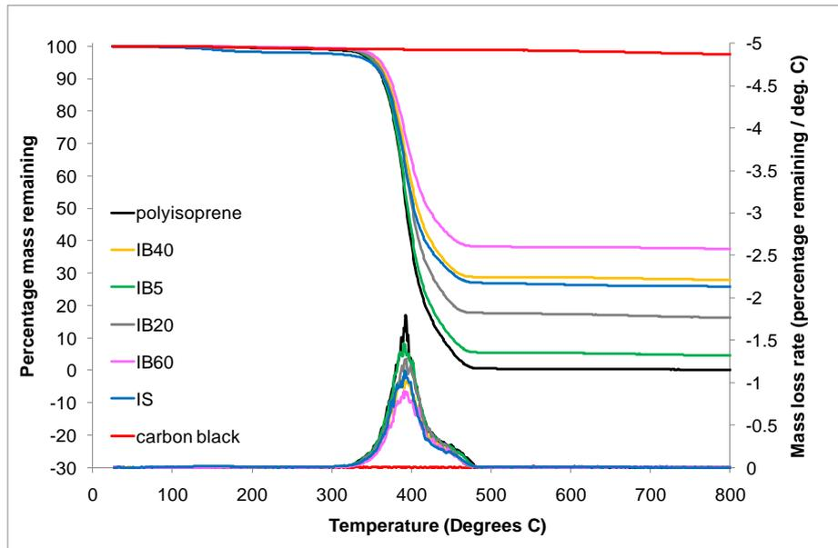
Figure 28 TGA and DTG curves for the variation of filler level and type in nitrogen
