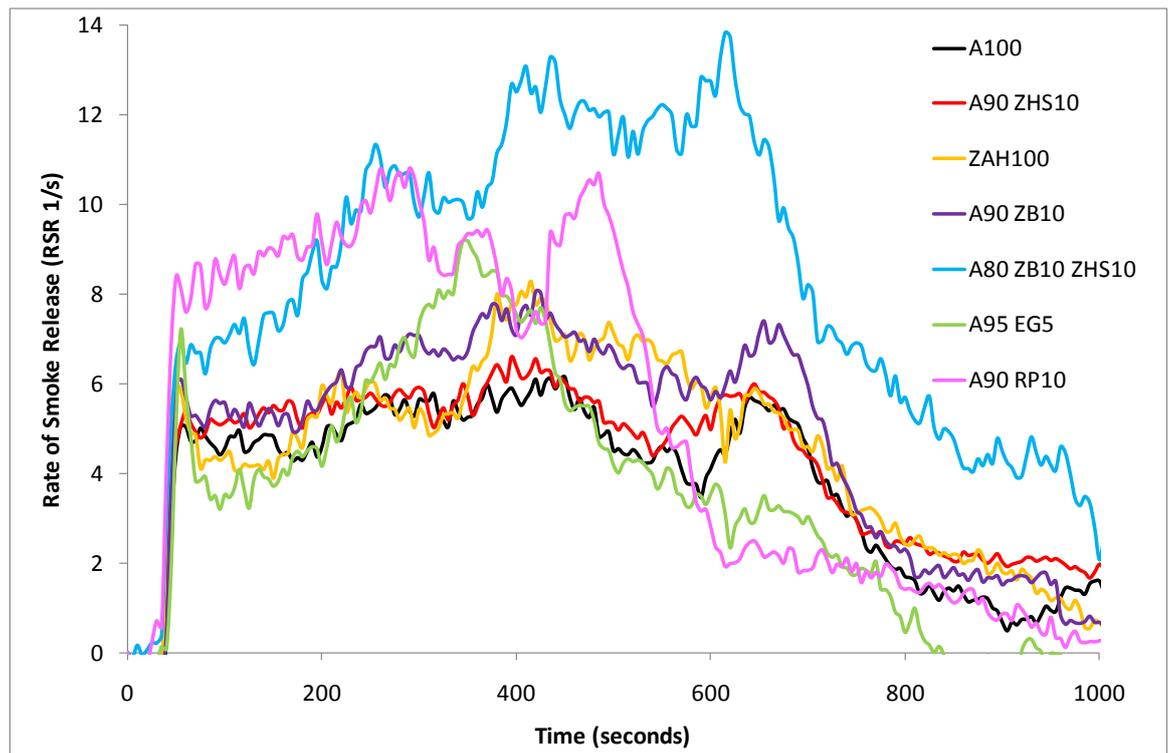
**Figure 90 Mean rate of smoke release from cone for ATH / synergist formulations**
