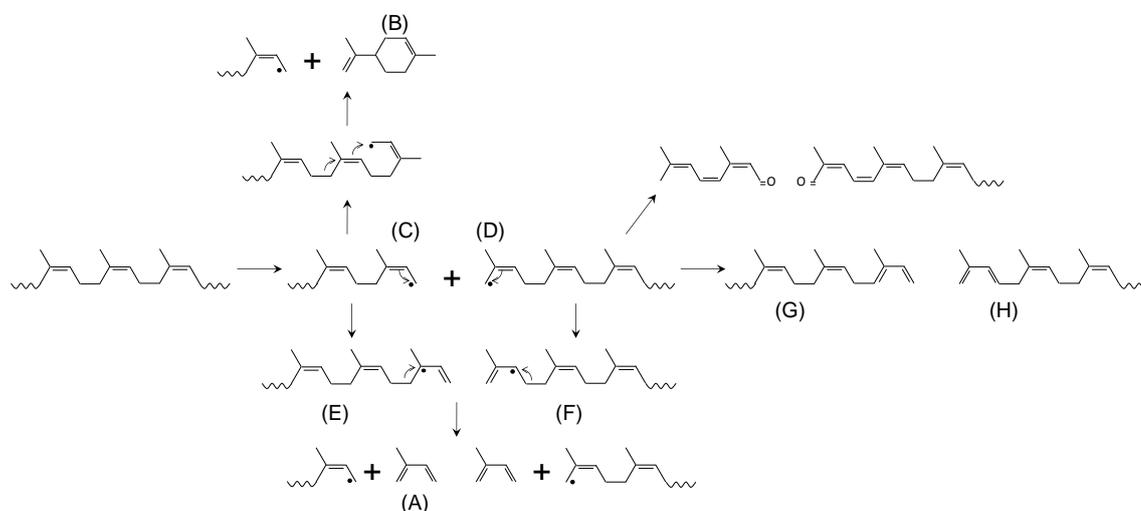
**Figure 7 Decomposition scheme for polyisoprene (Cataldo)**
