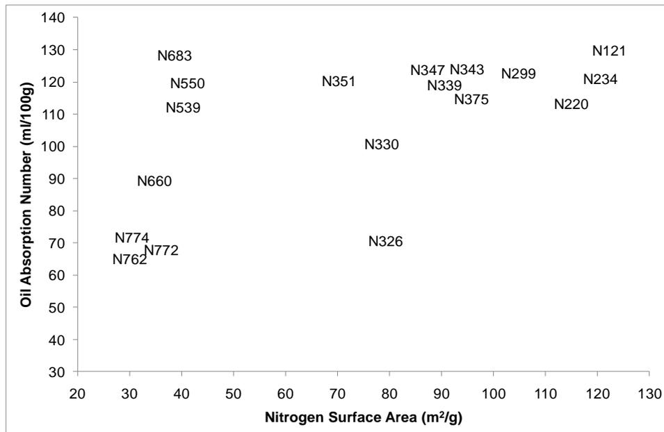
**Figure 4 ASTM D1765 classifications for carbon black in rubber**
