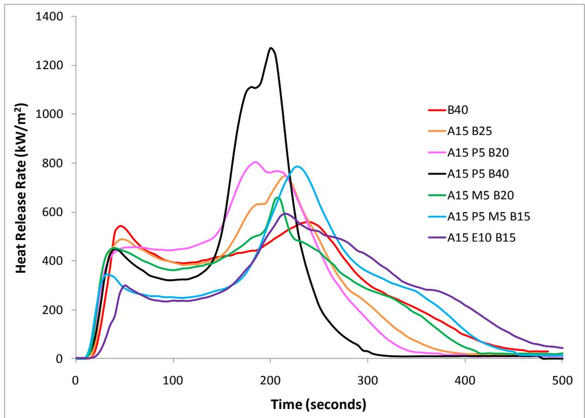
**Figure 55 Heat release rate from cone calorimeter for APP formulations**
