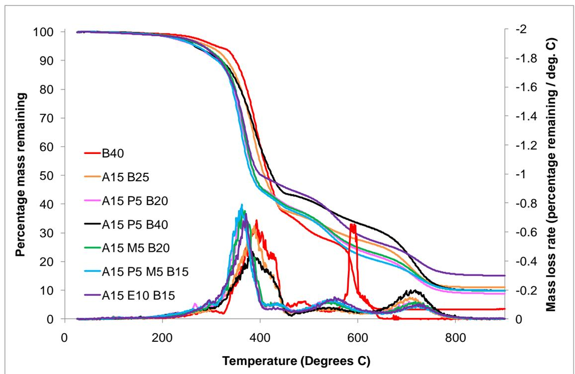
Figure 54 TGA and DTG curves for APP formulations in air
