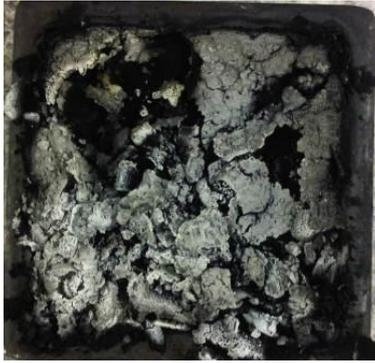
The use of red phosphorus led to a bound residue structure within the remaining residue
