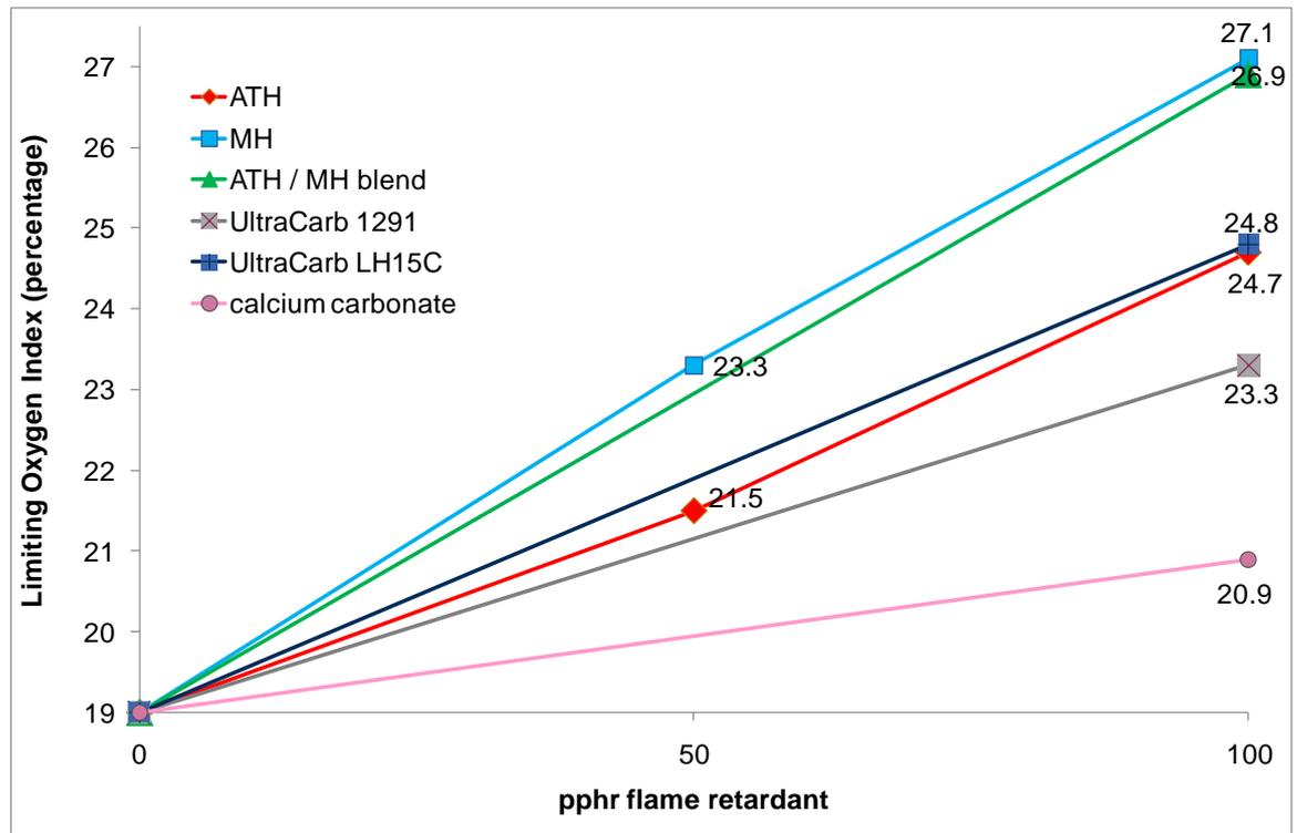
**Figure 69 Contribution to LOI for hydrated filler formulations**
