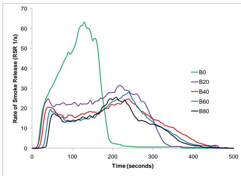
**Figure 51 Mean rate of smoke release for carbon black formulations**
