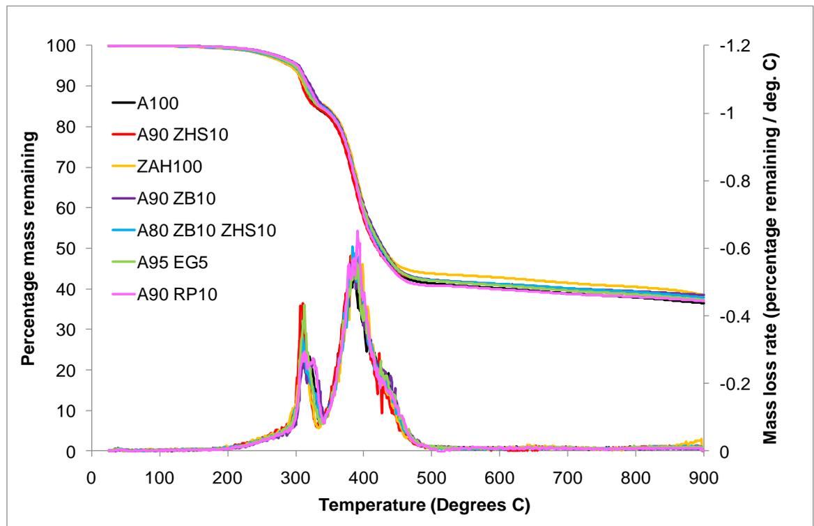
**Figure 82 TGA and DTG curves for ATH / synergist formulations in nitrogen**
