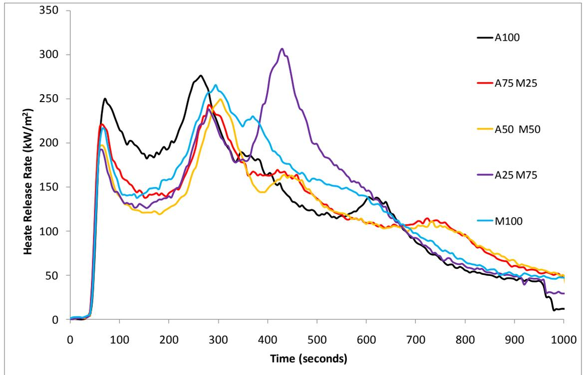
**Figure 105 Heat release rate from cone for ATH / MH blend formulations**
