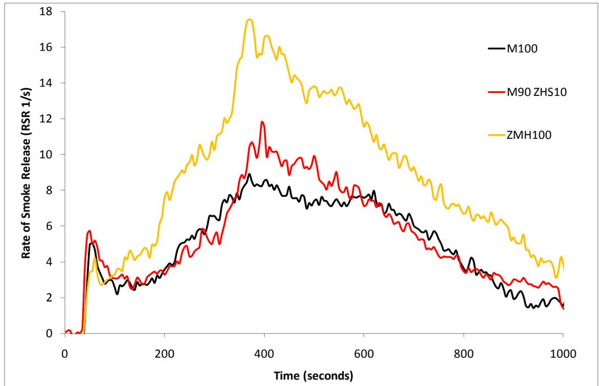
**Figure 91 Mean rate of smoke release from cone for MH / ZHS formulations**
