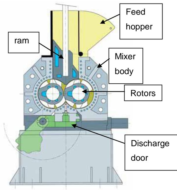
Figure 17 Cross-sectional schematic view of a typical internal mixer
