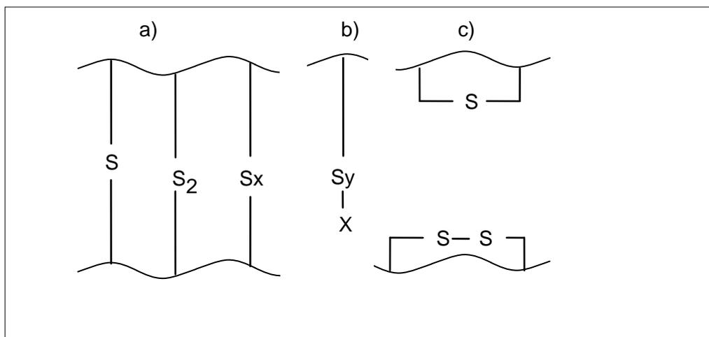
**Figure 5 Schematic view of sulphur cross-links across polymer chains**
