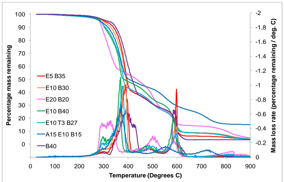
Figure 59 TGA and DTG curves for expandable graphite formulations in air
