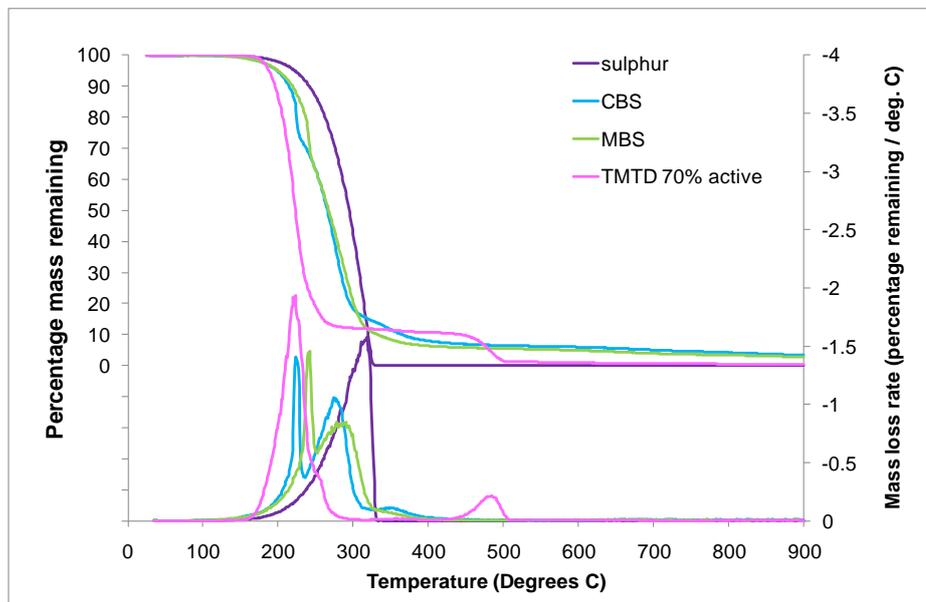
Figure 26 TGA and DTG curves for cross-linking additives in nitrogen
