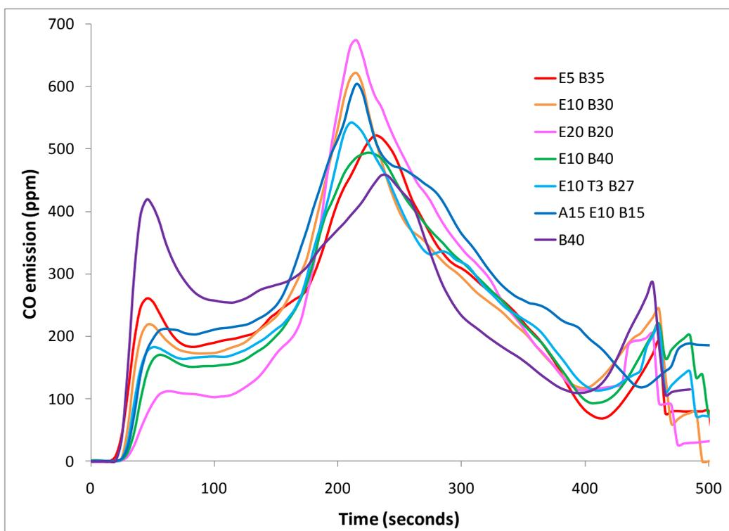
Figure 63 CO emissions from cone for expandable graphite formulations
