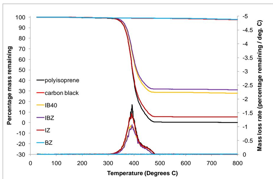
**Figure 31 TGA and DTG curves comparing the influence of zinc oxide in nitrogen**
