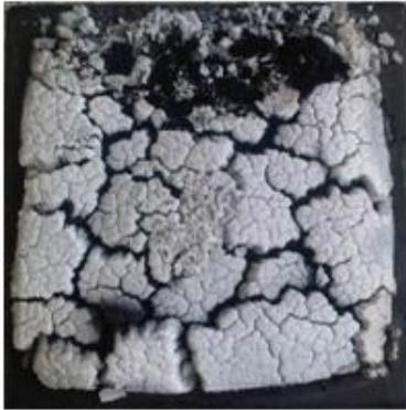
UC12 100 leaves a residue stronger and more intact than ATH or MH, but with more cracks than C100.
