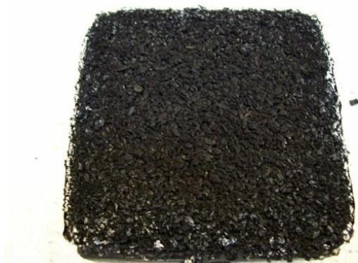
**Figure 40 Image of cone residue from formulation N**
