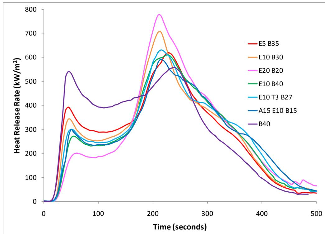
**Figure 60 Heat release rate from cone for expandable graphite formulations**
