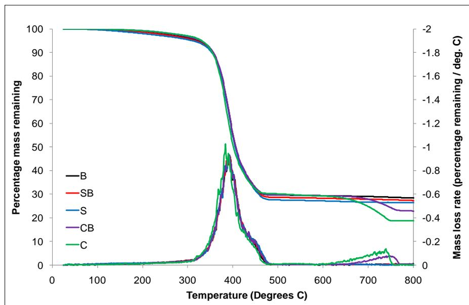
Figure 41 TGA and DTG curves for varied filler formulations in nitrogen
