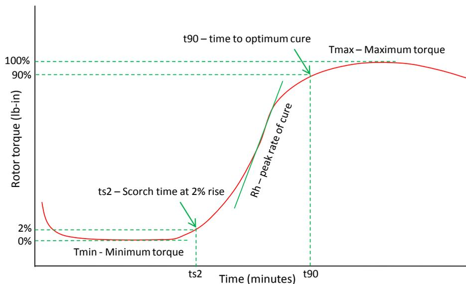
**Figure 18 Simplified MDR plot showing key data points**
