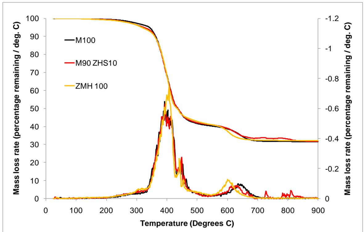
Figure 85 TGA and DTG curves for MH / ZHS formulations in air
