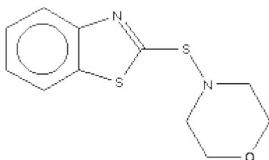
**Figure 15 Chemical structure of MBS accelerator**
