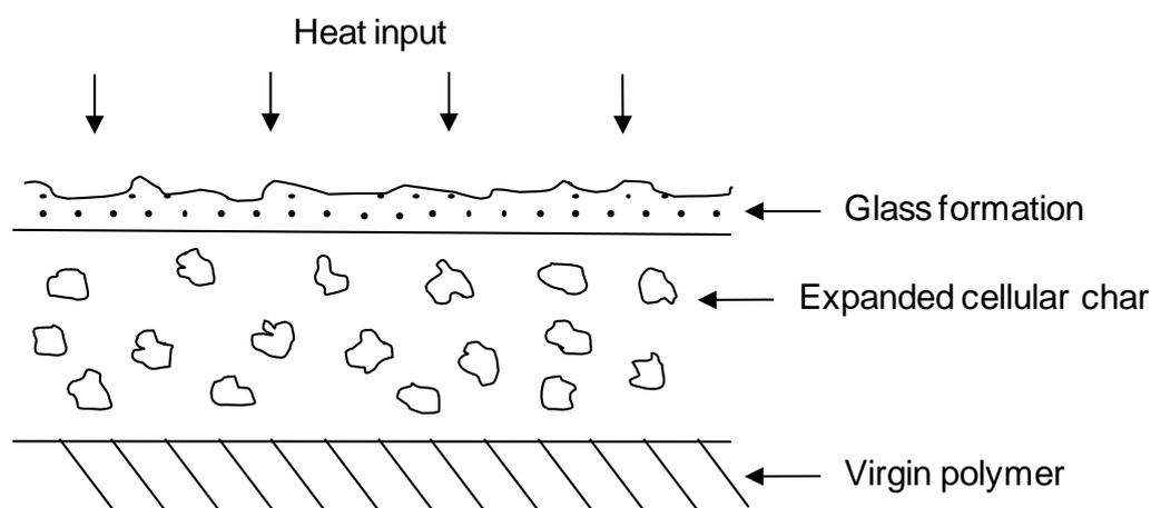
**Figure 12 Scheme for intumescent char layer development for APB**
