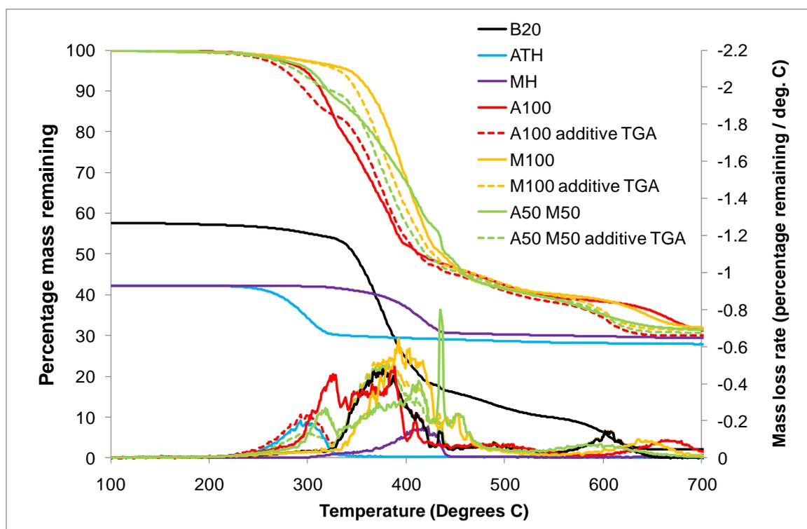
**Figure 66 TGA and DTG curves actual and additive for ATH / MH formulations in air**
