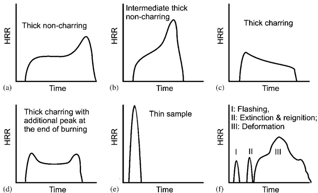
**Figure 23 Typical HRR curves for different characteristic burning behaviours**
