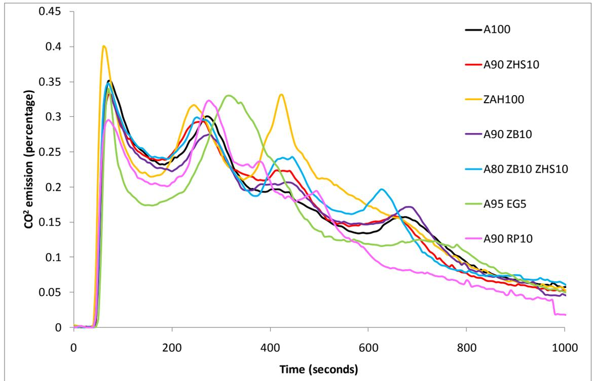
**Figure 88 CO<sub>2</sub> mean % emission from cone for ATH / synergist formulations**
