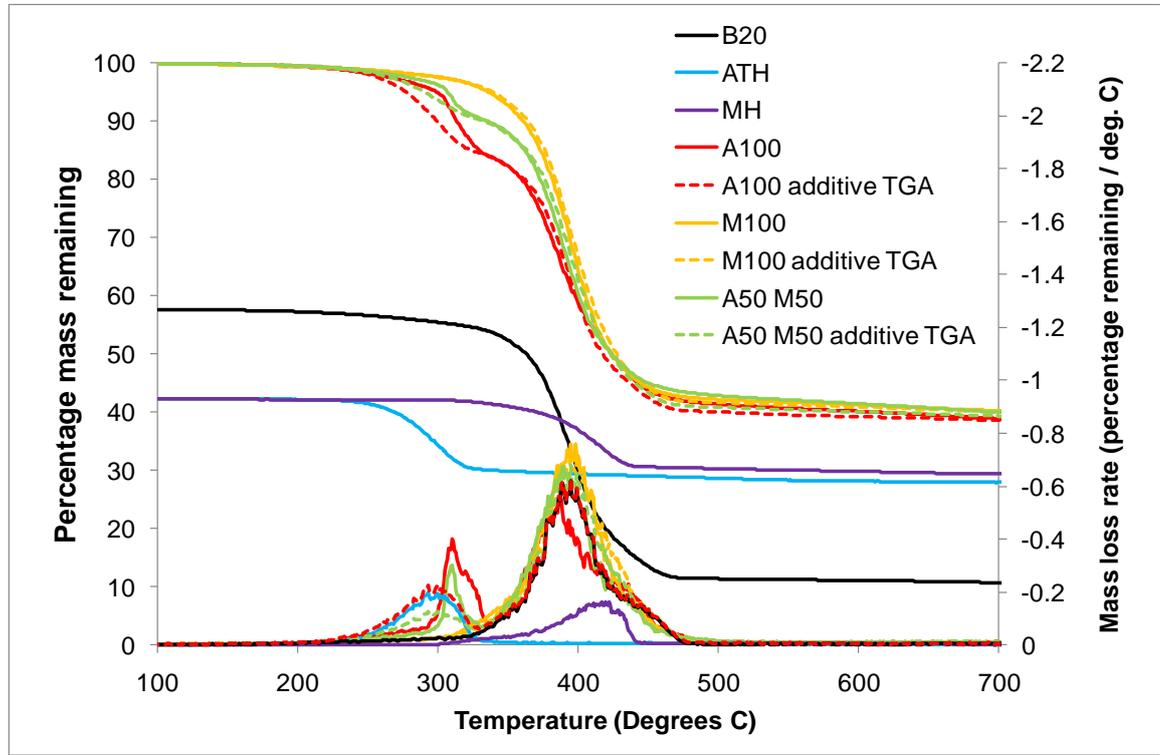
**Figure 65 TGA and DTG curves actual and additive for ATH / MH formulations in nitrogen**
