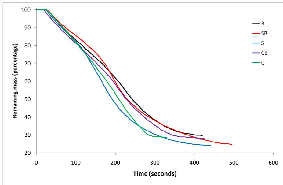
**Figure 44 Residual mass from cone for varied filler formulations**
