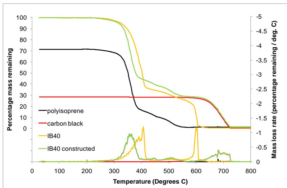
**Figure 30 Constructed and actual TGA and DTG curves for IB40 in air**
