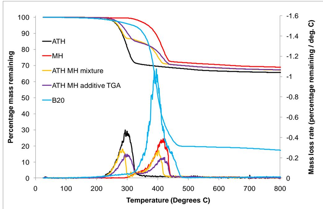
**Figure 113 TGA and DTG curves actual and additive for ATH, MH and a mixture, in nitrogen**
