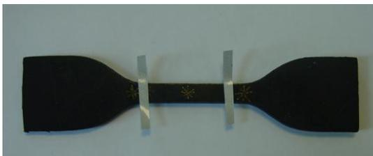
**Figure 19 Dumb-bell test piece with reflective tape indicating extension section**
