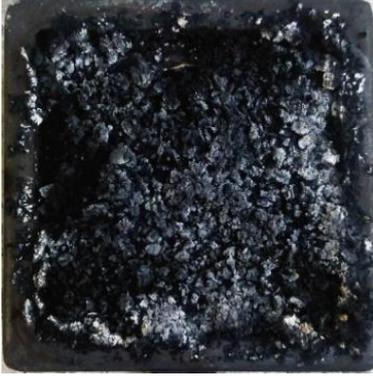
The residue from A50 was extremely friable with small residual particles and carbon black and ATH residue.
