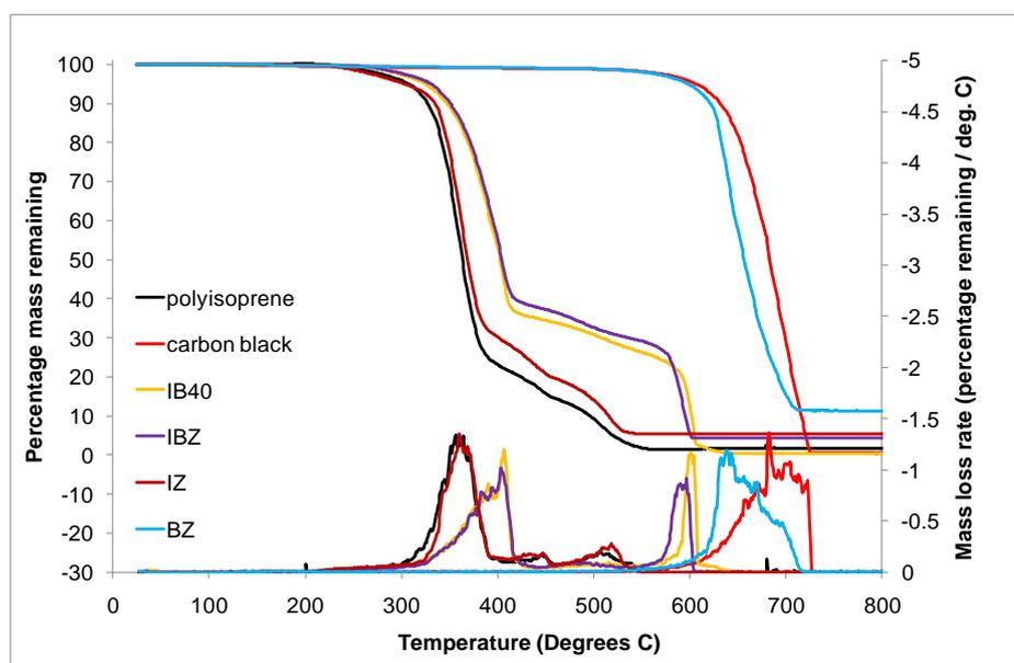
**Figure 32 TGA and DTG curves comparing the influence of zinc oxide in air**
