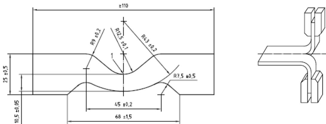
**Figure 20 Crescent and Trouser tear test piece shapes**
