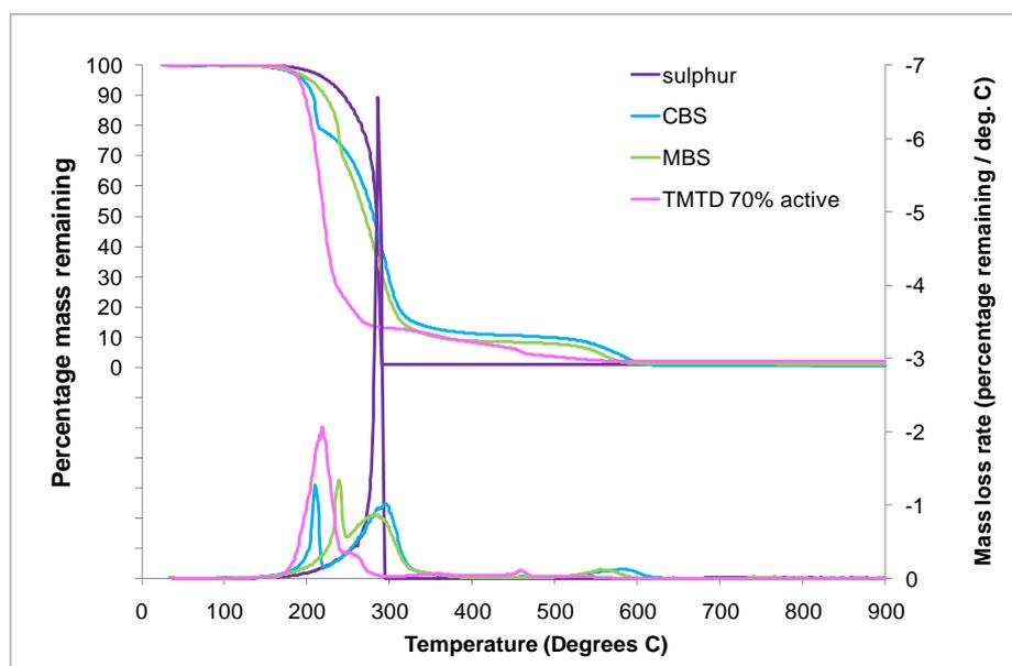
**Figure 27 TGA and DTG curves for cross-linking additives in air**
