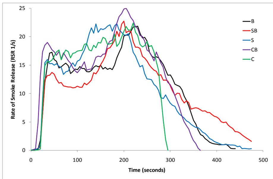
**Figure 45 Mean rate of smoke release from cone for varied filler formulations**
