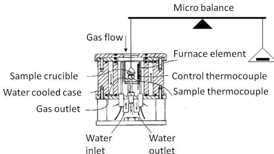
**Figure 6 Cut-through view of a Stanton Redcroft TGA**
