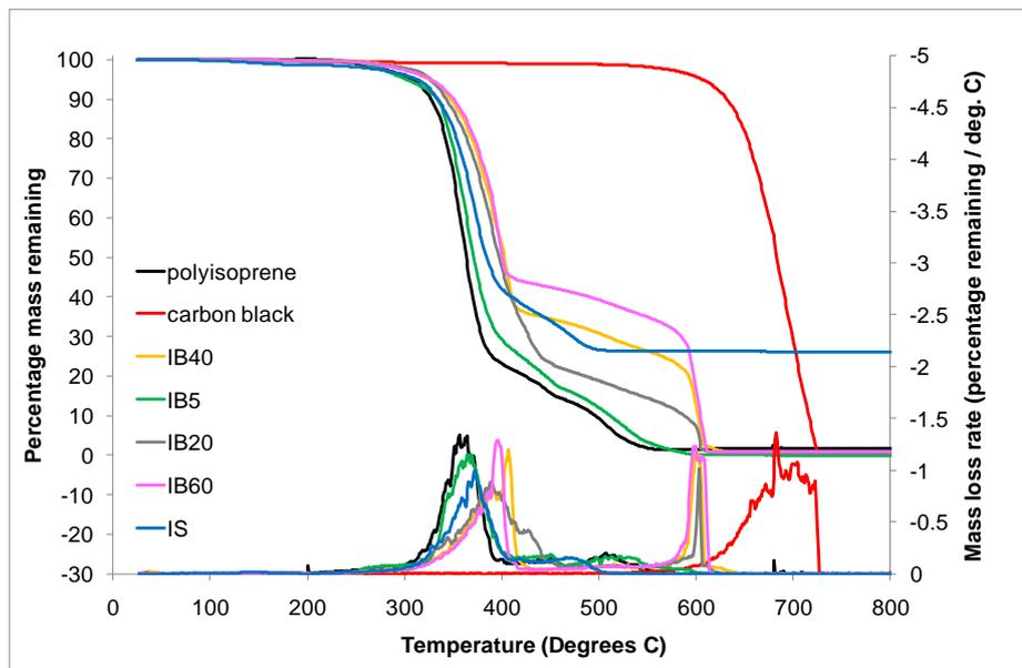
Figure 29 TGA and DTG curves for the variation of filler level and type in air
