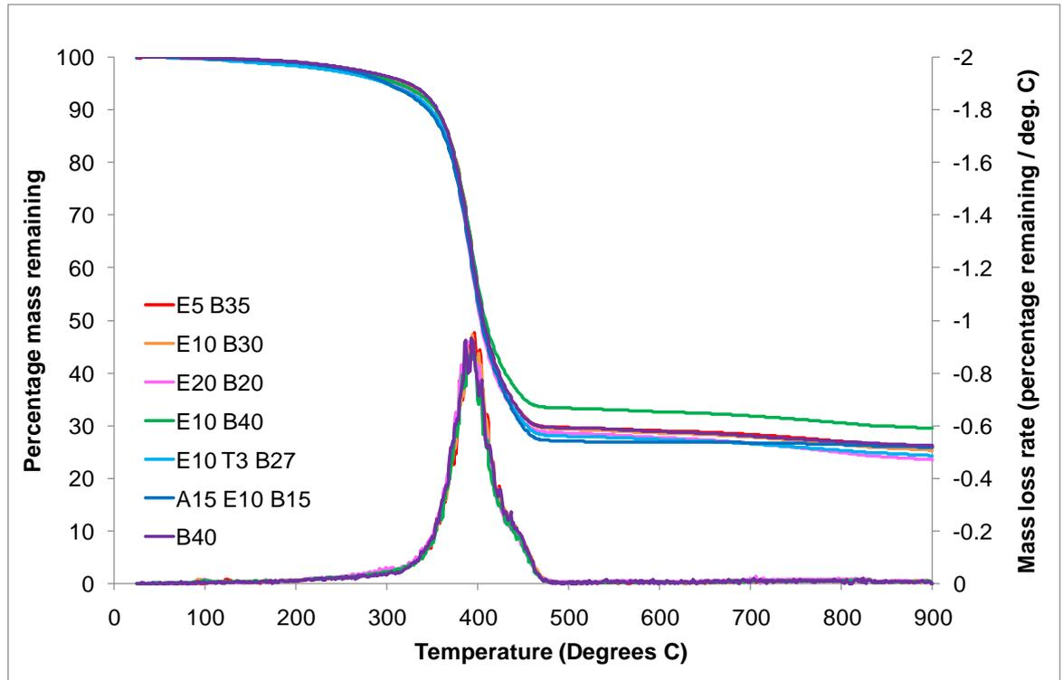
Figure 58 TGA and DTG curves for expandable graphite formulations in nitrogen
