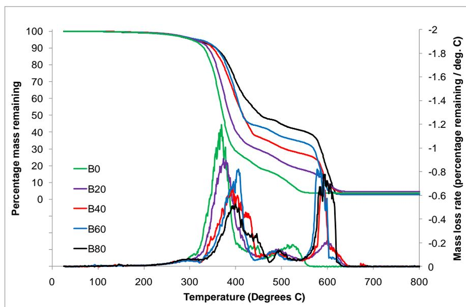
**Figure 47 TGA and DTG curves for carbon black formulations in air**
