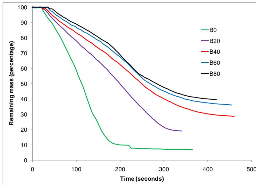
**Figure 50 Residual mass from cone calorimeter for carbon black formulations**
