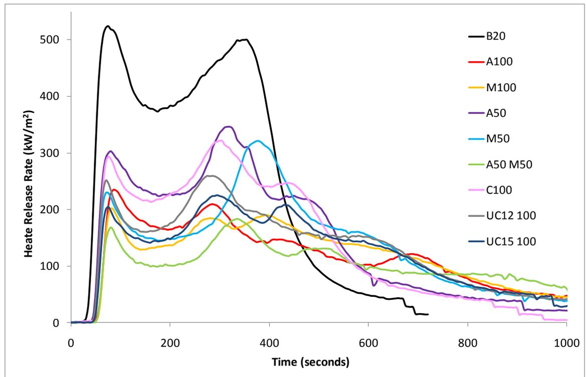
**Figure 71 Heat release rate from cone for hydrated filler formulations**
