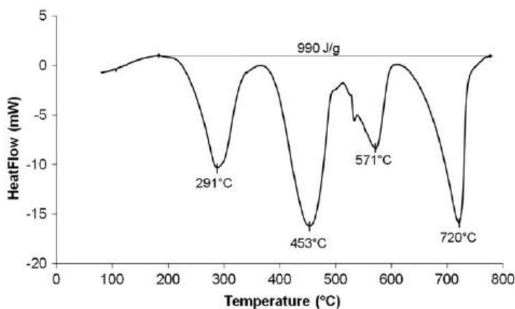
Figure 11 DSC profile of a mix of huntite and hydromagnesite
