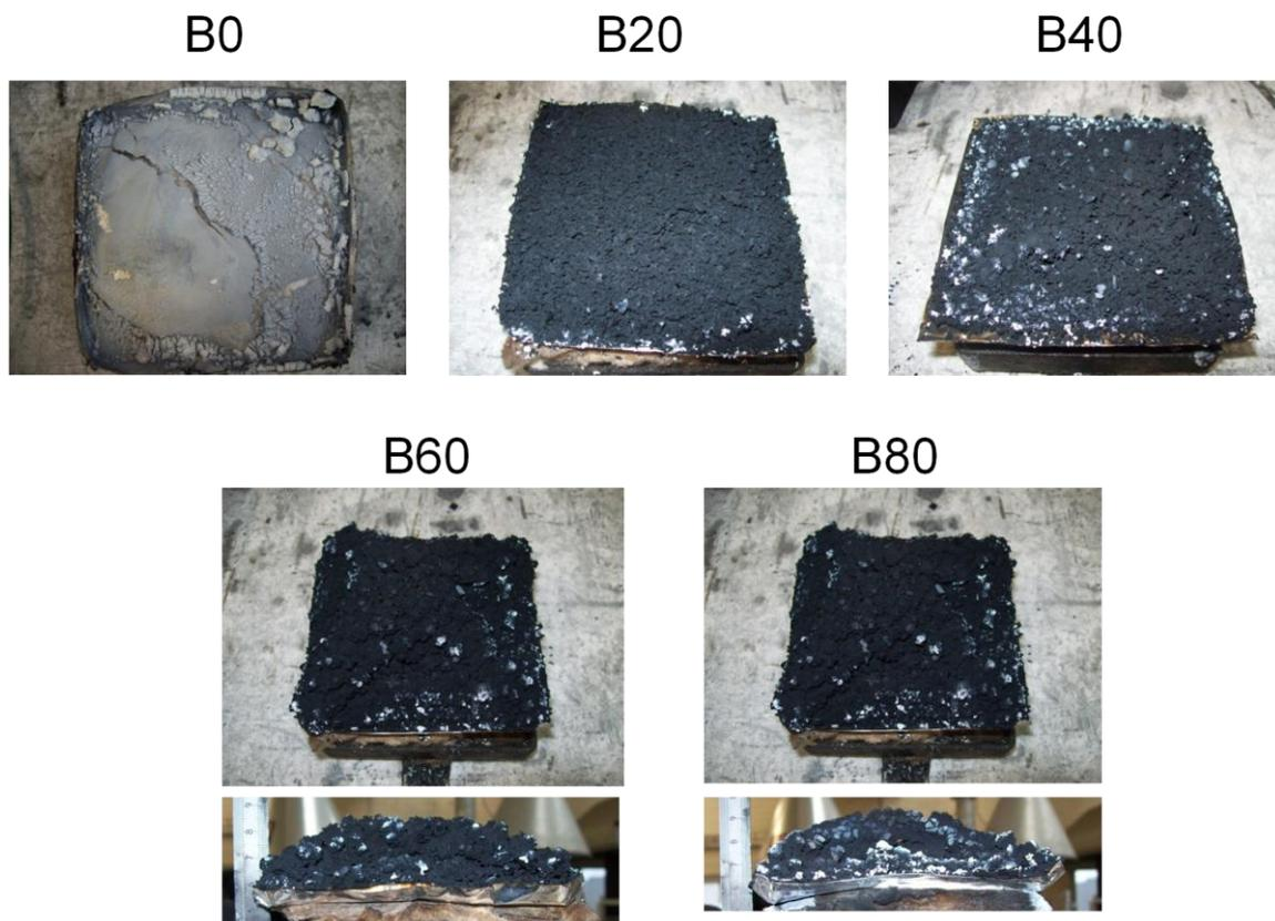
**Figure 52 Images of typical cone residues for carbon black formulations**
