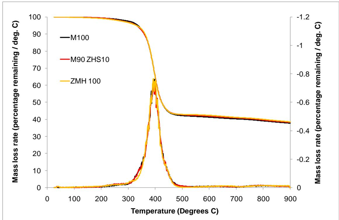
Figure 84 TGA and DTG curves for MH / ZHS formulations in nitrogen
