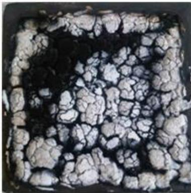
M100 has a similar structure to A25 M75, with smooth sections separated by deep cracks in the residue
