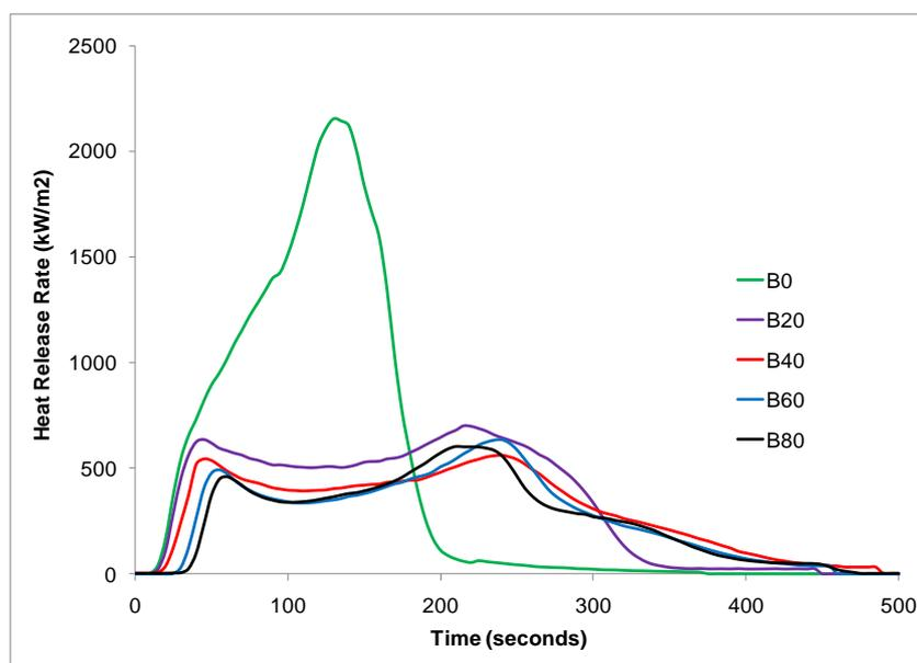
**Figure 49 Heat release rate from cone calorimeter for carbon black formulations**
