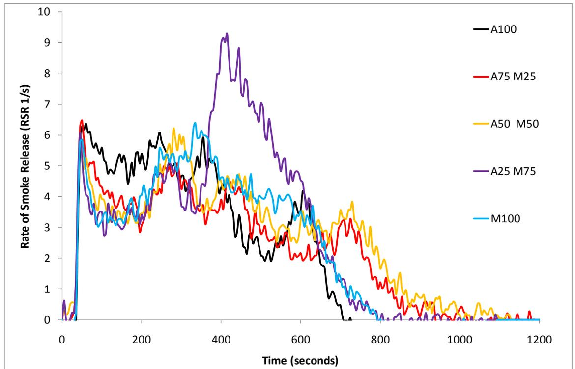
**Figure 106 Mean rate of smoke release from cone for ATH / MH blend formulations**
