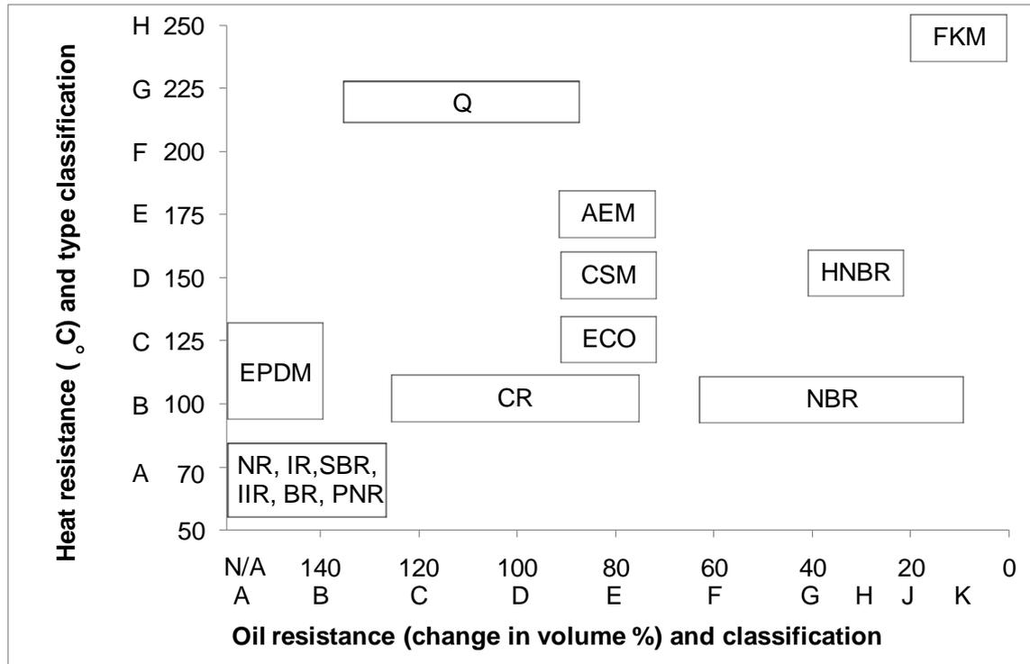
**Figure 3 Polymer types within ASTM D2000 classifications**
