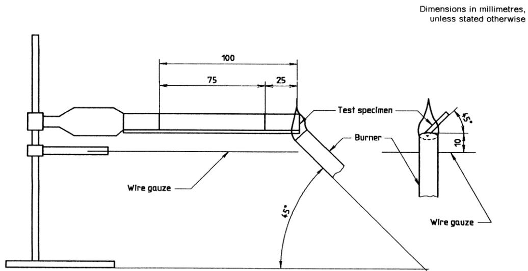
**Figure 21 Test sample configuration ISO 1210 method A**
