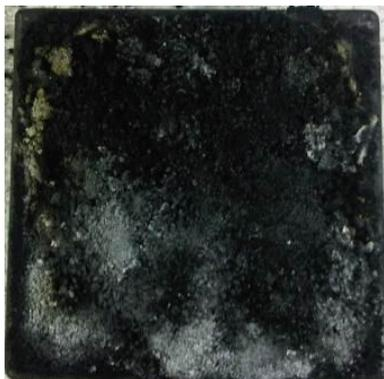
A95 EG5 left an expanded and powdery residue around 25mm in height
