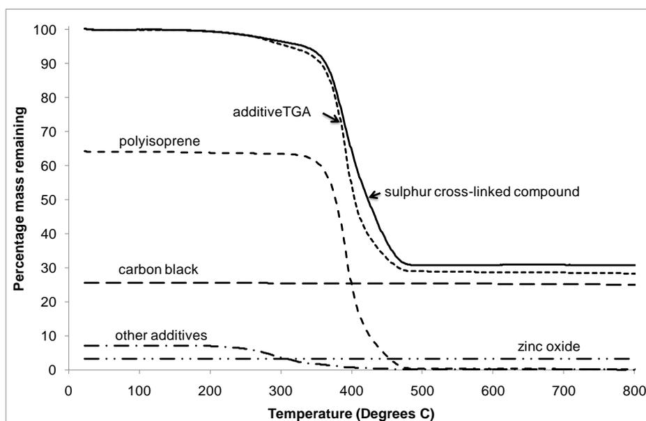
Figure 35 TGA curves for compound SV - actual and additive in nitrogen
