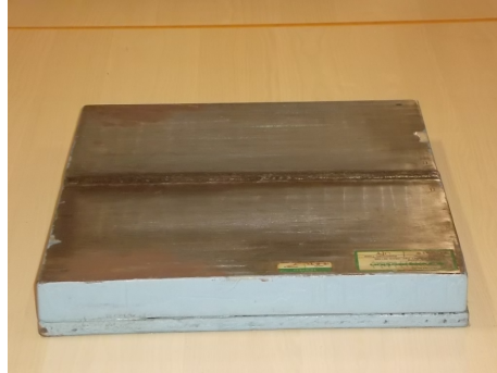
b) Welded Test Block
