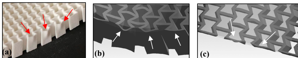
Fig. 7. A qualitative comparison of the 3D printed re-entrant core failure shown by the plastic deformation of some of the cells between (a) the experimental and (b,c) FEA results.
