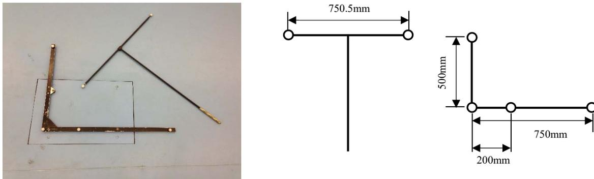
**Figure 2.4.** T shaped wand and L-frame (Left) and dimensions of the T shaped wand and L-frame (Right)
