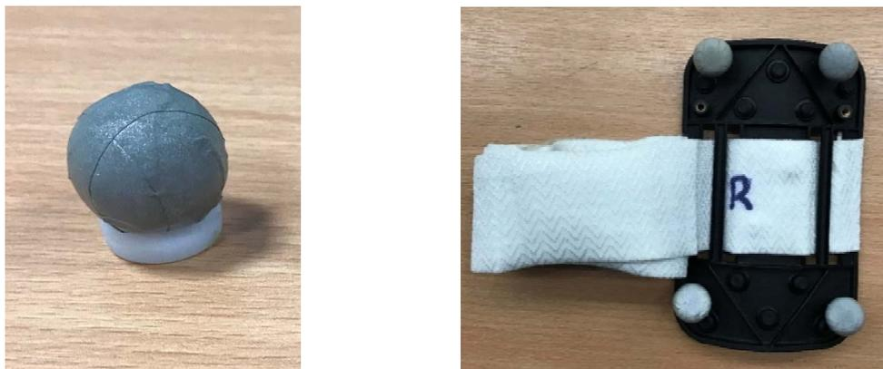
**Figure 2.6.** Anatomical marker (left picture) and tracking cluster (right picture) which were attached to the body of the participants.
