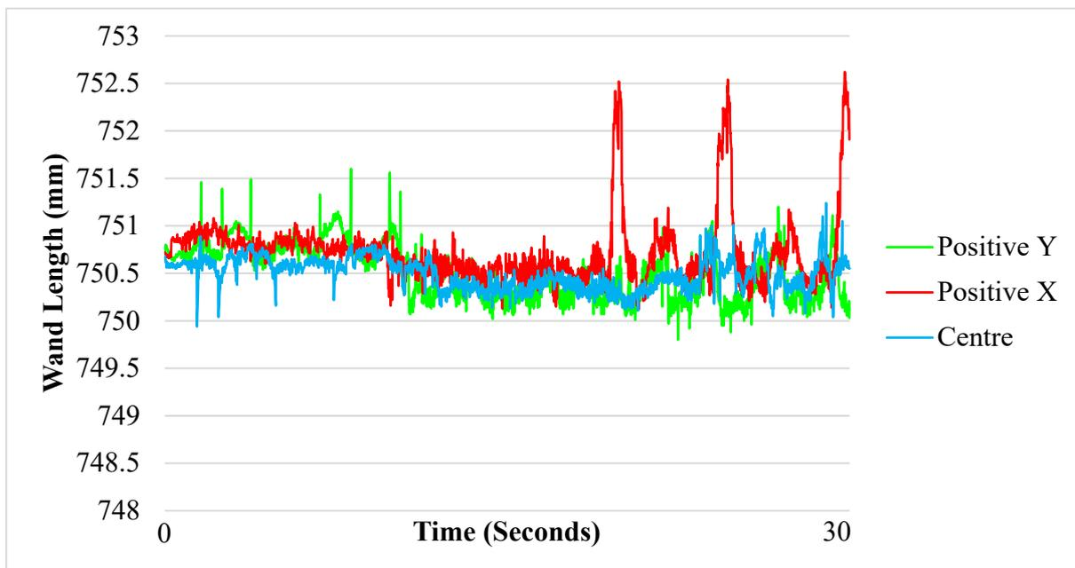
**Figure 2.5.** Fluctuation of the distance between the two markers attached to the T shaped wand for the three differing positions.
