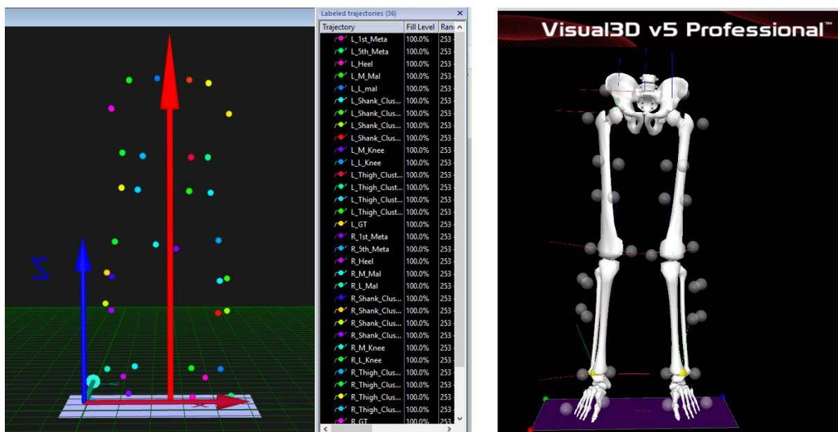
**Figure 2.7.** Anatomical and tracking markers attached to a participant's lower body segments shown in the QTM software (left picture) and once built into a skeletal model in the Visual 3D software (right picture).
