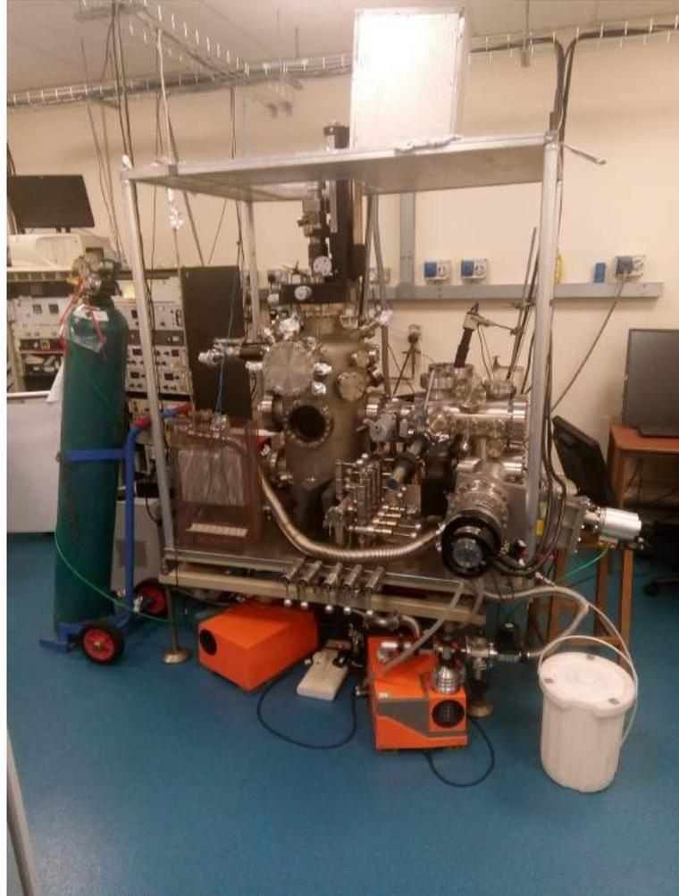
Figure 4.1: UHV chamber with a partially assembled bake out cage around it, situated in the nanophysics lab at UCLan.
