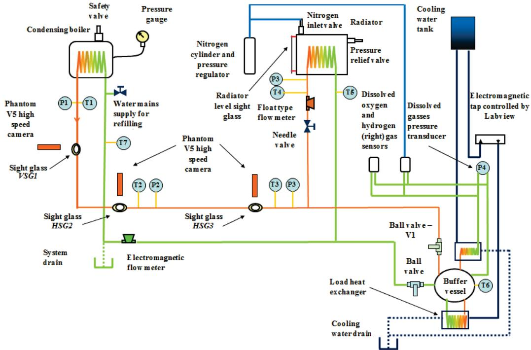
**Figure 2:** Schematic diagram of experimental set up
