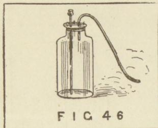
the bottle place some fragments of marble. Then pour down the funnel some dilute hydrochloric acid. Marble is calcium carbonate, and as soon as the acid comes into contact with this it forms calcium chloride and liberates carbonic acid gas. This will at once be observed by the copious effervescence that is set up, and the current of gas that is passing down the delivery tube. In the absence of marble ordinary chalk may be used, with dilute sulphuric acid. The manufactured
