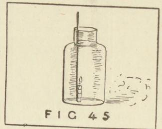
board. The candle will quickly expire. Remove the candle and shake up the lime water in the bottle; it will at once become turbid owing to
