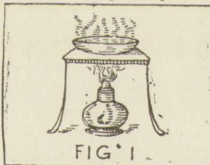
in Fig. 1. On gently heating the liquid the water is driven off in the form of steam and the salt remains behind in exactly the same quantity as was originally taken. No
