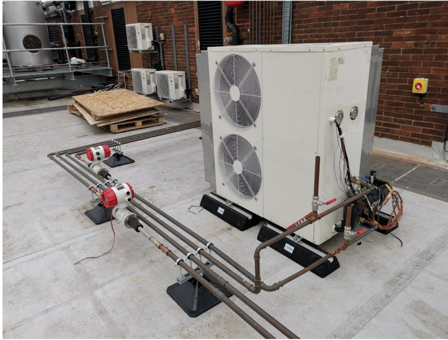
Fig. 14. Prototype of the novel DSVIHP.
