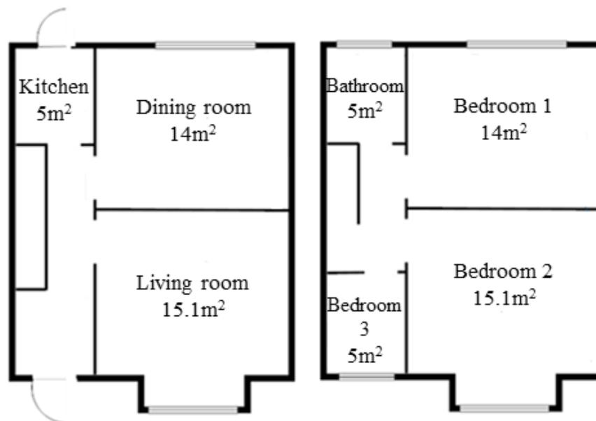
Figure 4.1 Floor plans of the semi-detached A&P house (left: ground floor, right: first floor) and floor area (m<sup>2</sup>) of each room (re-created from (Allen and Pinney, 1990))
