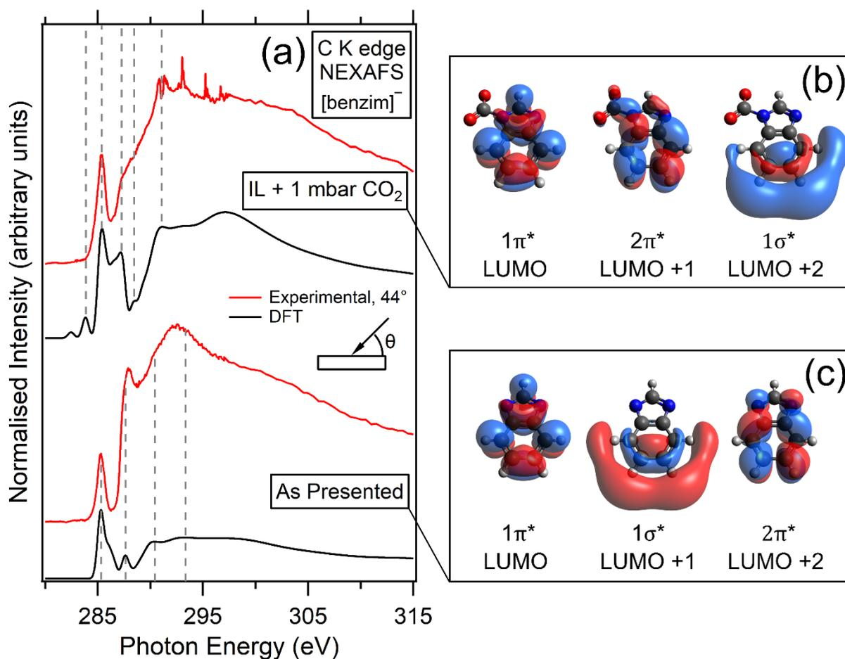
**Figure 4.** (a) Experimental and simulated (DFT) C K edge NEXAFS of  $[P_{66614}][benzim]^-$  as presented and when exposed to 1 mbar of  $CO_2$ . The grey dashed lines highlight features of the DFT spectra for comparison with the experimental spectra. The experimental spectra were taken  $44^\circ$  from the IL surface. (b) Lowest unoccupied molecular orbitals (LUMOs) of  $[benzim]^- + CO_2$  arranged in order of increasing energy (left to right). LUMO, LUMO+1 and LUMO+2 are assigned
