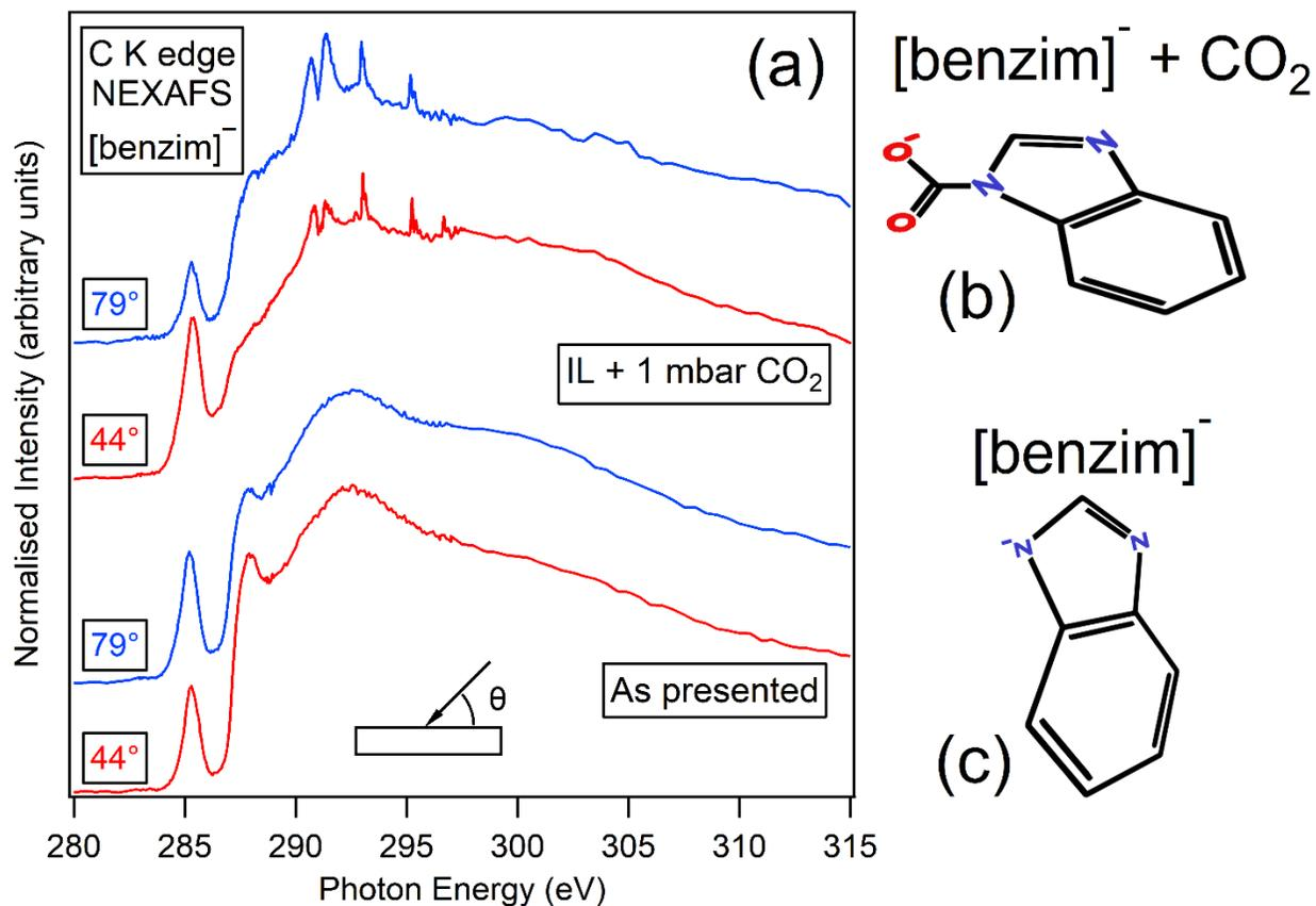
Figure 3. (a) C K edge NEXAFS spectra of [P<sub>66614</sub>][benzim] as presented and when exposed to 1 mbar of CO<sub>2</sub>, for the X-ray beam incident at angles ( $\theta$ ) of 44° and 79° from the IL surface. Schematic pictures indicating the orientation of the anion (b) while exposed to CO<sub>2</sub> (benzim ring 54° from surface normal) and (c) as presented (benzim ring 27° from surface normal).
