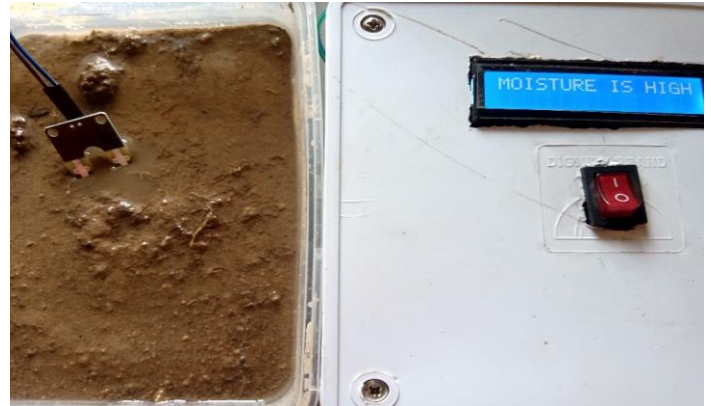
Fig. 7 Response of the soil sensor when the water content is large
