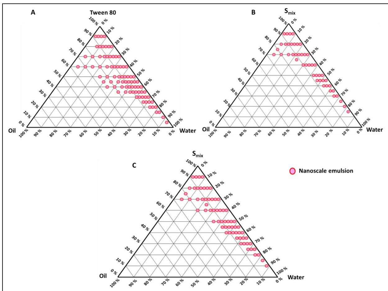
**Fig. 1: Pseudoternary phase diagrams. (A) Tween 80 used as surfactant; (B) S<sub>mix</sub> is Tween 80: PEG-300 [1:1] and (C) S<sub>mix</sub> is Tween 80: PEG-300 [2:1]**
