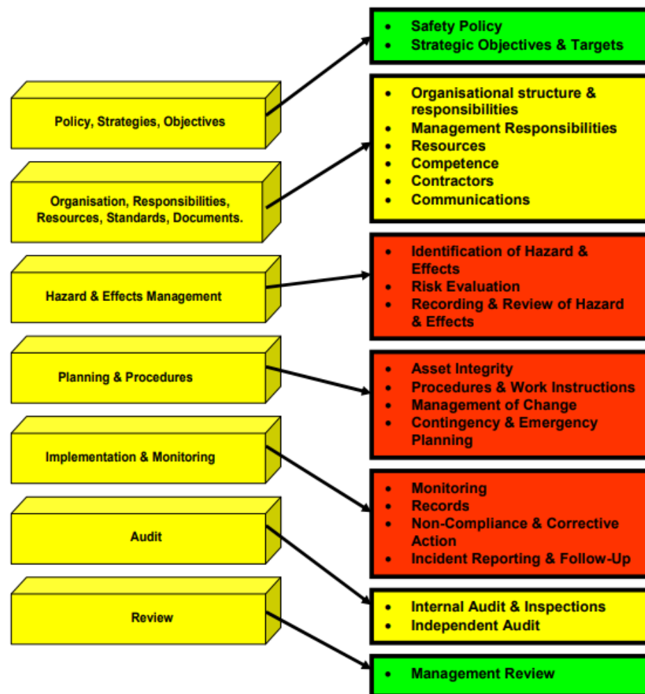
Figure 12. Elements of a management system that is capable of managing aging plant issues (This image is re-used/reproduced with permission of the Health and Safety Executive under the terms of the Open Government License, Courtesy: HSE, UK. Source: [224]).
