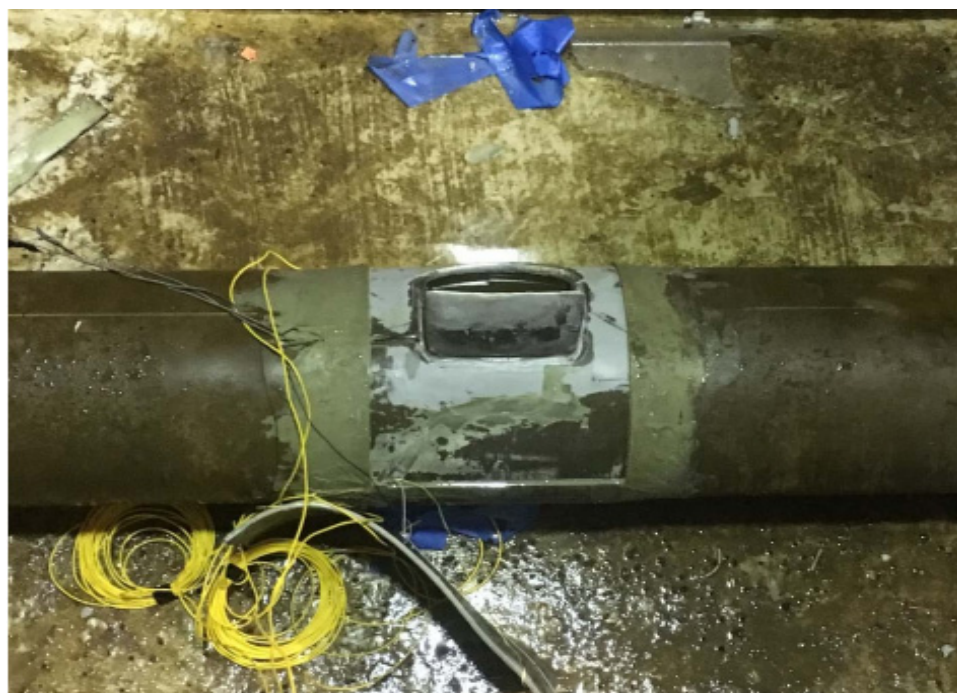
Figure 25. Typical composite pipe that is repaired with CompositSleeve™ sample after pressure testing showing the attached optical fiber sensors (Reprinted/adapted with permission of Dr Chris Alexander. Copyright 2018 ASME & Chris Alexander. Source: Ref. [377]).
