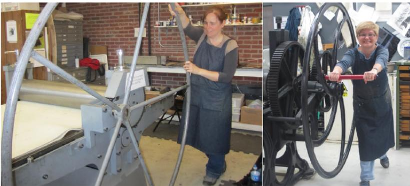
Above, Tracy Hill at Pyramid Atlantic. At right, Martha Oatway at UCLan studios. From Martha: "The press at PA is so new you can spin it (literally) with one finger. The press at UCLan is from the early 20th century and geared much differently. Using the press is hard work; someone told me that from one end of the bed to the other is upwards of 75 turns of the wheel. Just look at the gearing!"
