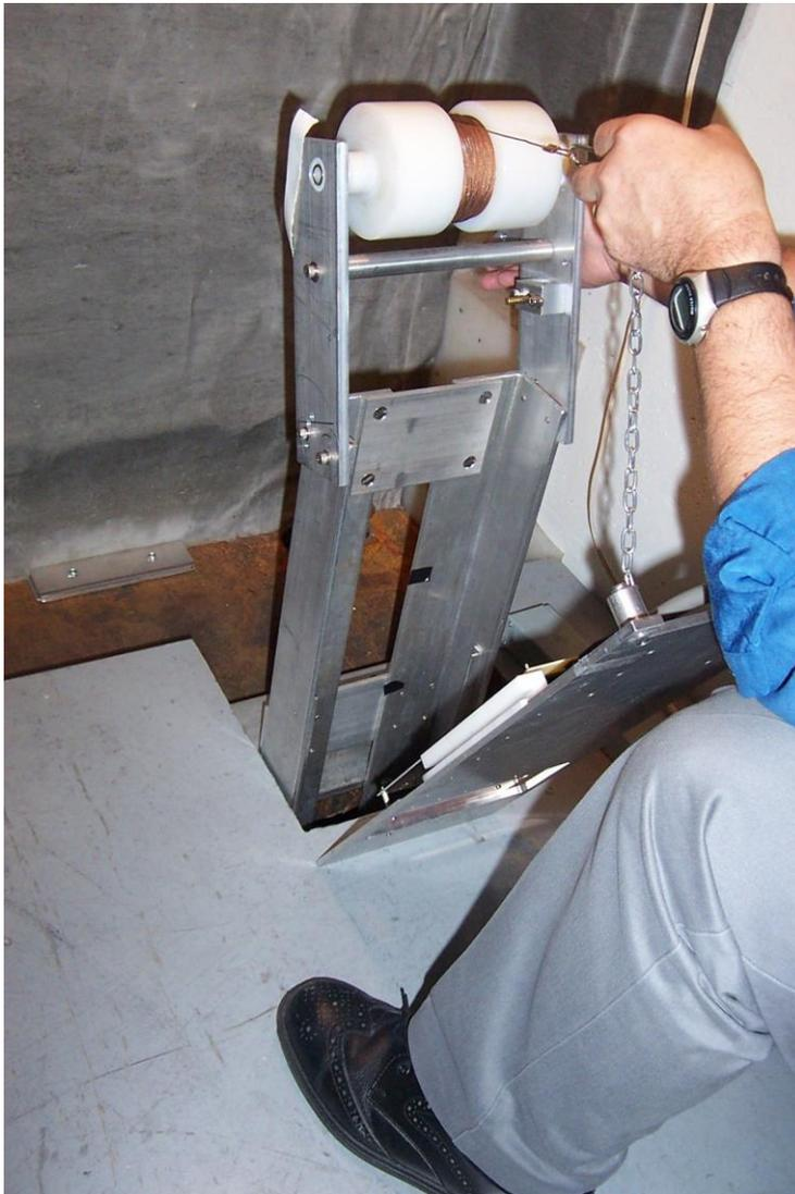
**Figure 4.17 TRIUMF NIF Slot and an Example Test Board on Slider Plate**
