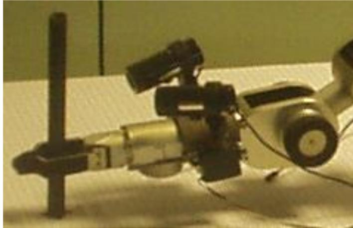
Plate 3 Location of visual servoing system on Katana Robot arm
