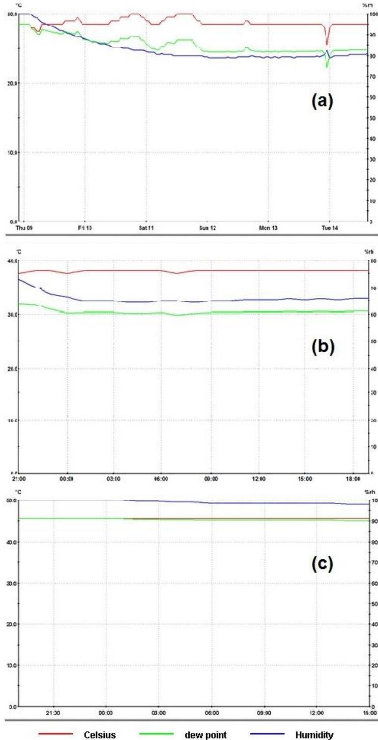
**Figure 2.7** Shown above is an example of data recorded during rabbit controlled incubation experiment using USB data logger, a) 27 °C, b) 37 °C and c) 47 °C.
