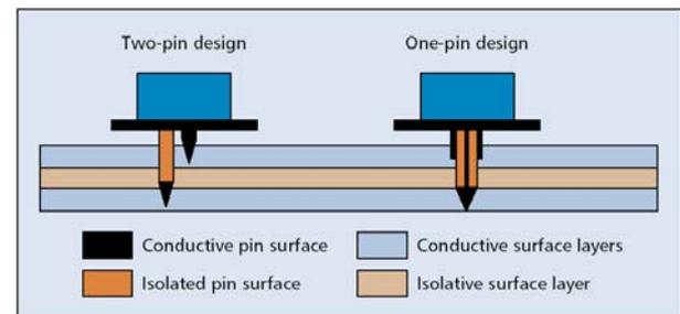
**Figure 1** Surface with Pushpin connectors, dual pin with a simple layered structure
