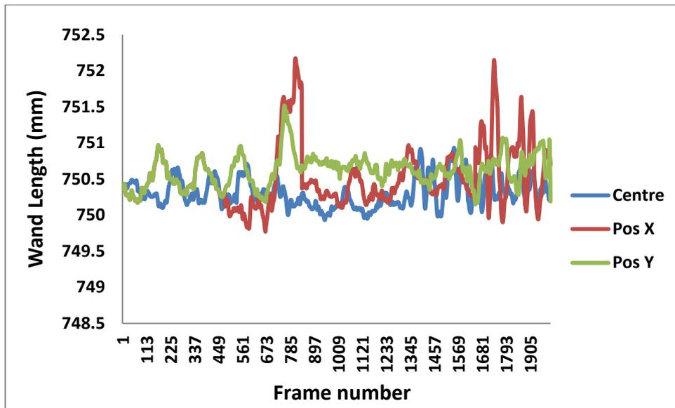
Figure 4.1: Measured wand length over 2000 frames at different areas of the calibration volume.
