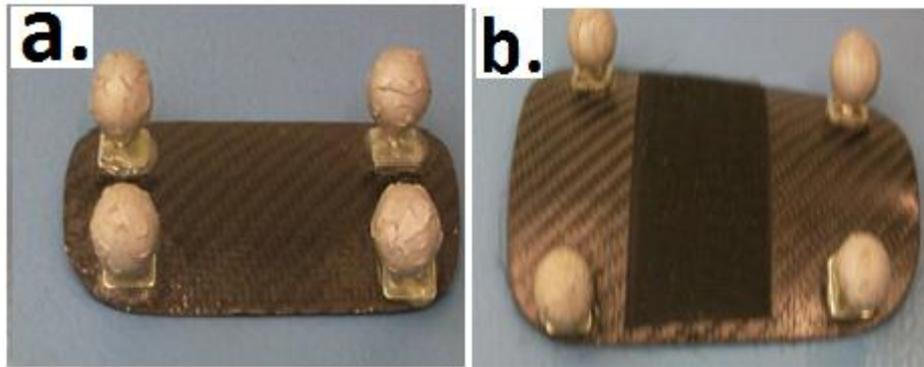
Figure 3.7: Rigid carbon fibre tracking clusters (a. = tibial cluster and b = thigh cluster).
