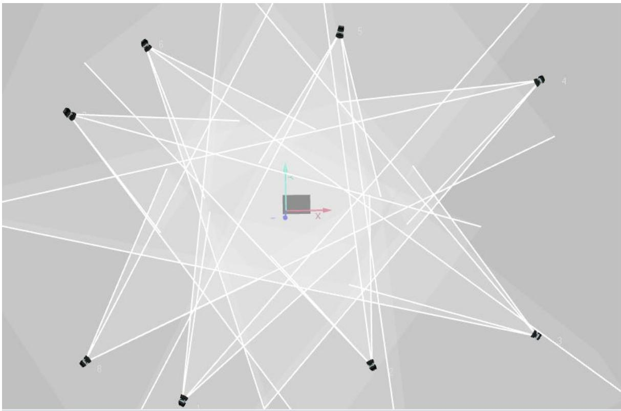
Figure 3.4 Camera positioning around the force platform using eight camera set-up.
