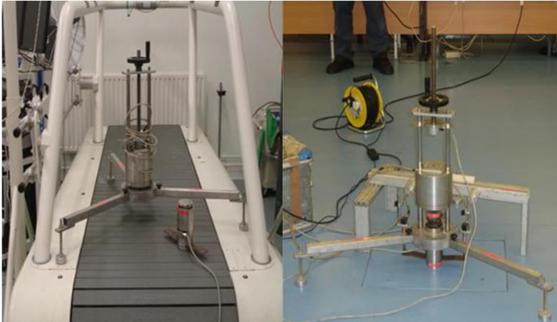
Figure 4.22: Berlin artificial athlete positioned on both treadmill and biomechanics laboratory floor.
