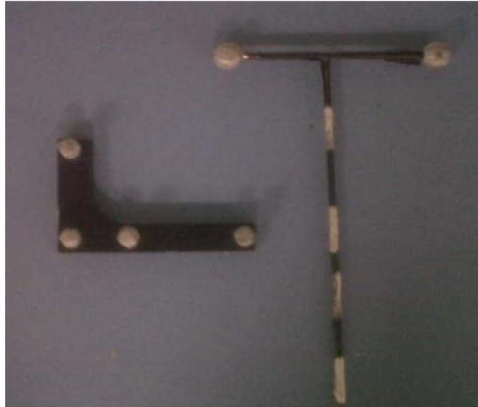
Figure 8.8: Miniature calibration wand and L-frame.
