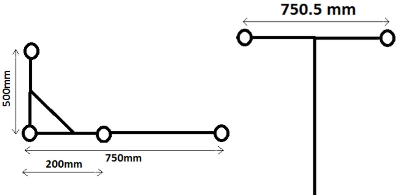
Figure 3.3 Schematics of the L-frame and wand
