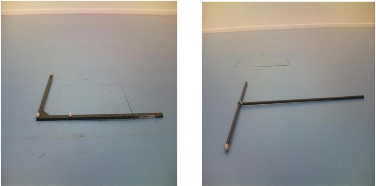
Figure 3.2: Static reference L-frame and wand used for dynamic calibration of 3-D Oqus system.
