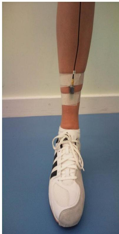
Figure 5.3: Positioning of the accelerometer on the distal antero-medial aspect of the tibia.
