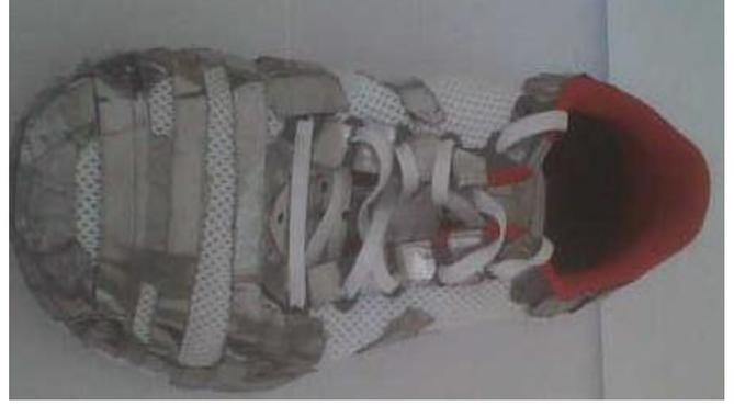
Figure 8.7: Nike Free shoes fitted with lead tape
