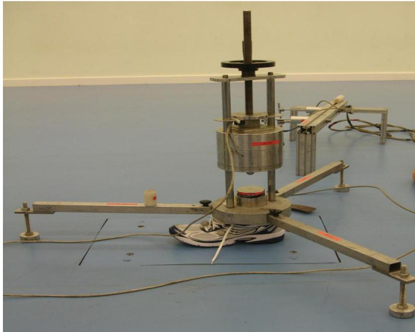
Figure 4.23: Mechanical testing of footwear shock attenuation properties using the Berlin Artificial Athlete.
