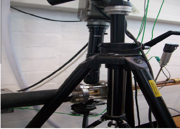
Fig. 4. Camera and sight glass set up.
