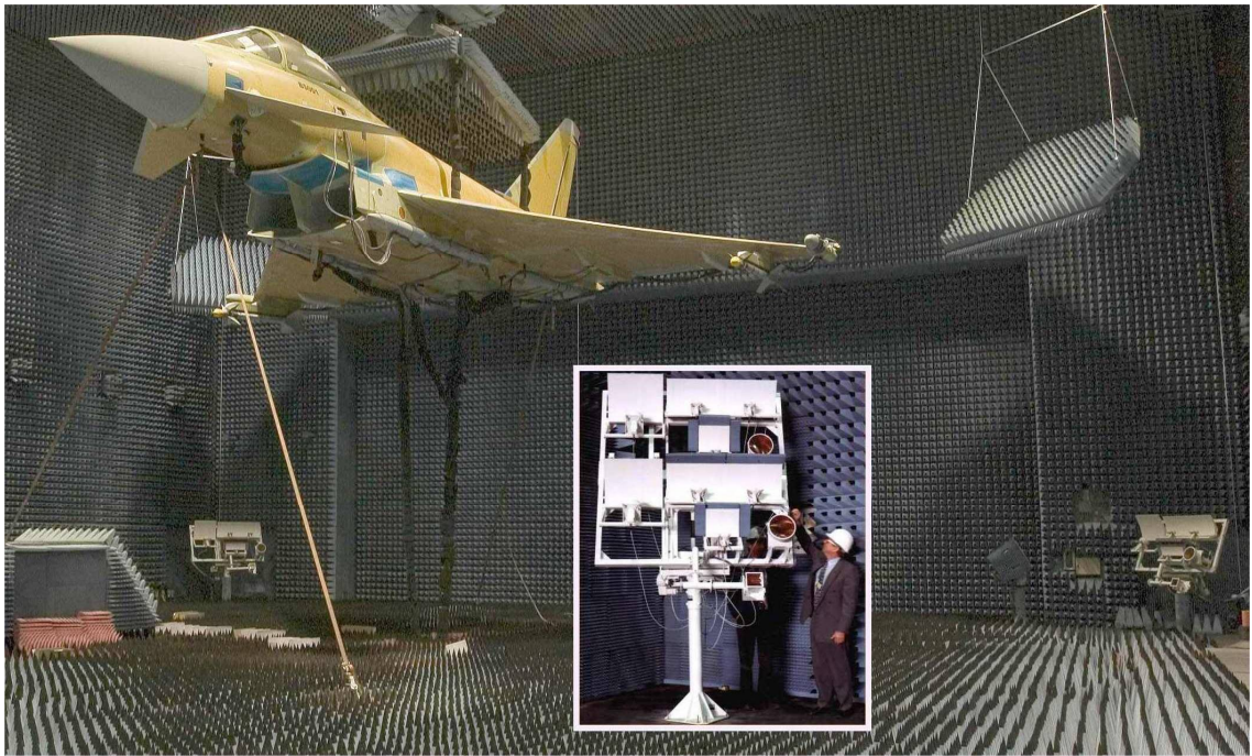
Figure 3-2: Typical ISTF: BAE SYSTEMS' EW Test Facility (UK)
