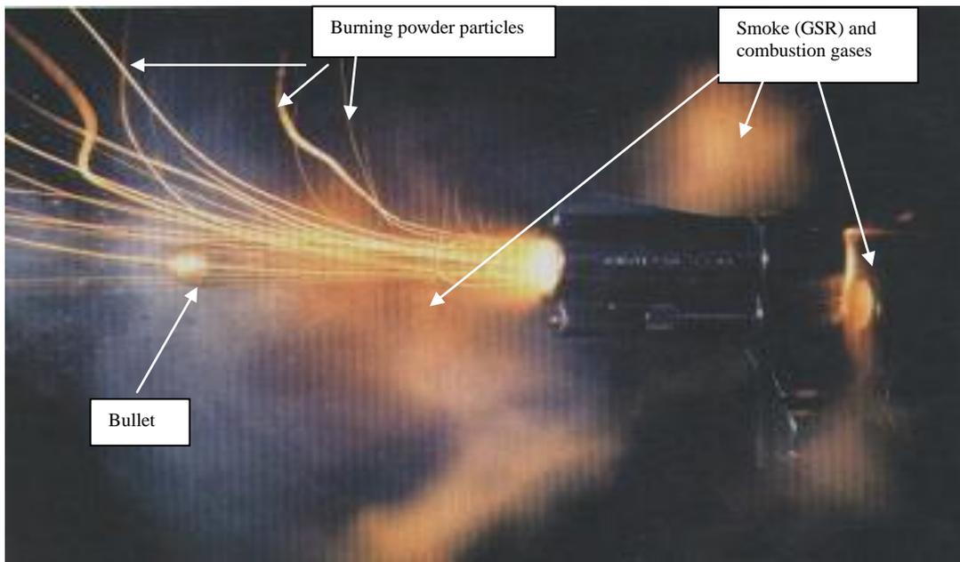
***Figure 1.3. A discharging revolver showing gunshot residue components [46]***
