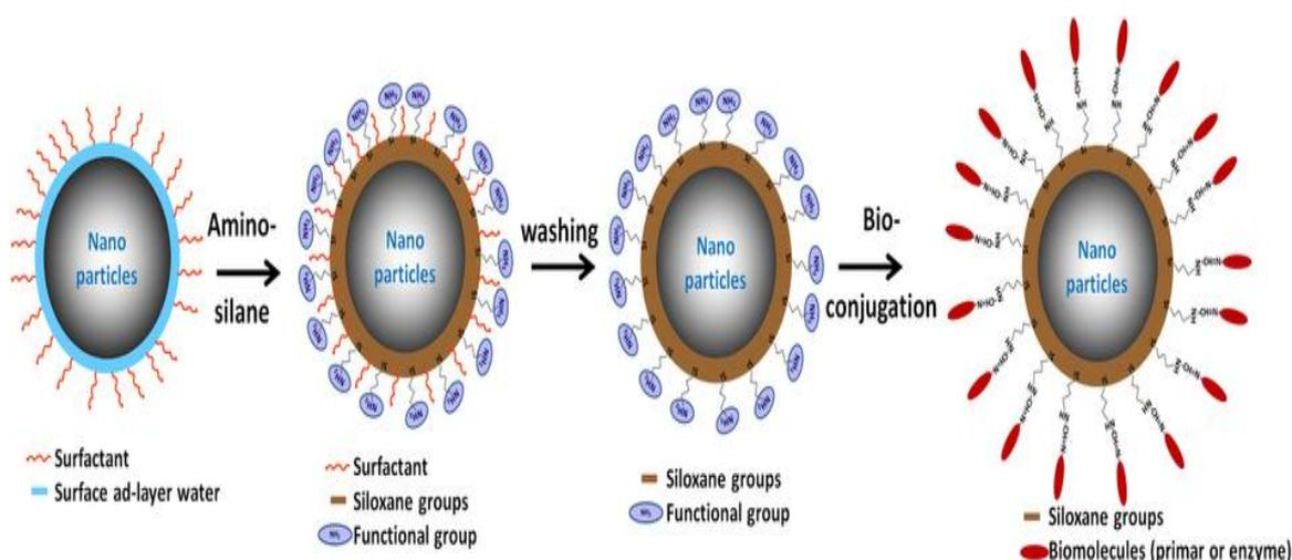
**Figure 6.2.** A schematic diagram of TPRE for surface patterning of nano-particulates in suspension [234]
