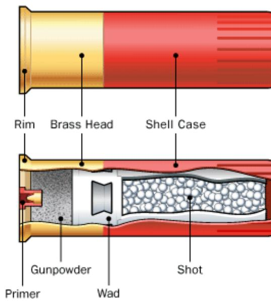
*Figure 1.2. The composition of shotgun ammunition [23]*
