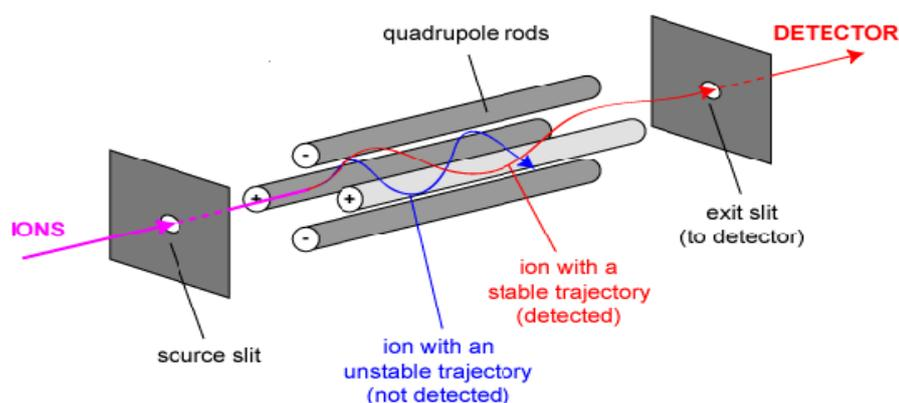
*Figure 2.2. Basic Operation of a mass spectrometer[179]*
