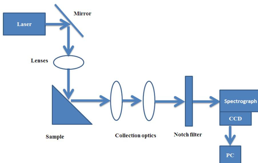
*Figure 2.7. Schematic diagram for Raman spectroscopy [202].*
