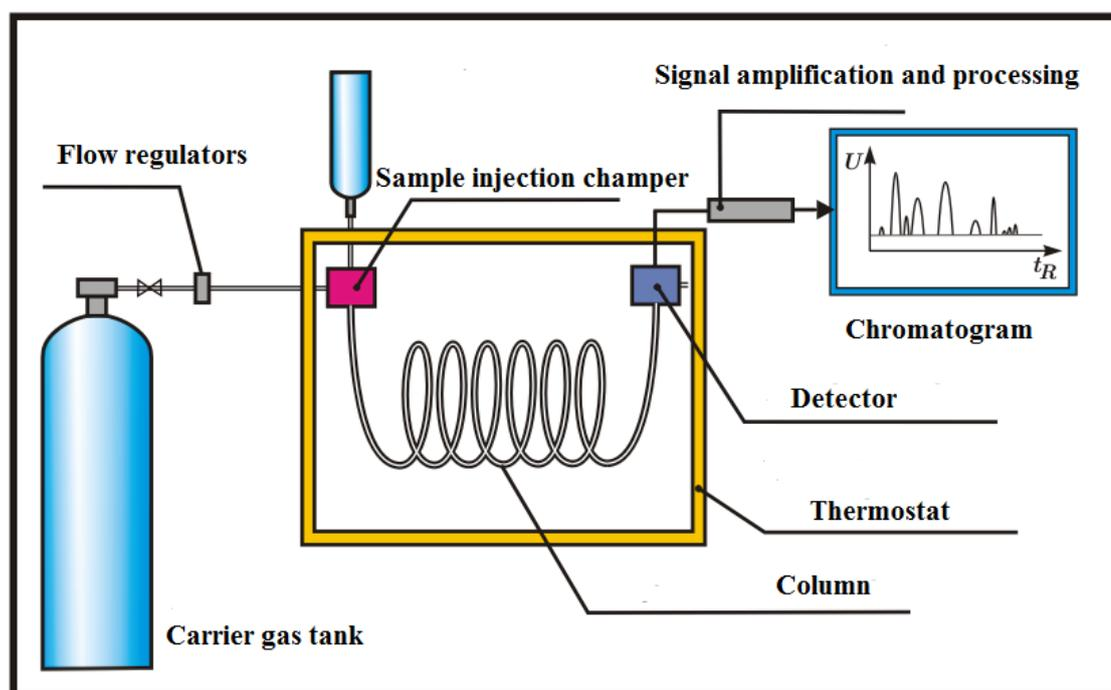
*Figure 2.1. Block diagram of a typical gas chromatography[177]*
