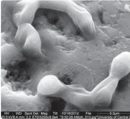
**Figure 4: Filamentous bacterial growth on the surface of sand within unplaced concrete.**
