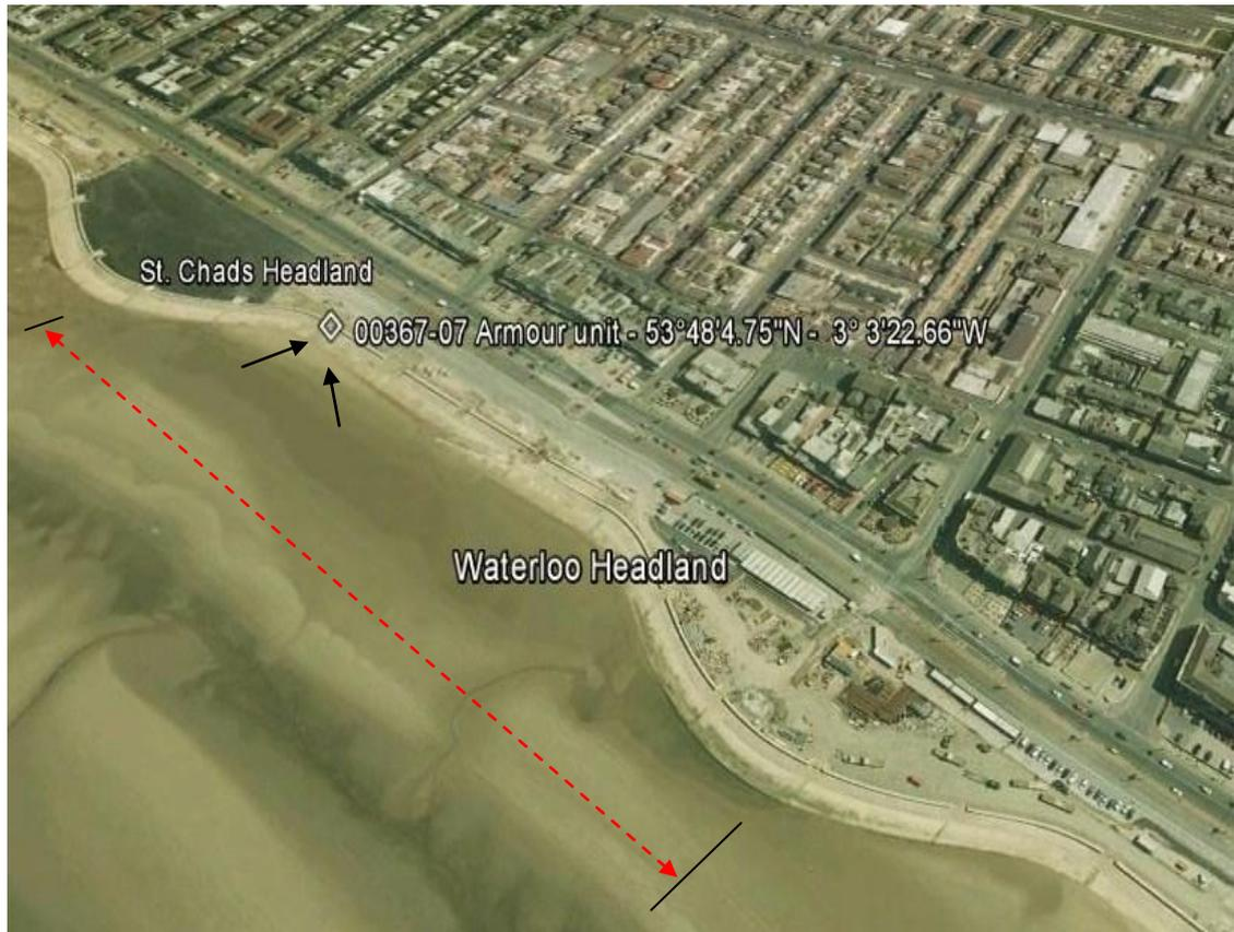
**Figure 3.6** Position (St. Chads Headland) of a monitored unit at the study site (arrowed). Hammer and UPV test on other units were also undertaken at Waterloo Headland. The red line indicates the area of the study site for this phase of work. Video of site on disc in Appendix.
