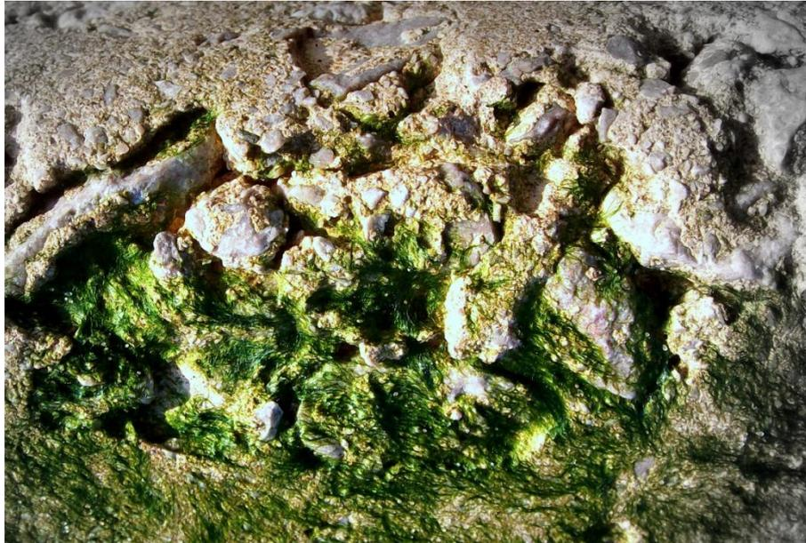
**Figure 8.9** Algal colonisation around large aggregate
