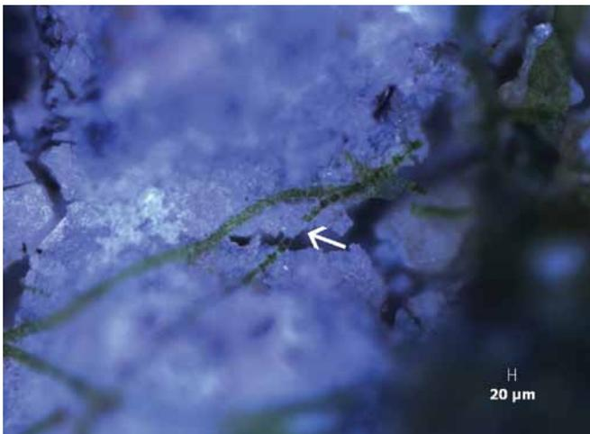
Figure 8. Algae penetrating through the coating (arrowed).
