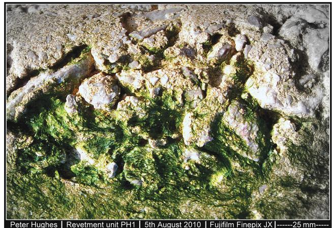
Figure 5. Digital photograph showing the nose of the step of the unit, tested in this research after 2.5 years' exposure (2010)
