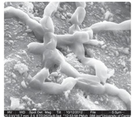
**Figure 2:** Extensive microbial surface fouling; filamentous bacterial growth can be seen on the surface of sand from within new concrete.
