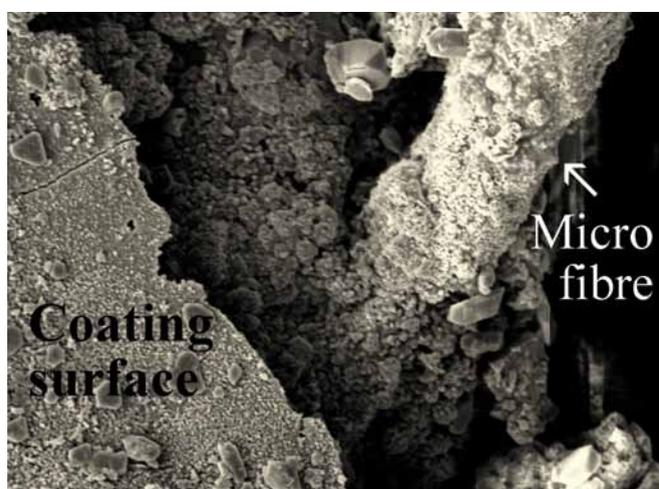
Figure 3. Fibre 'pop out' through the coating.
