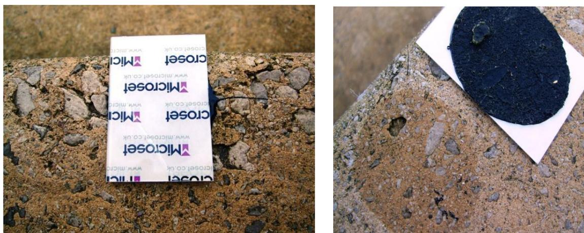
**Figure A3.3** Curing replication polymer at the study site.
