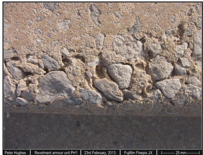
Figure 6. Digital photograph showing the nose of the step of the unit, tested in this research after 5 years' exposure (2013)
