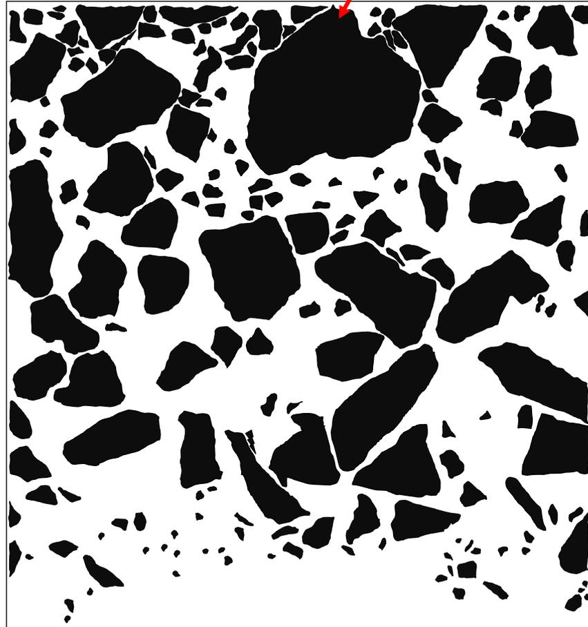
**Figure 3.15** Binary representation of inverted specimen detailed in Fig. 3.14 The tightly packed and overlapping limestone aggregate now at the exposed surface of the unit. Figure 3.16F is a typical example of aggregate tightly packed at the surface of the armour unit at the study site, particularly at the nose of the step.
