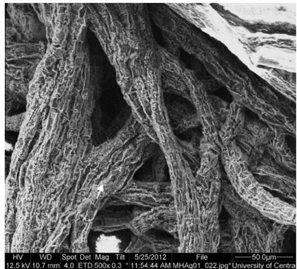
**Fig. 8.** SEM micrograph, side view of algal colonisation under a fibre specimen, after 4 years exposure.
