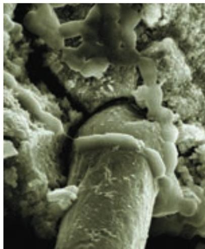
Figure 1: a micro-fibre (22µm-diameter) with bacterial bio-tenacious growth (350nm-diameter) around the cement interface
