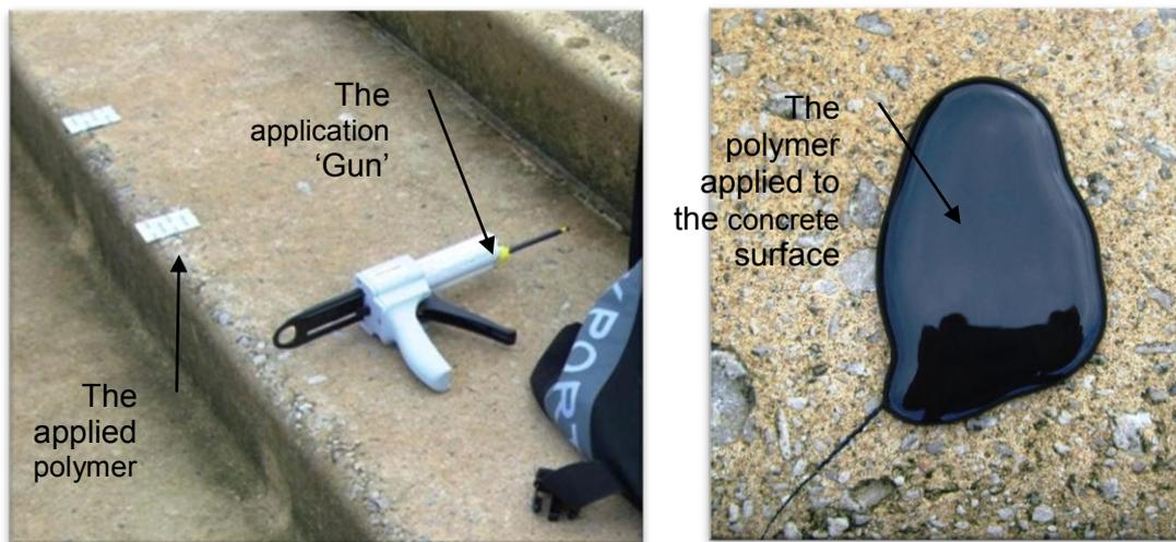
**Figure 3.8** Equipment used for the surface replication technique at the study site.
