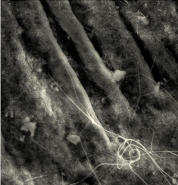
**Left - Figure 4:** SEM of a water void within the matrix. The chamber had 'rippled' effect walls, similar to tide marks on a beach. This cavity probably held water utilised by the micro-organism.
