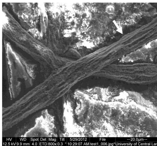
Figure 4.15 Growth cutting into fibre
