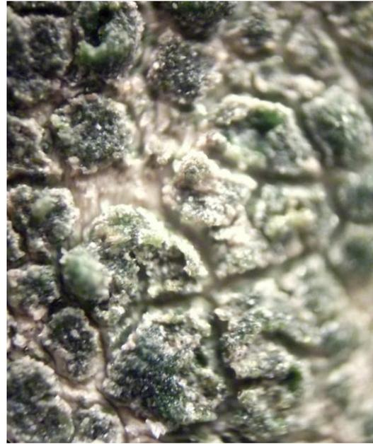
**Figure 5.12** Surface of sealant at 2 yrs exposure.
