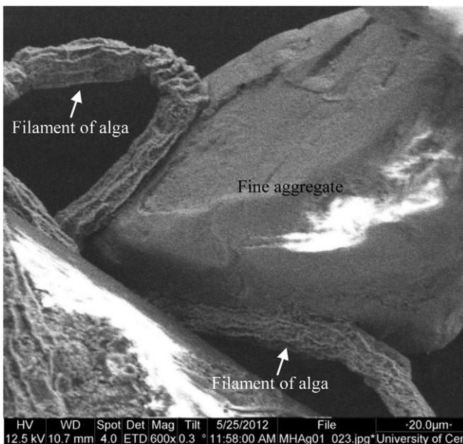
**Fig. 5.** SEM, secondary electron micrograph, side view of revetment armour concrete surface, after 3 years exposure. This sample was not sputter coated, showing the algae filament in its natural condition. The filament can be clearly observed growing freely around the almost fully exposed fine aggregate.
