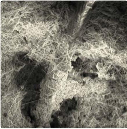
Figure 2 above: A micro-fibre protruding from the surface of concrete. Note the bacterial colonisation within the void beneath the surface.
