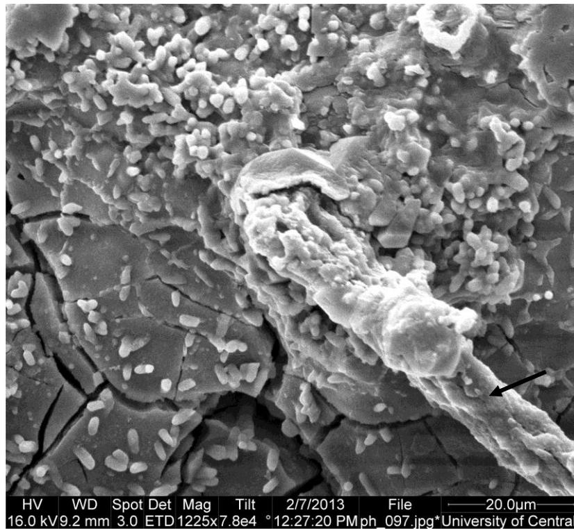
**Figure 6.18** Coating of revetment tile after 2 months exposure at site 3. Algal filament (arrowed) is shown attached to the surface of the coating.
