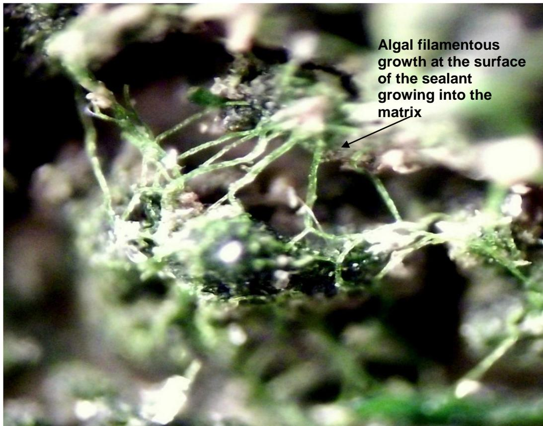
**Figure 5.13** Algal colonisation on the surface of the sealant after 2 years exposure.
