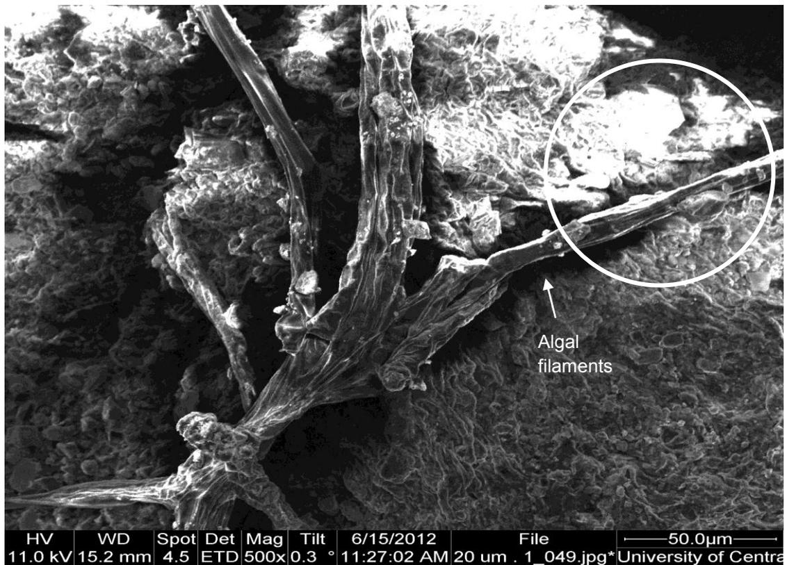
**Figure 4.9** Network of algal filamentous growth intertwine over the limestone aggregate within the matrix to a depth of approximately 25 mm. Filaments appear to cut into the surface of the aggregate surface (circled).
