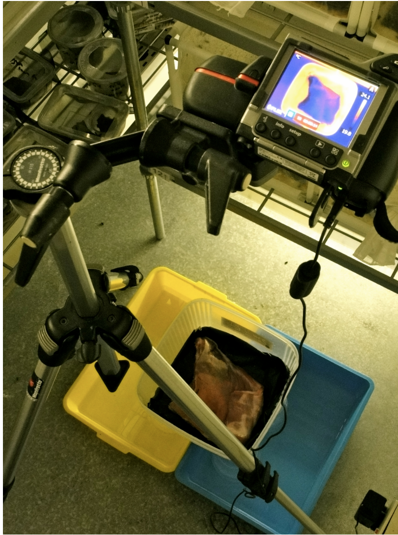
Figure 5.1. Experimental setup for data collection with the FLIR T425 thermal imaging camera positioned directly above the maggot mass and set to record temperatures every five minutes
