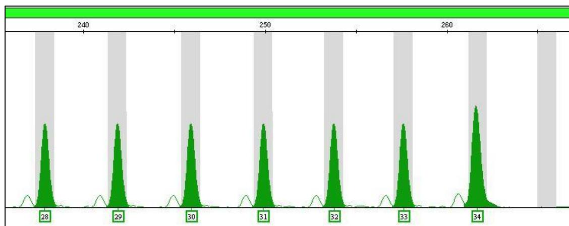
**Figure 4.1:** In-house developed DYS626 locus allelic ladder comprising alleles 28 to 34. The alleles had 28 to 34 repeats and were called in accordance with ISFG recommendations in this regard (Ballantyne et al., 2010).
