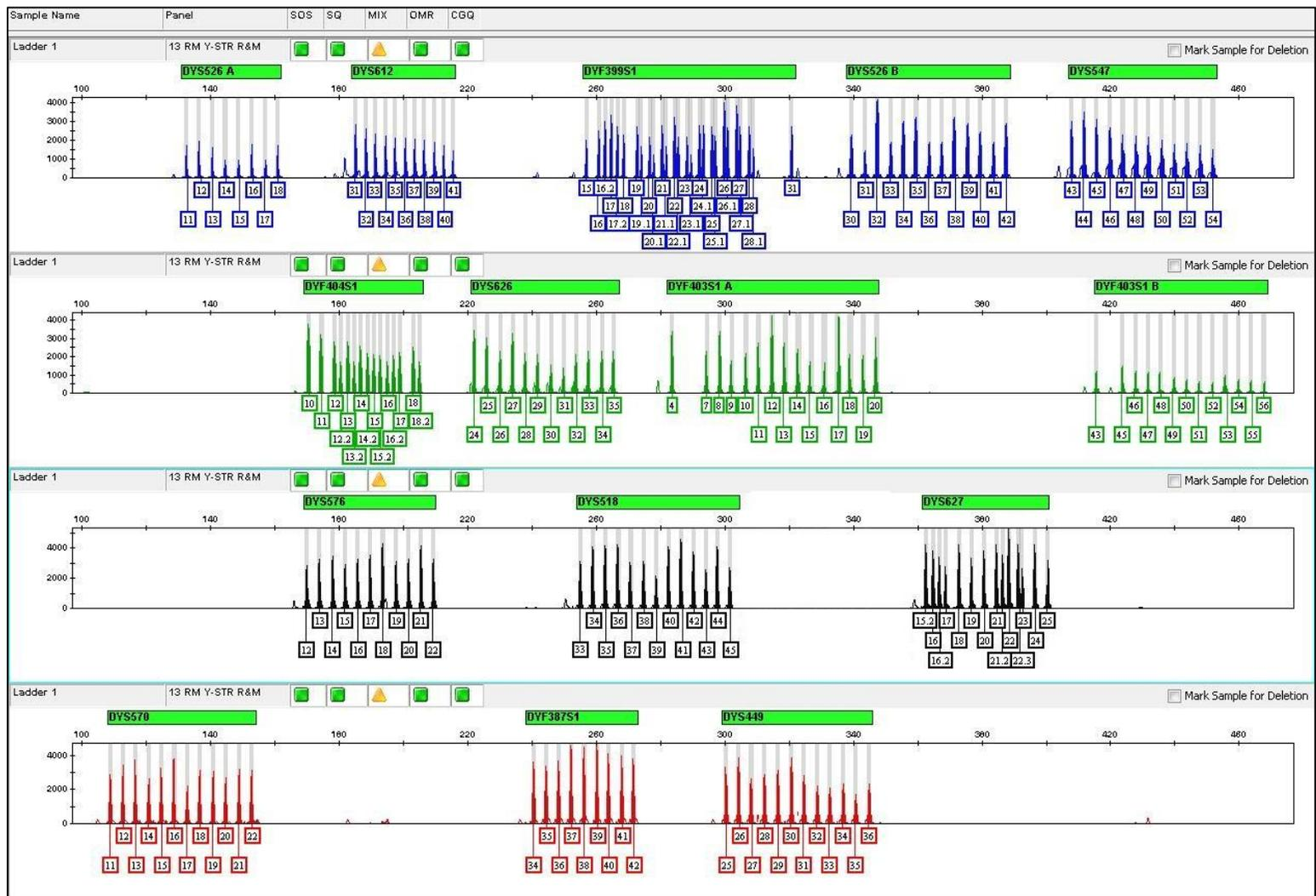
**Figure 4.4:** Electropherogram as a results of analysing 1 µl of the developed allelic ladder for RM-Yplex multiplex assay
