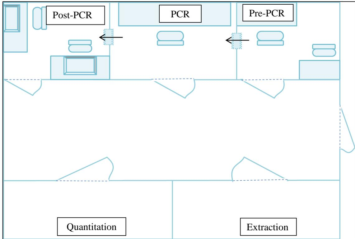
**Figure 2.4:** Illustration of DNA profiling Laboratory design in the Department of Forensic Sciences and Criminology (DFSC) Dubai Police.
