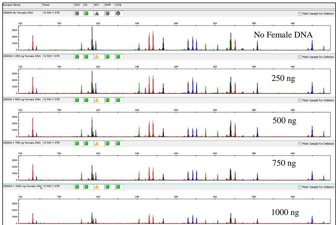
**Figure 5.3:** RM Y STR profiles generated from amplification of various ratios of male:female mixtures. The male sample used was the male control DNA 2800. All panels are in scale. Amount of female DNA is typed in each panel.
