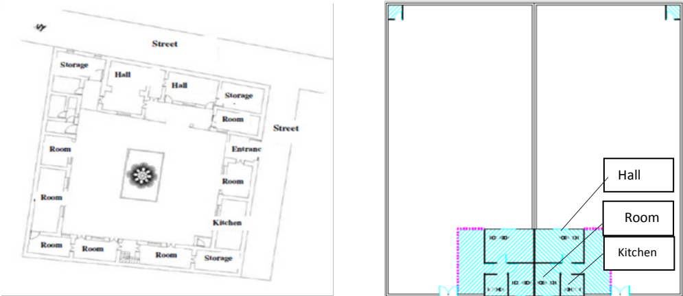
Fig.2 Spatial planning of a pre-earthquake (Left) compared with the post-earthquake (Right) housing units in Lar.
