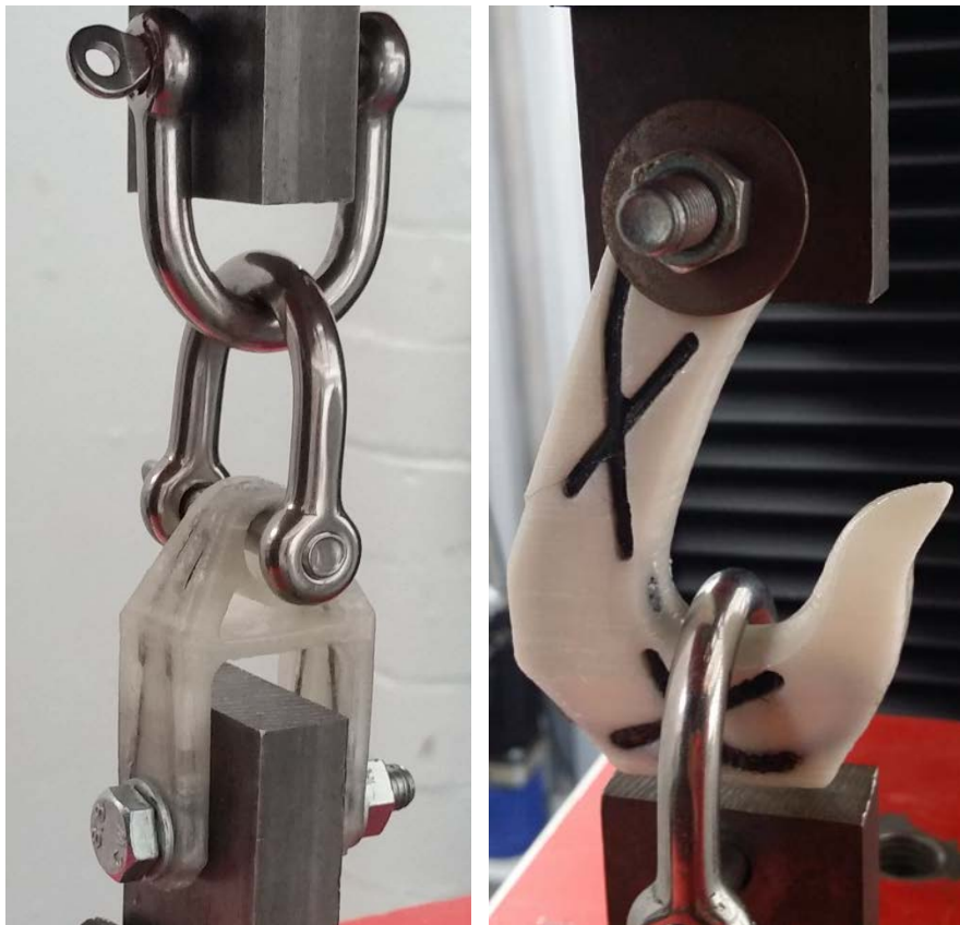
Figure 8. Fixtures for pulley and hook tests.
