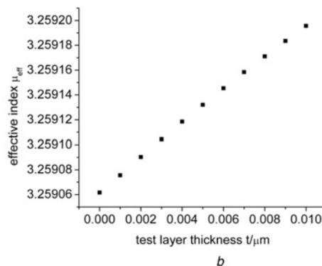
**Fig. 8** Effective index against test layer index
