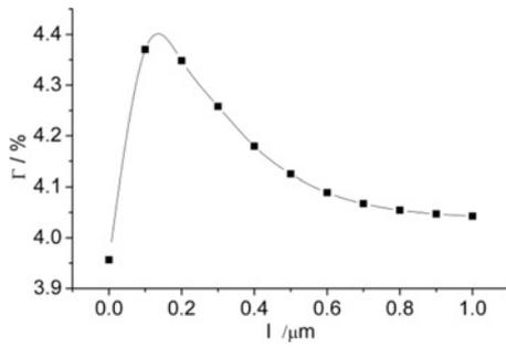
**Fig. 7** Confinement factor as a function of cladding layer thickness for three-layer waveguide with  $\Delta\mu = 0.23$
