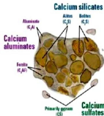
*Figure 3.1 composition of cement clinker [98]*
