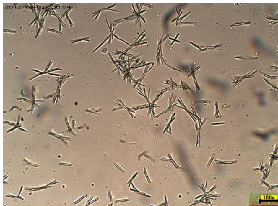
Figure 3.12 A photograph showing BDP crystals deposited in the bottom of centrifuge tube after 90min centrifugation observed under 40X magnification. This is typical of 3 such different experiments.
