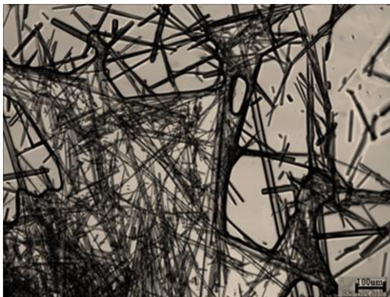
Figure 4.9 Light microscopy image showing the formation of mannitol crystals on hydration of mannitol based proliposomes. Magnification used is 400x. This is a typical of three images
