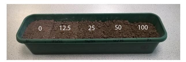
Figure 1. Linear gradient mescocosm (0.6 m x 0.13 m x 0.1 m) with nominal Ag NP / AgNO<sub>3</sub> concentrations (mg kg<sup>-1</sup>) used in the Experiment 2 avoidance test. Each treatment occupied an equal soil volume (0.12 m x 0.13 m x 0.085 m).
