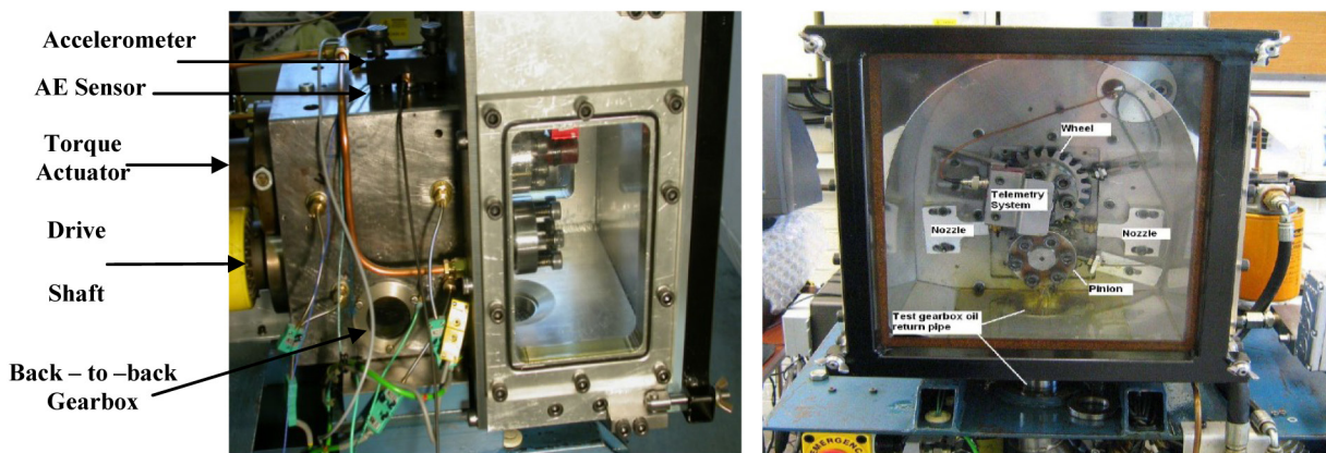
Figure 1. Newcastle University 75 mm centre distance back-to-back gear test rig
