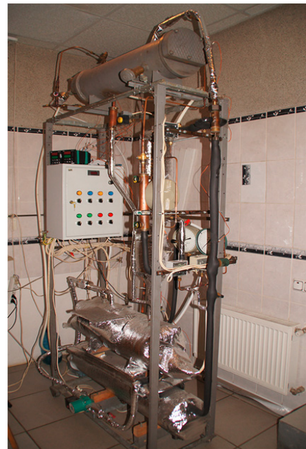
Fig. 1. ERS experimental unit. P_{gen} , P_{cond} , P_{eva} – generation, condensation, evaporation pressures; FM1,FM2,FM3 – water flow meters; SV1,SV2 – solenoid valves; CV1,CV2 – check valves; T1-T12 – thermocouple.
