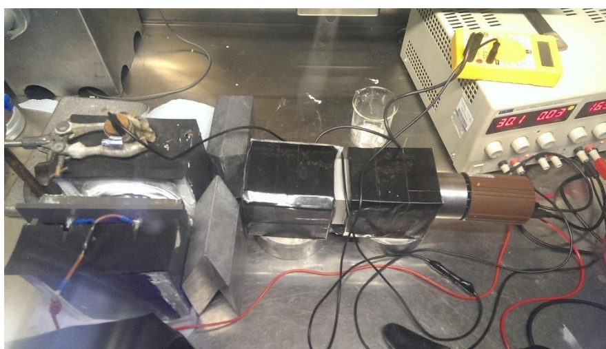
Figure 2. Photograph of the in situ CsI(Tl) detector setup used to monitor the decontamination of ^{137}\text{Cs} , where the detector is surrounded with a lead collimator sheath with the circular aperture cut into the centre.
