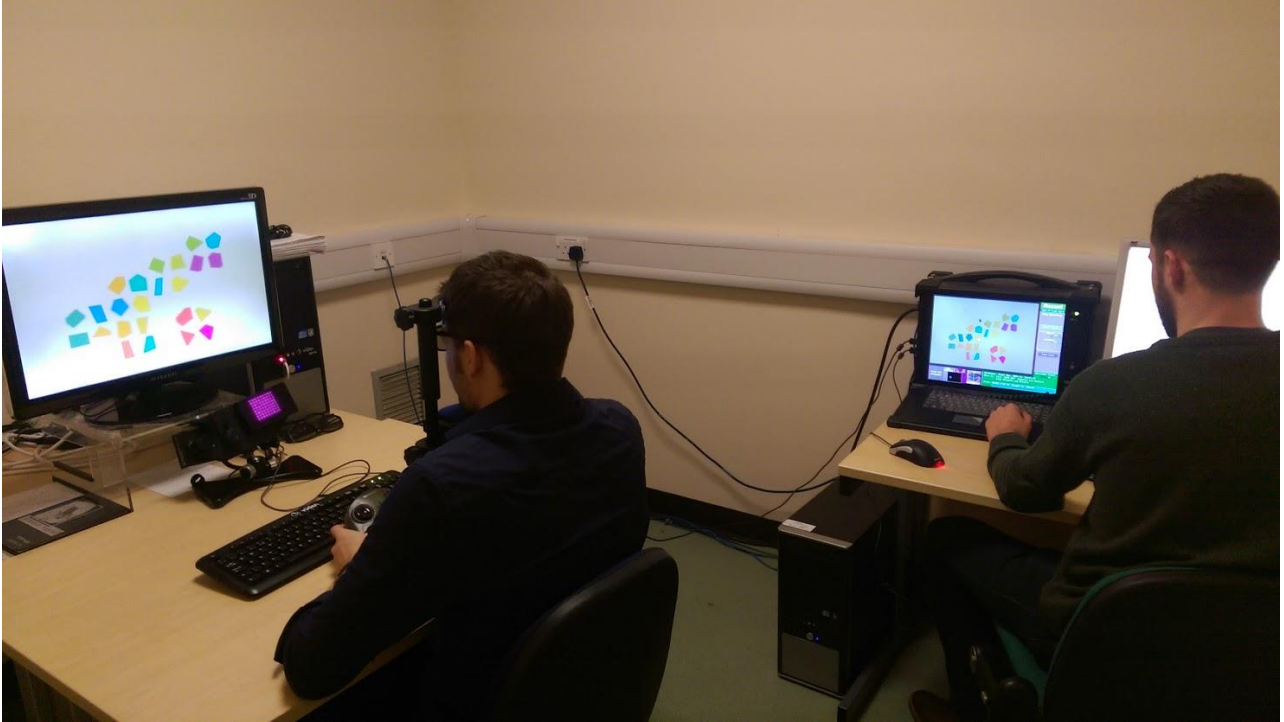
Figure 3. Lab setup example. Participant is seated in front of the stereoscopic display (left side) while the experimenter controls the running of the experiment from a separate computer (right side). During actual data collection, the lights are dimmed in the room.
