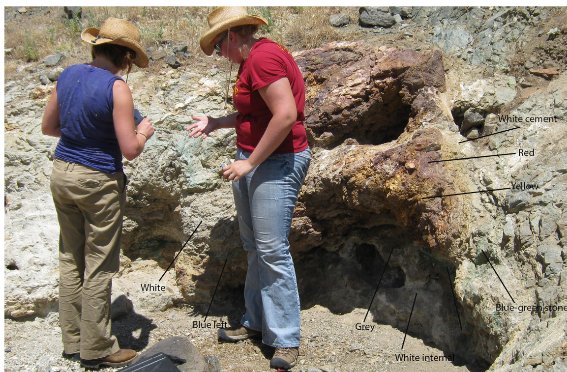
Figure 9. Overview of quarry site showing areas from which assays were taken (see supplementary material 1 for full data).
