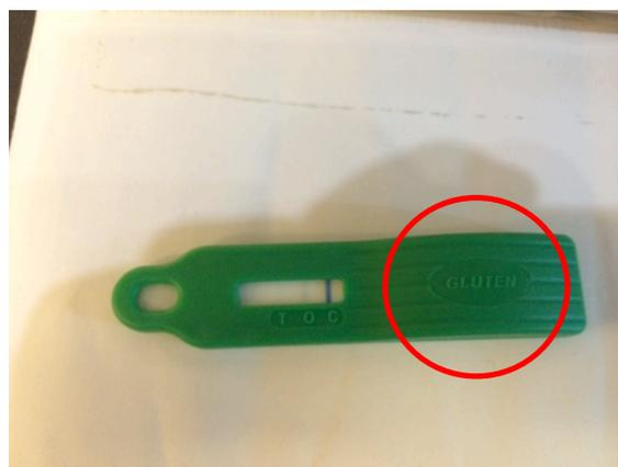
Test 3 in detail shows only two lines and no line can be seen on the T. Level of gluten is below the detection level which is at 1.0 ppm. Please note *GLUTEN* embossed on the devise.
