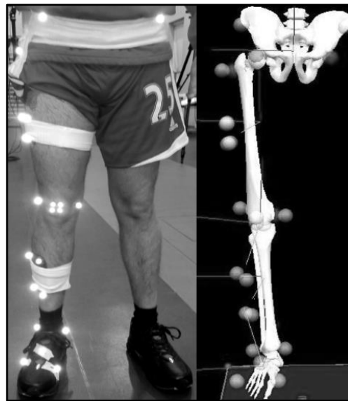
Figure 7: CAST Marker setup & corresponding image on Qualysis.
