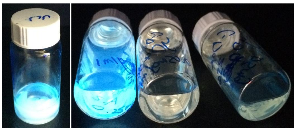
Fig. 3.4. Images of the fluorescence characteristics of 32.5% w/t P-123 hydrogel samples with aC-dots, and dilute solutions of aC-dots, JD-230 C-dots and JD-400 C-dots respectively from left to right. The hydrogel was made at a concentration of 0.103 mg/ml and each dilute solution was maintained at 0.05 mg/ml.
