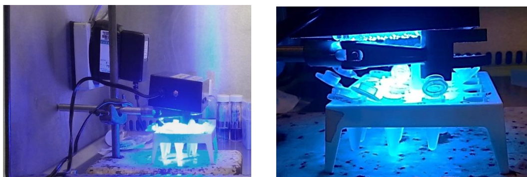
Figure 113 Set-up of UV illumination on to bacterial cells and biocide
