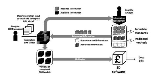
**Figure 1**: The dilemma of information within the BIM process, and how many information requirements by the quantity surveyors cannot be integrated within the BIM Model.
