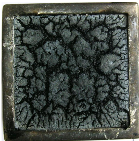
Figure 98: Residue from cone calorimeter test of samples containing ATH, magnesium hydroxide, and chalk
