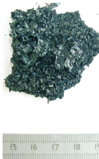
Figure 99: Internal structure of the residue of samples containing ATH and magnesium hydroxide
