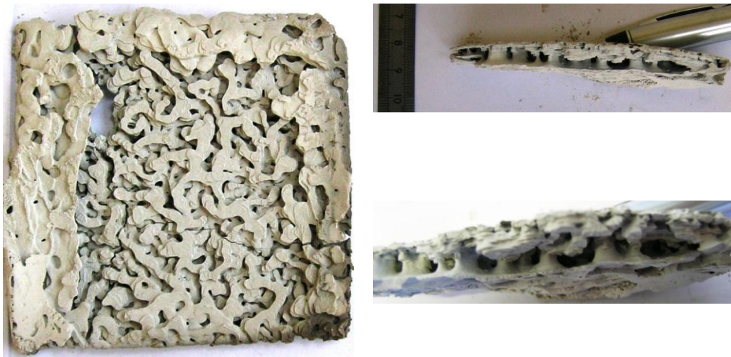
Figure 100: Internal structure of the residue from samples containing chalk
