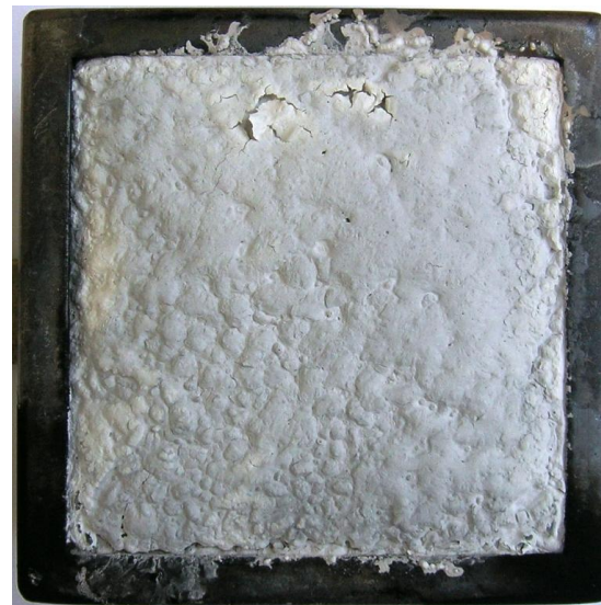
Figure 98: Residue from cone calorimeter test of samples containing ATH, magnesium hydroxide, and chalk
