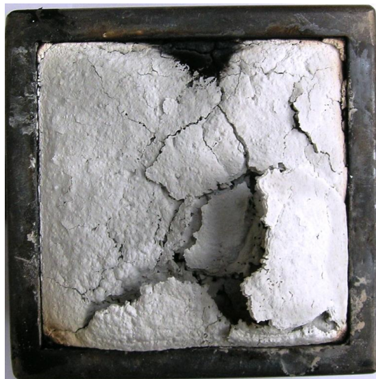
EVA.ATH (residue that collapsed during test)
