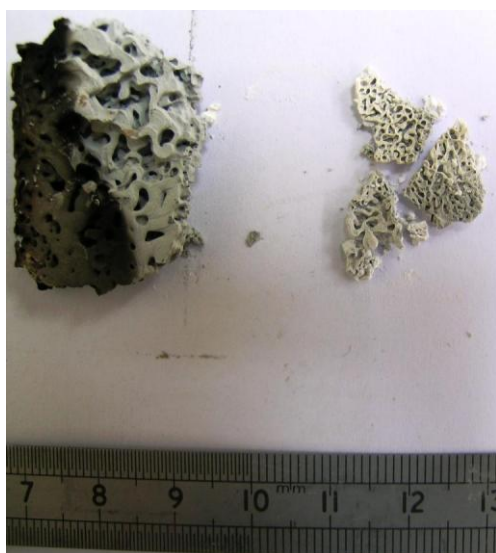
Figure 99: Internal structure of the residue of samples containing ATH and magnesium hydroxide
